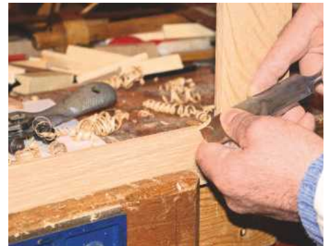
▲ Pic.15 A chamfer runs on the inside edges of back panels and outside edges of glazed panels...
