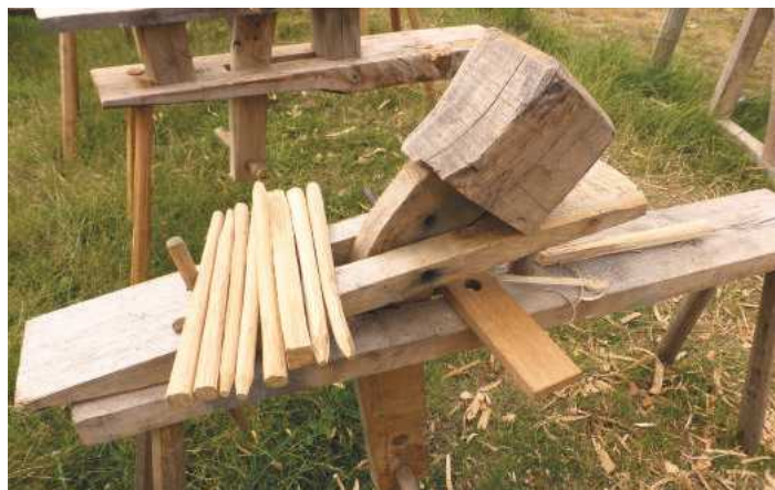
Pic.12 The shaving horse used to prepare dozens of hand-made pegs
