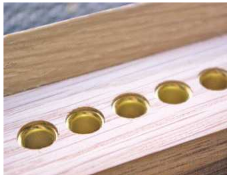
▲ Pic.23 With a suitable mandrill drive the sleeves in until the flange is below the surface
