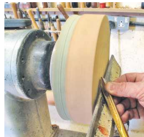
▲ Pic.3 He is using a 10mm bowl gouge in a pull-cutting technique to do the initial truing of the base. A push cut could cut directly into the end grain, resulting in an uneven surface
