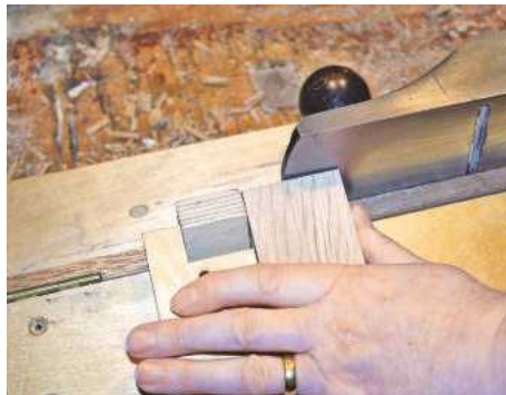
▲ Pic.11 Having marked out materials for the main frames, trim to accurate 90° on shooting board...
