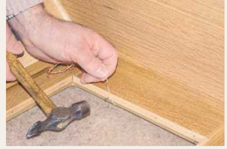
▲ Pic.3 Pin the strips to the frame – Bernard uses telephone wire to save his fingers!
