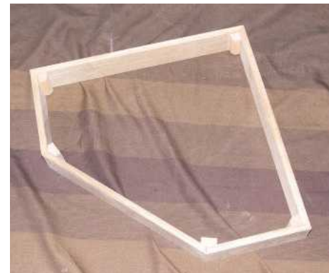
▲ Pic.3 Assemble the pieces for a dry run, enabling you to check angles and make changes
