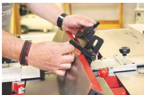
▲ A cast-iron fence is a great feature and it adjusts easily
