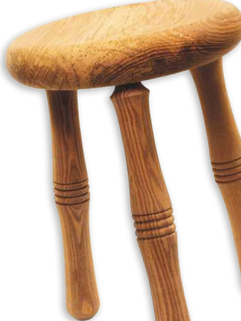
▲ Pic.35 The button and legs are glued in with a good-quality PVA. Traditionally the legs would go through the seat and be wedged, but modern glue makes this unnecessary
