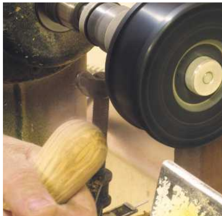
▲ Pic.32 Once the waste on the ends of the legs is cut off they must be sanded. His Sand-o-Flex rotary sander is the best tool for this as it doesn't over sand the end grain
