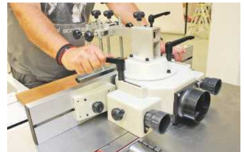
▲ The spindle hood is solidly made and secures with Bristol levers
