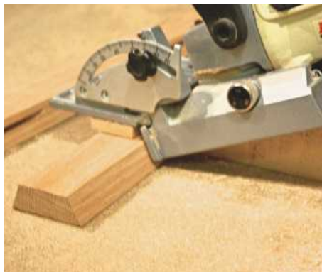
▲ Pic.2 Cut biscuit slots on the inside edge of the board which form right angles
