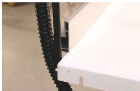
▲ The bracket for the crown guard hose allows the work to pass under without snagging
