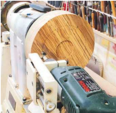
▲ Pic.10 His drill wizard is set up with a 22mm saw tooth and the lathe locked in the 1, 17 and 33 positions as it has 48-point indexing; on 24 point it would be 1, 9 and 17
