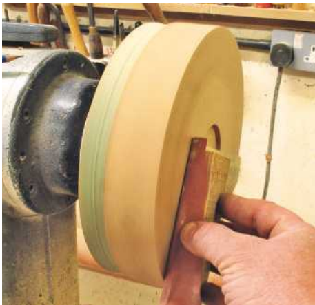
▲ Pic.13 To maintain the flatness of the bottom and avoid sanding out the softer grain to leave ripples, sand the base with sandpaper wrapped around a block of wood
