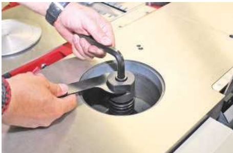
▲ A spanner and hex key are used to swap blocks
