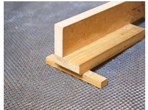
▲ Pic.12 ...or a jig to mount the pieces vertically in a bench vice
