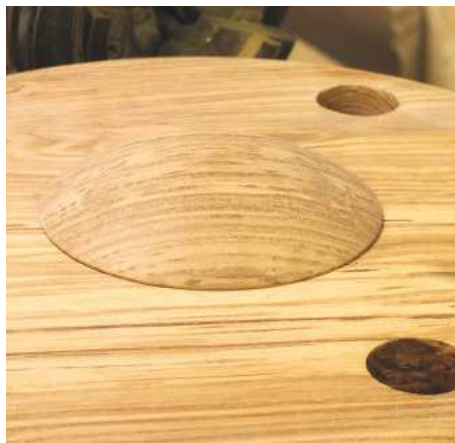
▲ Pic.35 The button and legs are glued in with a good-quality PVA. Traditionally the legs would go through the seat and be wedged, but modern glue makes this unnecessary
