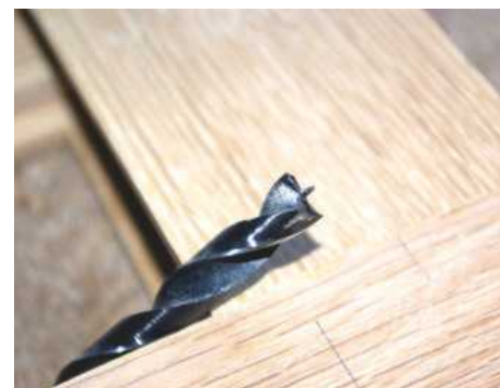
▲ Pic.19 A drill with a reduced tip was used to make holes for the shelf supports
