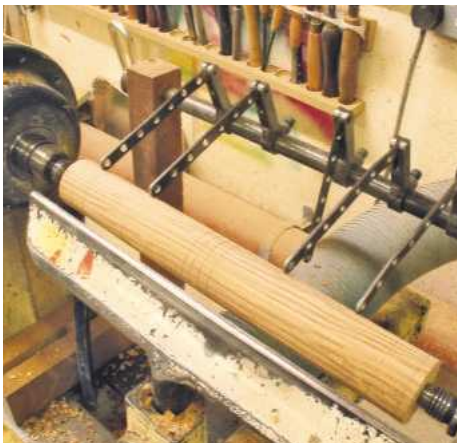
▲ Pic.31 He uses copying fingers to measure the next two legs, removing the wood until the fingers fall through; this is much better than using callipers
