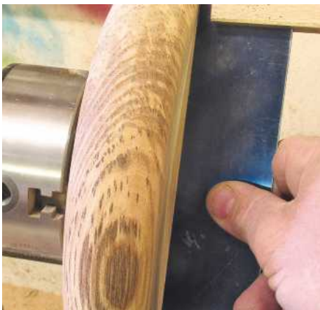
▲ Pic.16 You can see the light under the straight edge. You can also see how pretty the figure is on this ash, the colours almost making it look like a piece of brown oak
