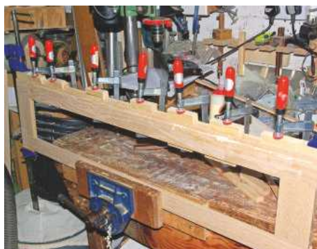
▲ Pic.18 Lots of clamps will be needed while gluing up the main frames
