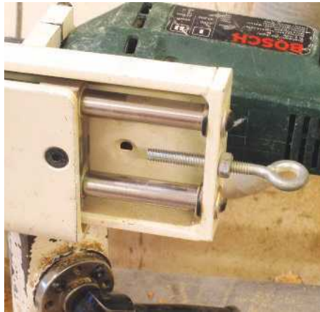
▲ Pic.11 The depth stop on his jig is set to drill 25mm deep; a piece of tape on the drill would do the same job. Doing this accurately will keep the legs the same length
