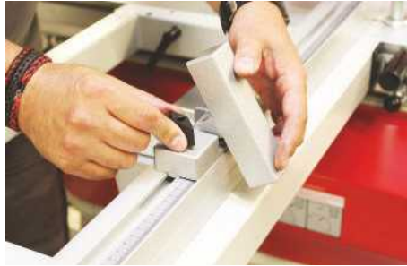
▲ A big hold-down clamp keeps things secured and can be used in conjunction with the flip stop
