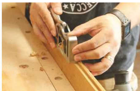
▲ Using the plane in a conventional manner on long-grain work is comfortable
