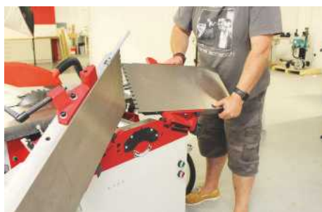
▲ The planer tables have to tilt away for thickness work
