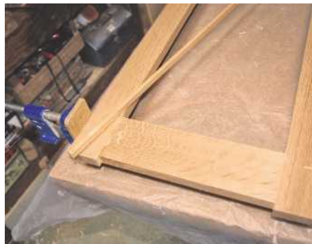
▲ Pic.14 Check the assembly prior to gluing up. After cramping check for squareness
