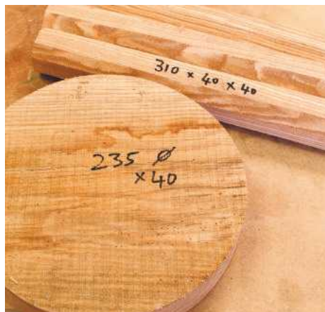
▲ Pic.1 The sizes to which the wood is cut are only a rough guide and are worked out from pictures. This ash has some stunning grain and has a moisture content of around 16%
