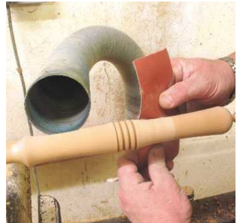
▲ Pic.30 To see the shape more clearly and not sand away the detailing Les likes to sand the wood behind like this. Be careful not to sand the spigot
