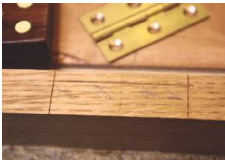
▲ Pic.34 The hinges were marked out on the edge of the door frame
