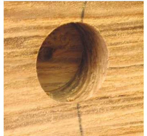
▲ Pic.12 Even though the hole is drilled at an angle it's really clean. The hole is drilled at an angle so the legs splay out, giving the stool stability on its three legs
