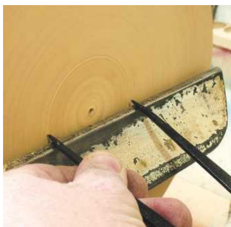
▲ Pic.5 Set the toolrest on the centre height and scribe a circle with only the left-hand point; if this lines up with the right you are correct. Do not let the right-hand point touch the wood
