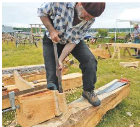
Pic.8 Why use a chisel to pare the cheeks of a tenon when you can use a bisaigue? Andy is using this French version of the thrust axe or twybil, with a mortise chisel at one end and a bevel chisel at the other, using his shoulder to help guide the heavy tool
