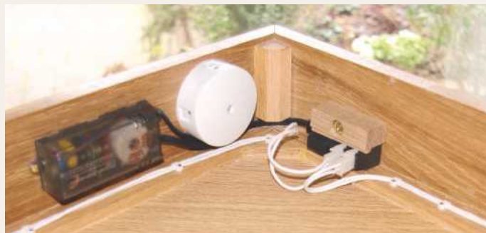
► Pic.1 A small lighting junction box, the 12V transformer and distribution block were all mounted securely under the plinth
