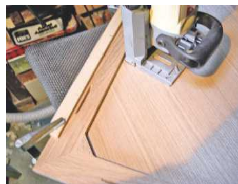
▲ Pic.27 Cut the biscuit slots into the base panel and plinth, making sure to match up the positions
