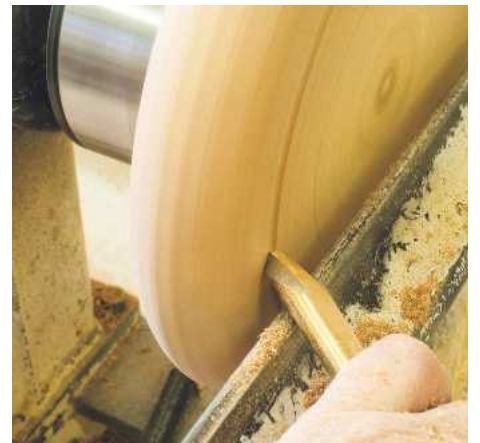
▲ Pic.15 For definition hollow the top slightly using the same gouge with the long grind in a push cut; slow the feed of the tool as you get towards the slower wood in the centre
