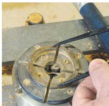
▲ Pic.4 The chuck recess on the bottom will be hidden by turning an insert and gluing it in. He is measuring the perfect dovetail jaws on his Axminster Evolution chuck with dividers
