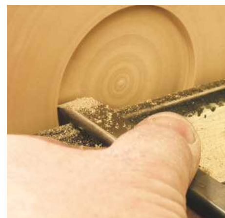
▲ Pic.6 After taking the majority of the timber with the gouge use the skew as a scraper and cut the dovetail; this will be covered later so a good finish is not necessary
