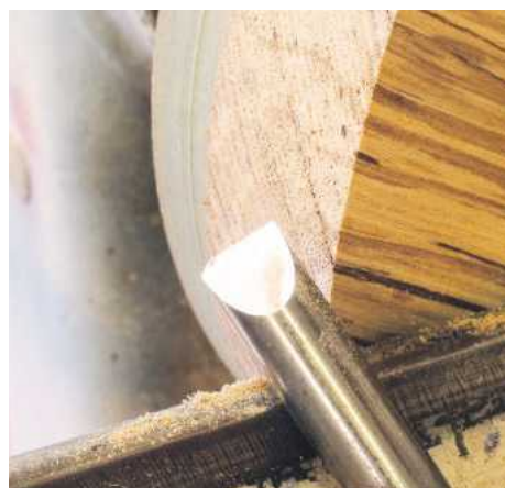
▲ Pic.7 To turn large flat surfaces on the lathe Les uses a 13mm round skew with the corner just taken off. The removal of the corner means that it cannot create lines on the surface
