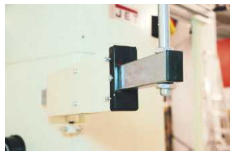
▲ This arm slides in and out as the carriage travels during a cut
