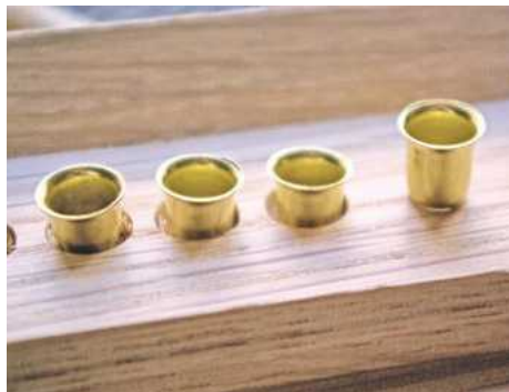
▲ Pic.22 Push the sleeves into the holes with your thumb and they will sit proud by about 5mm
