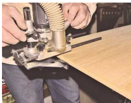
▲ Pic.26 Finally, cut a rebate 8 x 5mm deep 'round the back face to accommodate the beading
