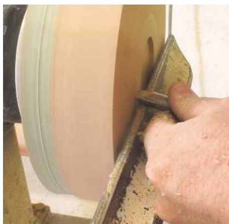
▲ Pic.8 His knuckles are running along the toolrest; this keeps the tool cutting at a consistent depth all the way along and will create a flat surface
