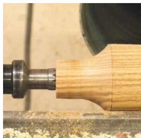
▲ Pic.24 You can see how the cove flows perfectly into the spigot; the larger-diameter curve will hide the joint where the spigot goes into the base
