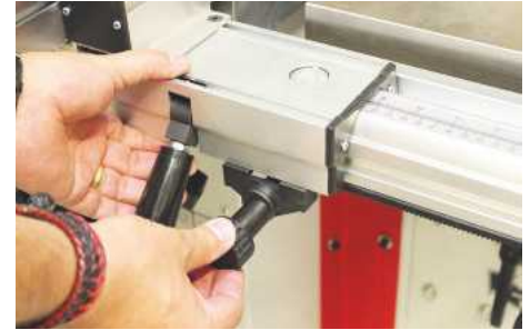
▲ The fence has a solid cam lock along with a fine adjuster
