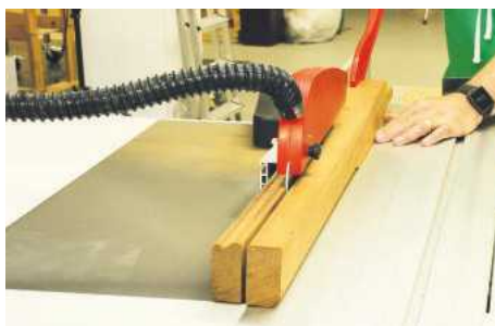
▲ Ripping 70mm-deep iroko was effortless at a steady feed speed
