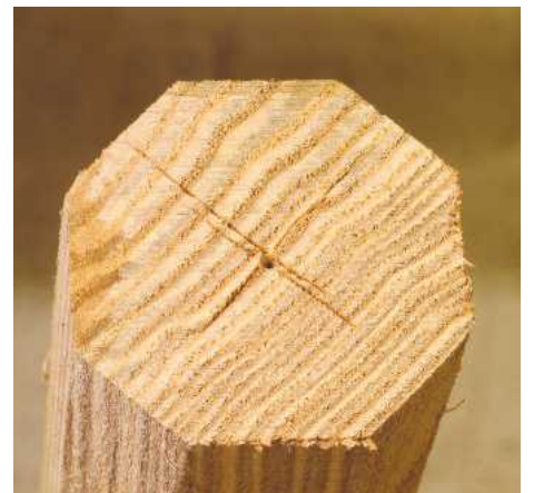
▲ Pic.18 Marking the centre with a bradawl helps to locate it onto the drive and the live centre. The end grain of the timber is just as stunning as the side grain
