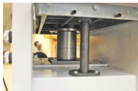
▲ The central ram is a feature normally found on more expensive models
