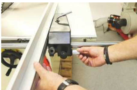
▲ The cast shoe houses a cam lever to lock it to the running rail and an adjustment knob
