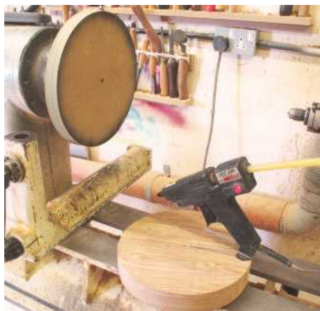
▲ Pic.2 Because Les doesn't want deep holes in the surface he is gluing the blank onto an MDF faceplate using hot glue rather than using a faceplate
