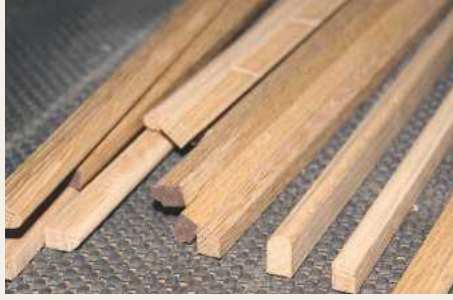
▲ Pic.2 With a fine saw separate this into two strips each about 13 to 14mm wide
