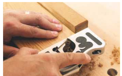
▲ The plane excels at end-grain work; fine controlled cuts are easy
