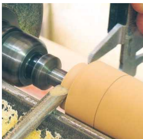
▲ Pic.22 The most important measurement is the spigot that fits into the stool top. Vernier callipers are more accurate than the bow-leg type
