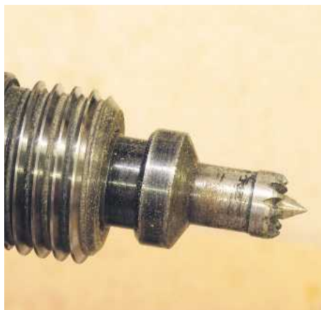
▲ Pic.19 This is the small steb centre available from Robert Sorby. They are not cheap but the spring-loaded point and the multi-tooth design make them the most effective of drives
