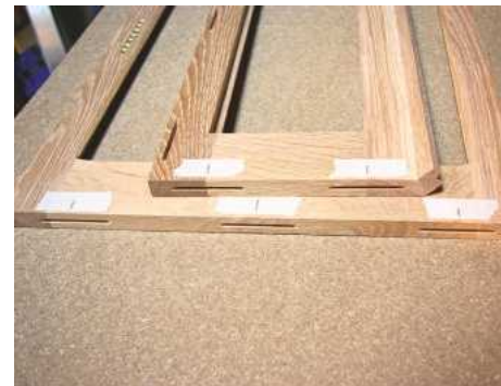
▲ Pic.17 Cut biscuit slots in the top and bottom of the frames for later attachment
