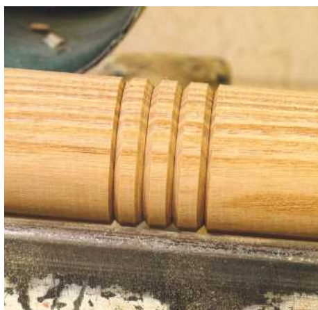
▲ Pic.25 The area of the three beads is marked up and a series of V cuts is made with the skew. They are now ready to turn into beads or you may think they look fine just as they are
