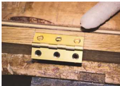
▲ Pic.37 The hinges were first screwed in with steel screws to check for fit, followed by brass ones
