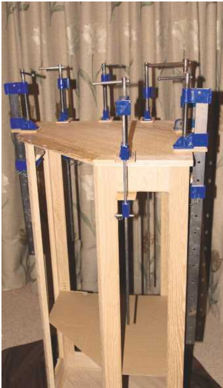
▲ Pic.31 He followed the same process for assembling the top panel to the frames
