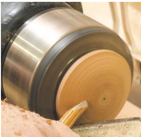
▲ Pic.34 Once a chucking point is turned on the piece it can be held while the top is rounded over. Les decided that a large button shape would look the best
