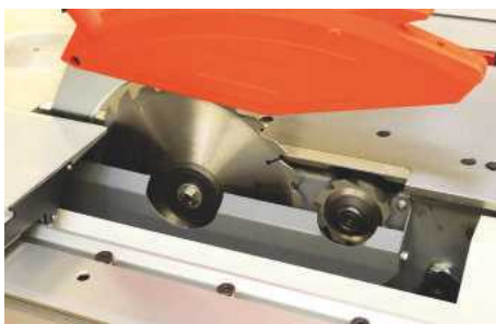
▲ Sliding the carriage back gives excellent access to both blades
