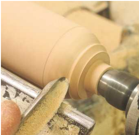
▲ Pic.28 Shaping the bottom of the leg is done with the Signature spindle gouge. Roll the tool over to the right keeping the bevel in contact with the wood
