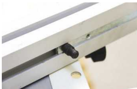
▲ A locating pin acts as a pivot for the crosscut fence
