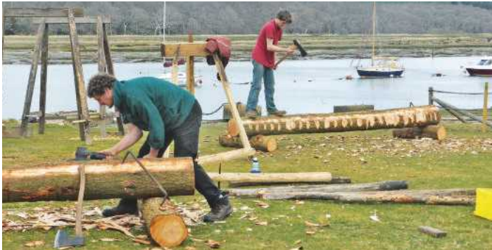
Pic.3 The first stage of hewing is snapping lines along the logs to give the required size. Notches are then cut almost down to this line with a felling axe. The final trimming off exactly to the lines is done with a side axe, which has a cranked handle and the blade bevelled on one side only. The side axe is a specialised timber conversion tool in contrast to the general-purpose felling axe. The timber 'dogs' bite hard into the timber and stop it rotating
