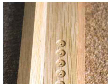
▲ Pic.21 Drill the frame at each position to a depth of 1mm
