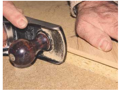
▲ Pic.9 Cut the MDF and trim to fit the frame. Bernard used a makeshift shooting board for this
