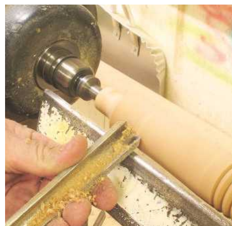
▲ Pic.27 To make the legs look lighter turn away some of the material to left and right of the beaded detail in the middle, using the small roughing gouge for more control
