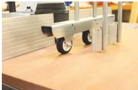
▲ These wheels allow the work to pass through easily
