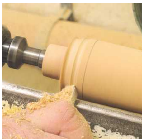
▲ Pic.23 Using the spindle gouge turn half a cove down to the diameter of the spigot, pick up the cut with the flute towards 9 o'clock and then open up to 11 o'clock as you progress
