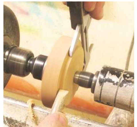
▲ Pic.33 All that's left to do is turn the cap to go into the recess. A piece of ash from the same board is cut to size and mounted between centres
