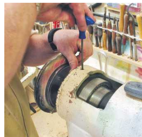
▲ Pic.9 Les likes to drill the leg holes now, using the indexing system on the Oneway lathe, but this could be done afterwards on a pillar drill
