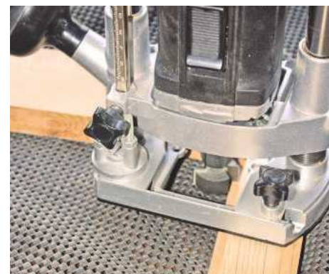
▲ Pic.6 Cut a rebate in the frame slightly smaller than the panel...
