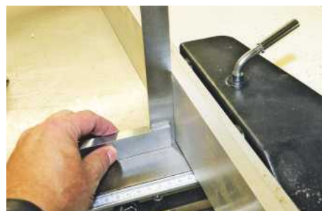
▲ Adjustments are via the running rail or the fence
