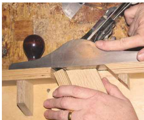
▲ Pic.4 Once bottom/top panels have been picked remove waste and trim angles on shooting board
