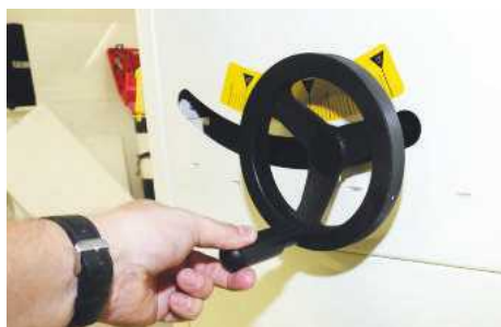
▲ Two smooth-running handwheels set the blade height and angle
