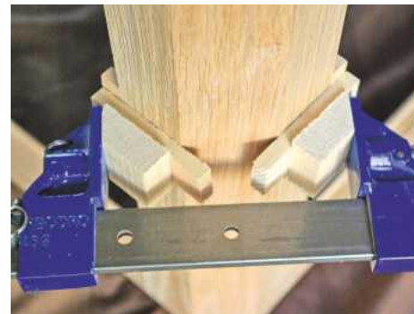
▲ Pic.24 A quantity of clamping blocks will be needed for the assembly of the main frames
