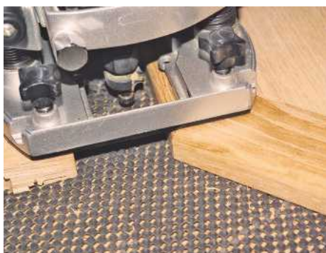
▲ Pic.28 With a 6mm bearing-guided ovolo bit, trim the underside of the bottom panel only
