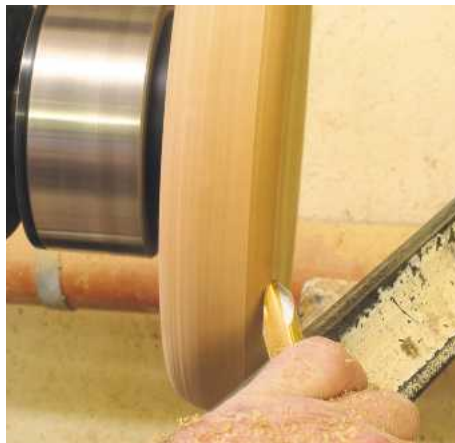
▲ Pic.14 Once it's mounted on the chuck round over the edge with the gouge. When doing a pull cut don't hang the tool too far over the rest as you could lose tool control
