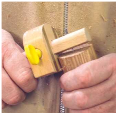
▲ Pic.17 To mark the centres on the legs Les uses a marking gauge. Set the point up on or near the centre and mark it all the way round
