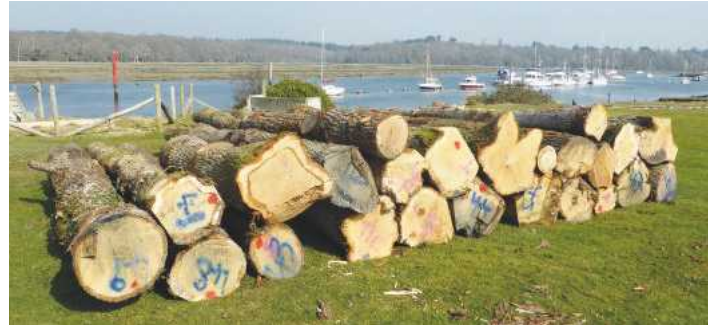
Pic.2 The marked logs were brought to site and stacked in the order in which they would be needed. These logs show the quality and size easily available today from English woodlands. While not joinery grade it is fine for construction
