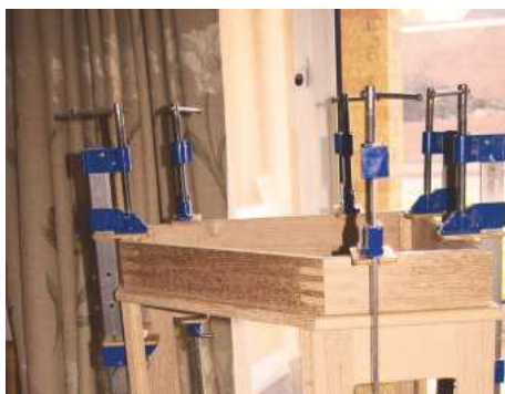
▲ Pic.29 The main frames were cramped to the base panel and plinth, then left to set
