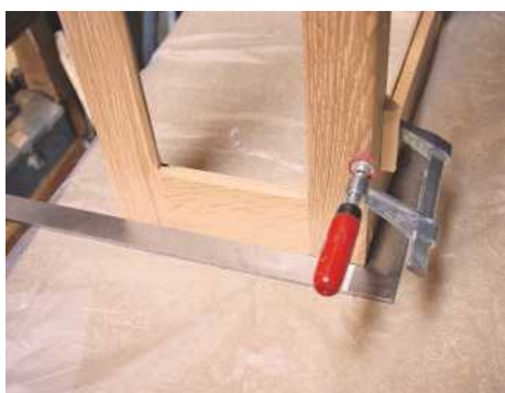
▲ Pic.25 In a similar manner assemble and glue the side frames to the back frames
