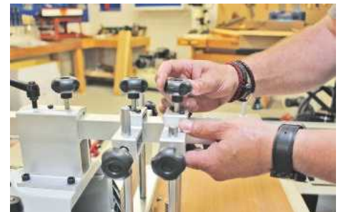
▲ Heavy box sections ensure the guards stay rigid under load
