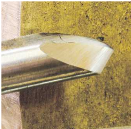
▲ Pic.5 As Les needs to remove timber quickly he is starting with a 13mm bowl gouge with a long or Irish-type grind; the quality of the sharpening when using a jig produces a really clean bevel and a 55° angle
