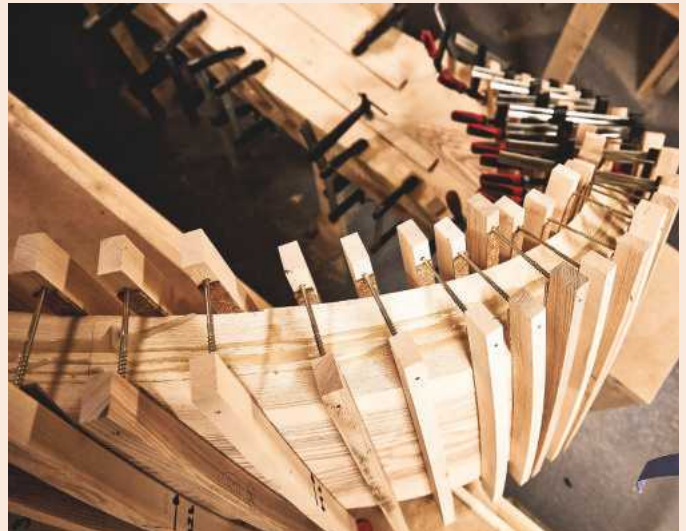
Battens and screws put on the pressure
