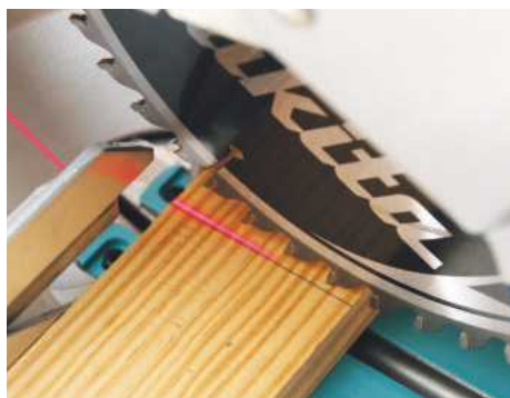
▲ When the head descends you can see how far out the laser is to the line
