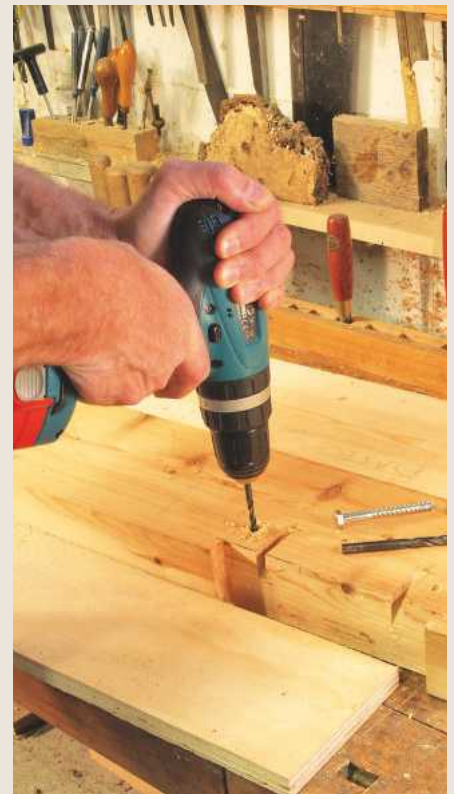
Pic.9 Drilling pilot holes
