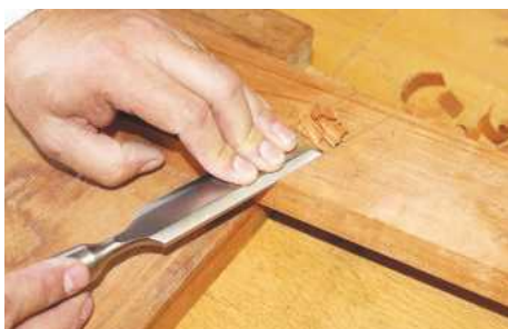
▲ Paring waste from housings is an area where the chisels work well
