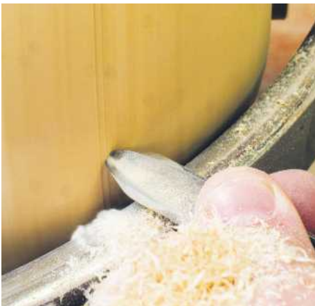
▲ Pic.22 He is running his finger along the toolrest while making a push cut with the bevel rubbing; the finish off the tool will be really good and the surface will not need heavy sanding
