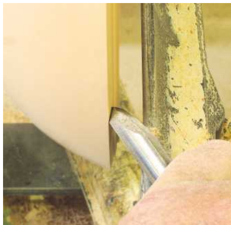
▲ Pic.26 To ensure a good surface finish care needs to be taken with the finishing cut on the rim; sometimes Les goes down to a smaller tool if he thinks the cut would be better
