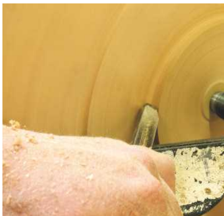
▲ Pic.10 Unlike the small bowls the big one for the main prize is having a large base so Les is turning a chucking point with oversize spigot that can be reduced when the bowl has stabilised
