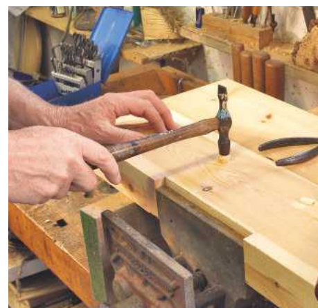
Pic.15 Fitting plugs to the counterbores
