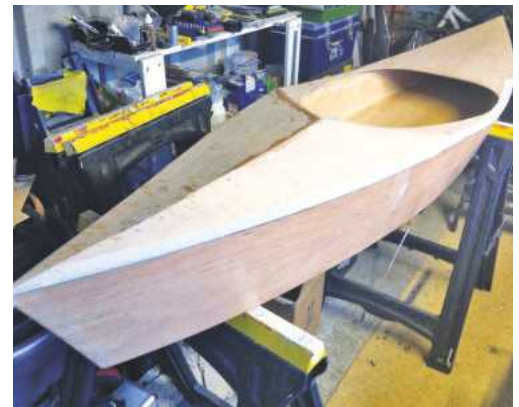
Pic.13 Filling any gaps between deck and hull
