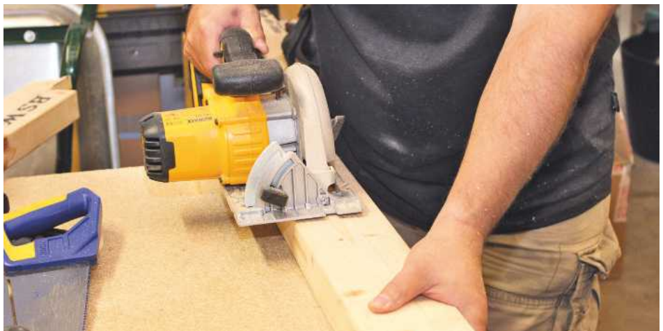
▲ Cutting notches in 45mm stock was well within the saw's capabilities
