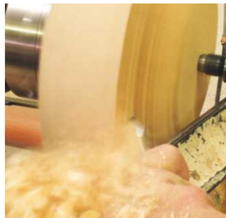
▲ Pic.12 Because he is only part turning the bowls today he is pull cutting with a really aggressive cut that is producing a lot of shavings
