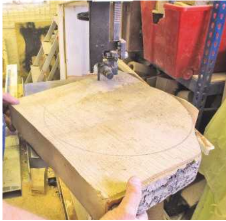
▲ Pic.2 Once the blanks are marked out with a compass cut them to rough circles on the bandsaw using a 10mm blade with 3 or 4tpi; a 100mm-diameter blank is achievable with this setup
