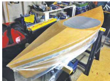
Pic.15 Epoxy resin applied to cloth over deck and roughly trimmed to masking tape line
