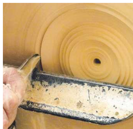
▲ Pic.15 Les hollows the bowl as normal; as it's only going to be part turned at this stage speed rather than finish is the key factor
