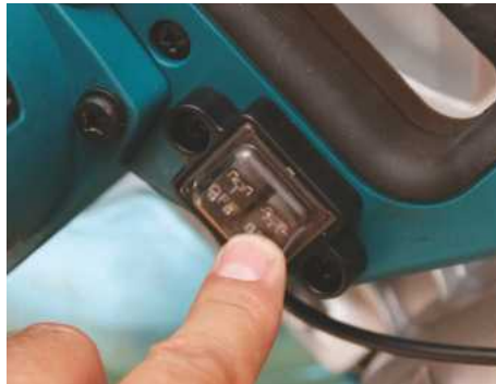
▲ The light and laser functions are independently switched
