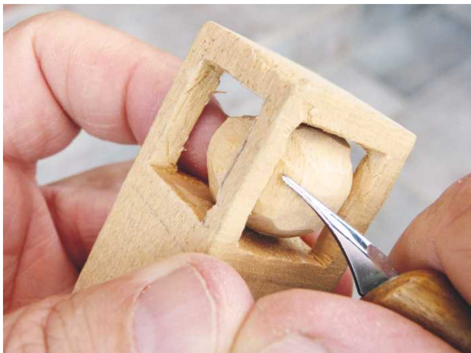
Pic.11 The freed shape will probably need a lot of work to get it spherical; use your forefinger and thumb to secure the shape when carving
