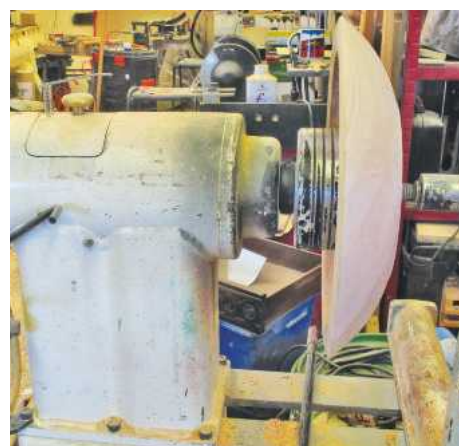
▲ Pic.33 His vacuum chucking system allows easy remounting of the bowls to remove the spigots; they could have been mounted between centres to cut away excess stock, leaving a small amount to be done by hand
