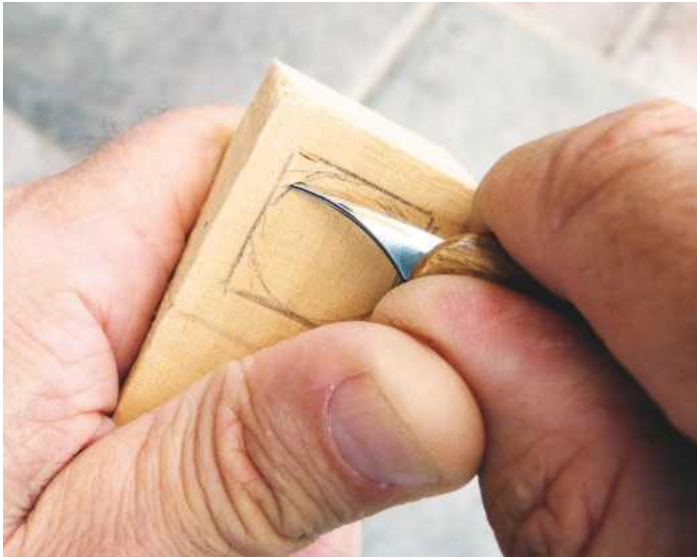
Pic.4 Pare out the timber between the two cuts then repeat this process on all the four sides of the block
