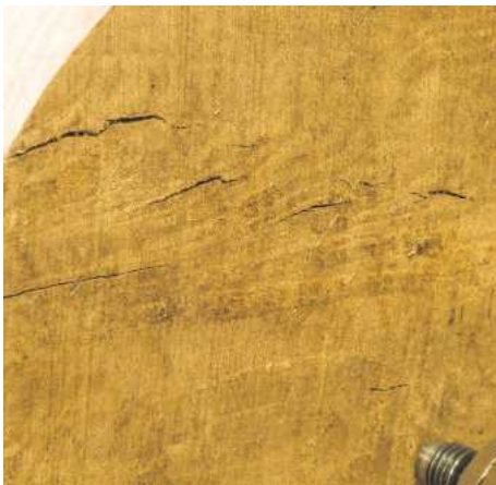
▲ Pic.4 These faults or surface checks appear during the drying process but mounting the timber in a particular way should mean they disappear in the turning
