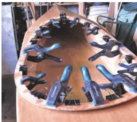
Pic.17 Building up the coaming around the cockpit
