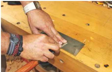
▲ Prepping the 25mm chisel with a few quick laps on the coarse diamond stone...
