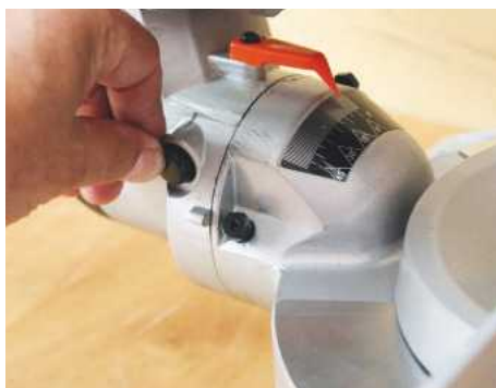
▲ There's an override button to gain an extra couple of degrees on the bevel settings
