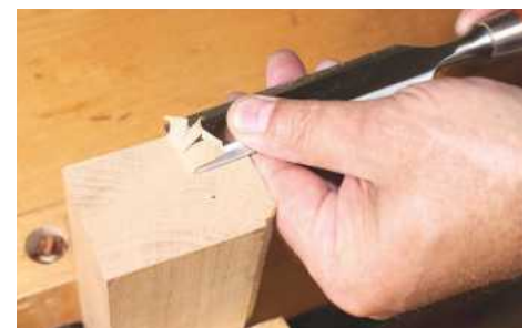
▲ You can get very keen edges for end-grain paring
