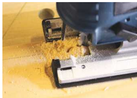
▲ There's a pendulum action but no blower so dust builds up around the cut line
