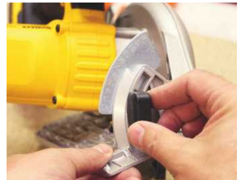
▲ The solidly cast base includes a protractor scale for locking angles
