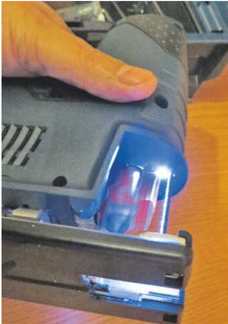
▲ It provides a good flood of light to the work area
