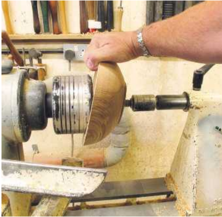
▲ Pic.19 After a week or so it's time to remount the bowls and complete the turning; Les is mounting them between centres using the tail stock and a friction chuck
