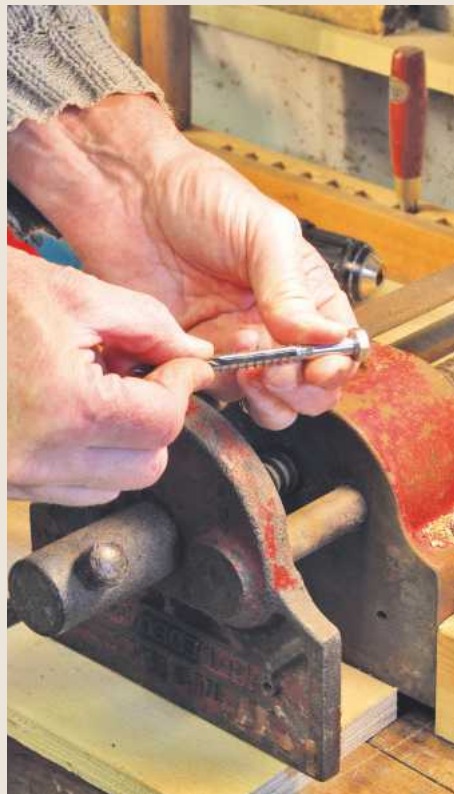
Pic.7 Eyeballing the shank of a screw against a suitable drill bit
