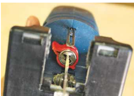
▲ When correctly fitted the collar wraps around the blade shank
