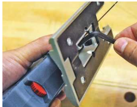
▲ There's a hex key adjustment for tilting the base
