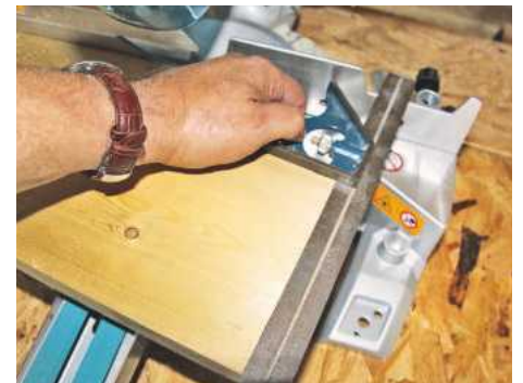
▲ Checking the cut on wider stock off the saw shows it is smack on
