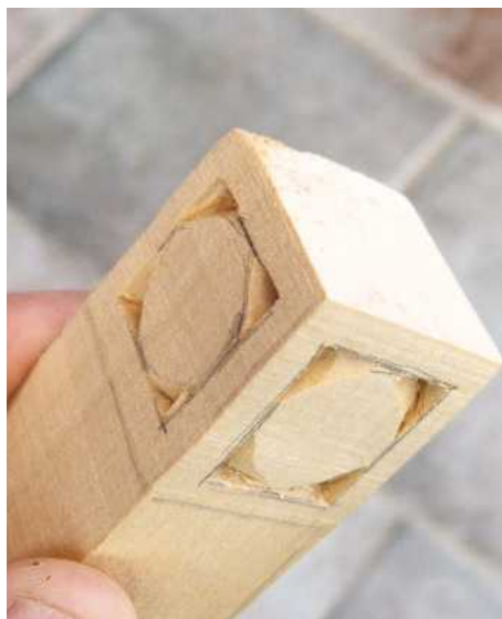
Pic.7 Continue the process, using the larger knife to cut deeper and taking care not to cut into the frame
