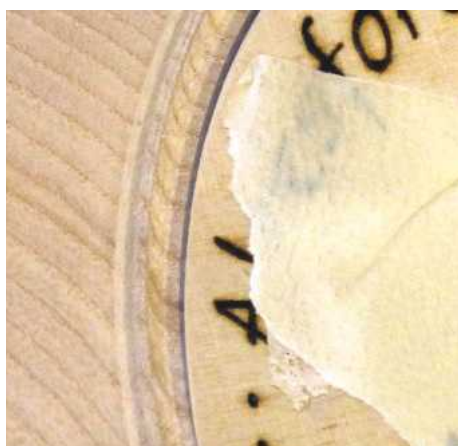
▲ Pic.32 Turning a small bead on the hole edge disguises any looseness of the discs in the recess; he uses an Ashley Iles bead-forming tool, taking care not to break away the bead top
