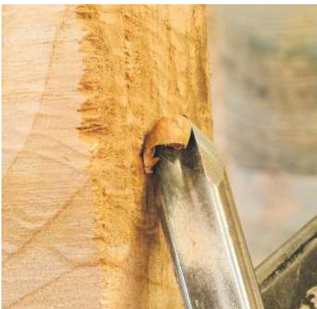
▲ Pic.7 When pull cutting with a long grind the flute is pointing almost upright and the shaving is cut on the left-hand side, rolling round the flute and coming out the right-hand side
