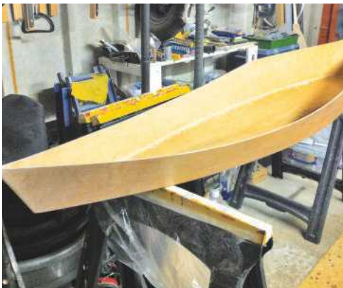
Pic.11 The hull glassed inside and out and edges trimmed
