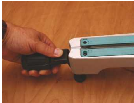
▲ Mitre angles are set and locked with the front handle
