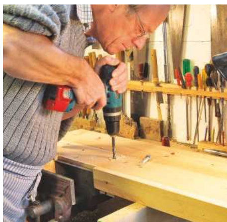
Pic.12 Enlarging the main hole to take the bolt shanks
