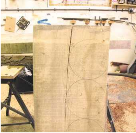
▲ Pic.1 Les has had this 75mm-thick ash for a number of years. The moisture content is around 18%, so the timber is likely to move after it's turned
