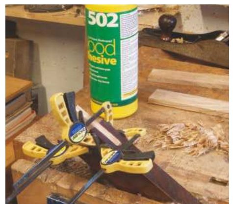
Pic.6 New tenon glued in place with PVA
