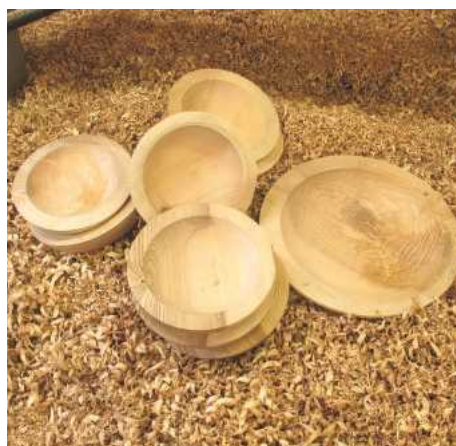
▲ Pic.17 Here they are all roughed out and left to do their settling down; the large amount of shavings indicates that most of the stock has been removed
