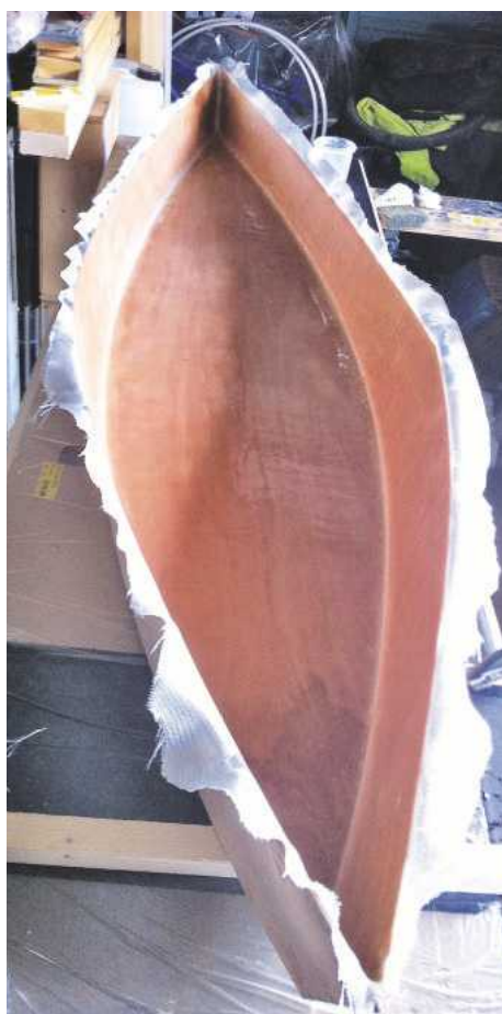
Pic.9 Glassing the inside of the hull
