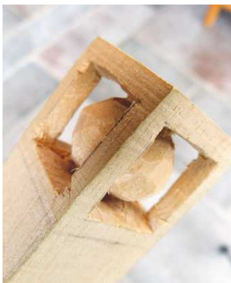
Pic.10 Carefully work away and separate the sphere from the frame and the top and bottom of the box
