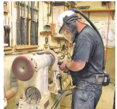
▲ Pic.24 Once turned the piece will need sanding; Les has elected to power sand the outside and the drill is tucked into his side as he moves his body through the curve of the shape
