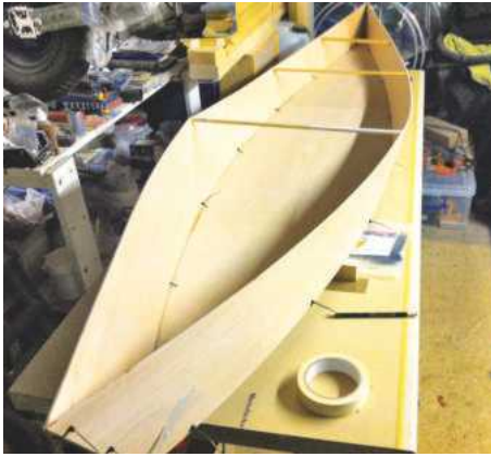
Pic.5 Zip ties hold the hull in shape with temporary spreaders
