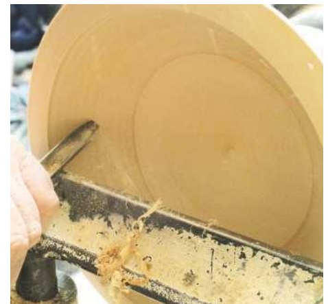
▲ Pic.27 He always tries to get the finish and shape that he wants using the gouge; if you have to use a scraper take very light cuts and if the bowl has moved at all do not go back to the edge
