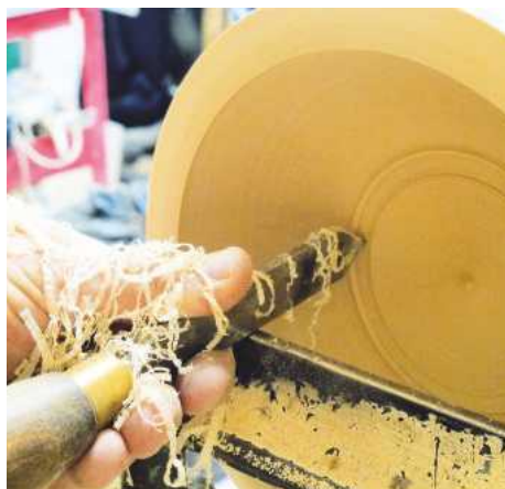
▲ Pic.29 Make a cut with a parting tool to mark out the size you need; for speed Les removes most of the stock with the gouge
