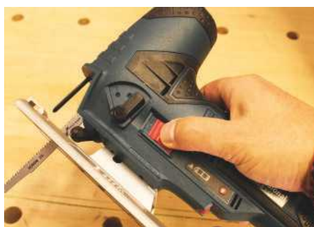
▲ The slider is positioned more favourably for right-handers
