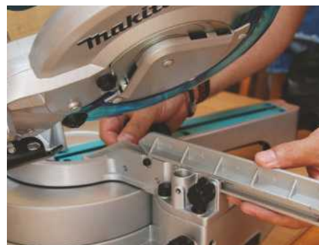
▲ The saw tilts to the left and the fence slides away to accommodate it
