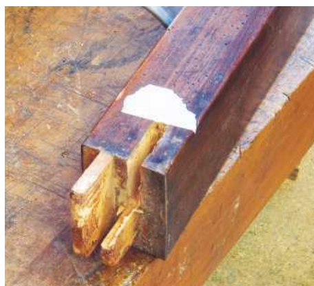
Pic.5 Slot routed for replacement tenon
