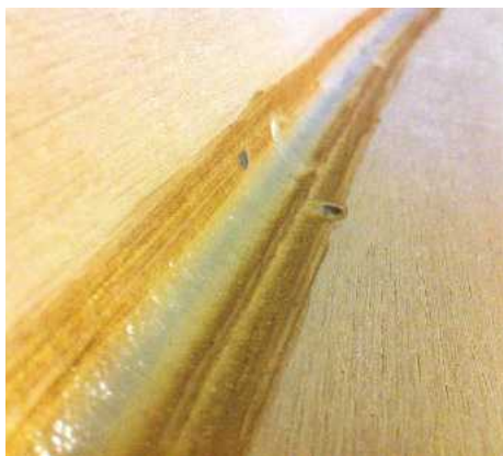
Pic.8 Final large bead of epoxy along the seams
