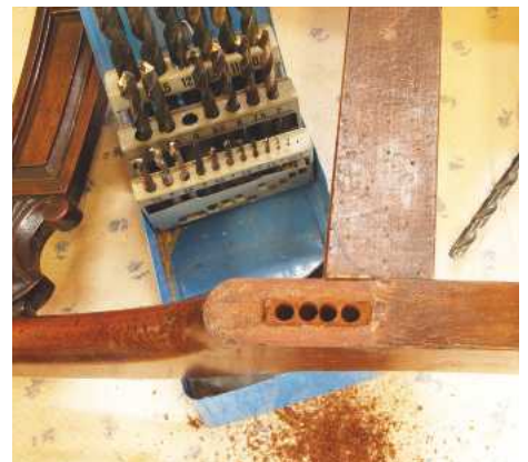
Pic.3 Controlled incremental freehand drilling to remove the waste
