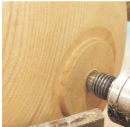
▲ Pic.23 Les has cut a little flat by the side of the chucking point; this will act as the base when the spigot is removed, giving the top of the chuck jaws something to bear on when he is hollowing
