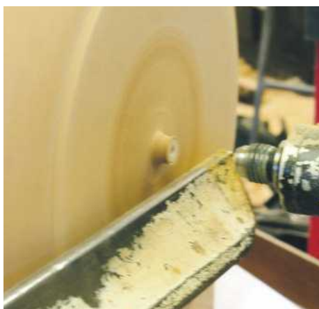
▲ Pic.34 Taking away the tailstock to finish off the last bit is always a leap of faith, with only atmospheric pressure keeping the piece on the lathe – hopefully there won't be a power cut!
