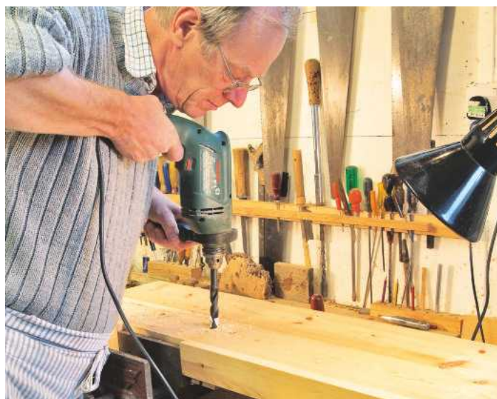
Pic.11 Counterboring; note the masking tape flag as a depth gauge
