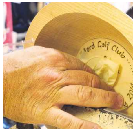
▲ Pic.30 Trying it for size: attaching a piece of tape to the front side means you can get it out if you happen to cut the recess a bit snug
