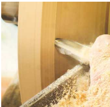
▲ Pic.11 Not yet! He could do a push cut with the bevel rubbing at this stage but this would not shape the wood quickly; he likes to use this technique when getting near the final shape
