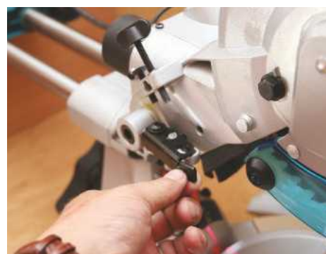
▲ The flipstop function allows you to swap between trenching and full cuts with ease
