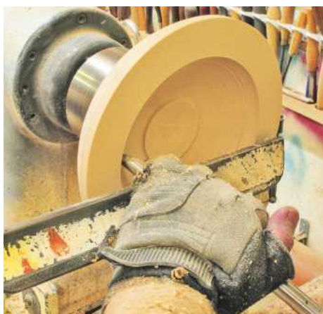
▲ Pic.16 The size of the cuts necessitate a glove on Les's left hand to stop his hand getting sore from the heat of the tool and the sharpness of the shavings
