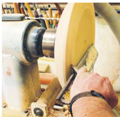
▲ Pic.14 When all the bottoms are done, it's time to turn the tops; the rim is turned first; putting a little curve on the top of his bowls adds to the overall design
