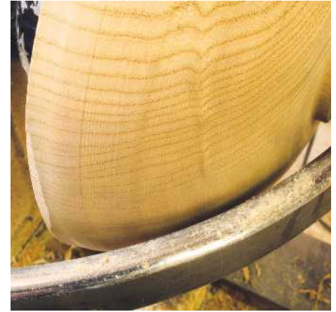
▲ Pic.21 One of Les's luxuries: a stainless-steel curved toolrest from Oneway manufactured in Canada; if he gets the shape of the bowl close to the curve he will achieve a good bowl
