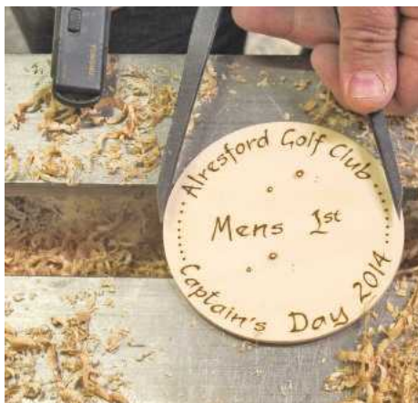
▲ Pic.28 He needs to transfer the diameter of the discs to the bottom of the bowl; he is going to leave them slack in the bottom to allow for movement
