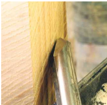
▲ Pic.8 Not this way! The closed flute will cause the tool to scrape the wood, blunting the tool really quickly and not cutting much timber away
