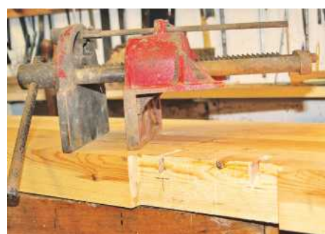
Pic.5 Slots cut and ready to receive the fins
