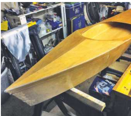
Pic.16 Glass cloth trimmed and masking tape and protective plastic removed
