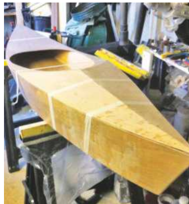
Pic.12 Starting to locate the deck onto the hull
