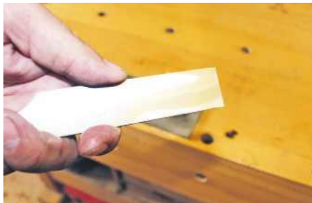
▲ ...reveals a long hollow extending to the cutting edge
