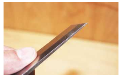
▲ The lands taper finely – ideal for cleaning into tight corners
