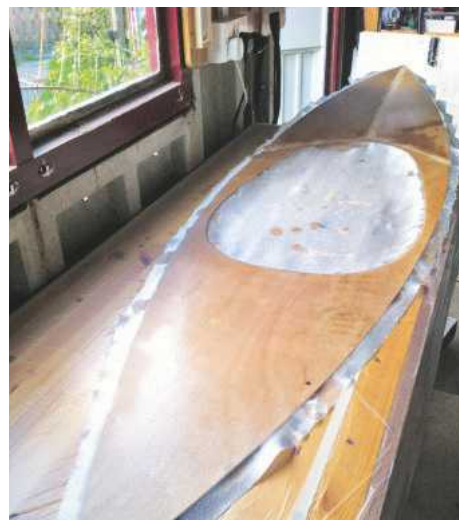
Pic.10 Glassing the underside of the deck
