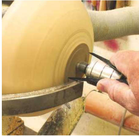
▲ Pic.20 The size of the spigot or chucking point will determine the base on which the bowl will stand; only touch the wood with the left-hand point of the dividers
