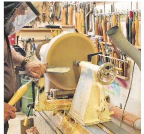
▲ Pic.6 For protection he wears a respirator and tucks the tool into his side; the tail stock adds security – you never know what is hiding inside wood like this
