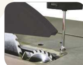
Height & side setting of the scoring blade conveniently accomplished with the tool provided.
