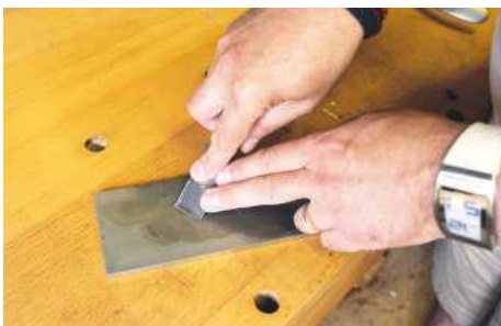
▲ After a few minutes lapping to get the area behind the edge flat it's ready for edge honing
