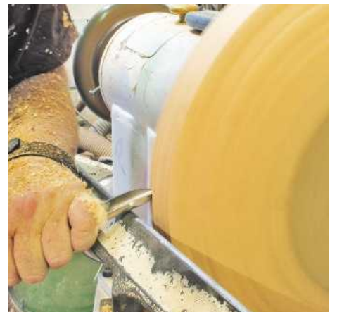
▲ Pic.9 The edge is achieved with a push cut; the flute is now pointing away from Les – keeping him out of the firing line from loose bits – as the tool is eased through the wood
