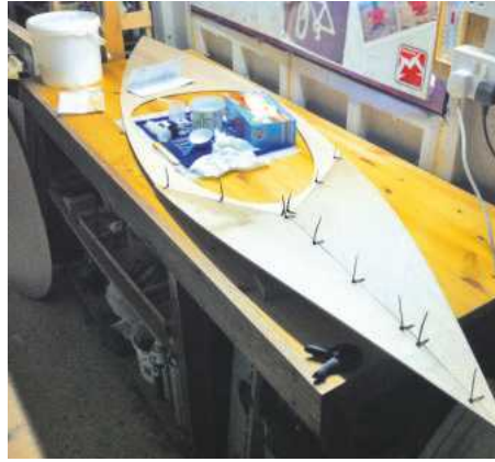
Pic.6 The upside-down deck zipped together
