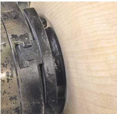
▲ Pic.25 You can see the importance of the flat part on the large bowl; the top of the jaws have located perfectly onto the surface
