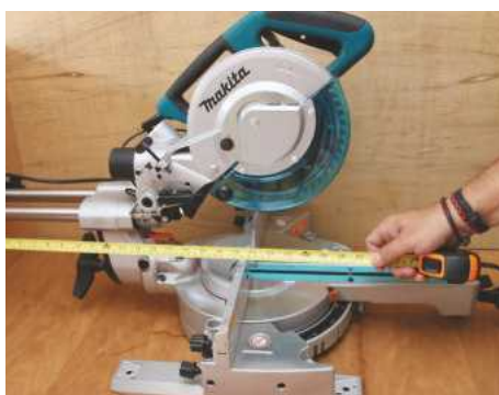
▲ You need about 700mm to sit the saw on and allow the bars to run their arc
