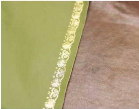
▲ Pic.17 Finally trim the skiver so it fits the rebate tight at the veneer edge
