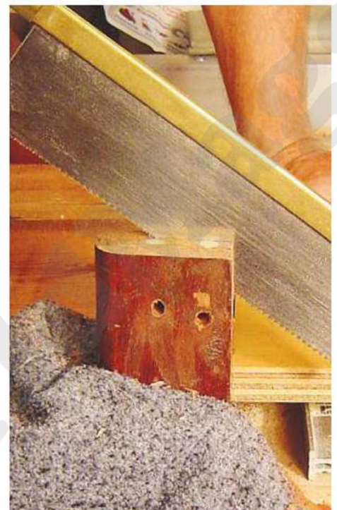
▲ Pic.7 Cut the tenon shoulders
