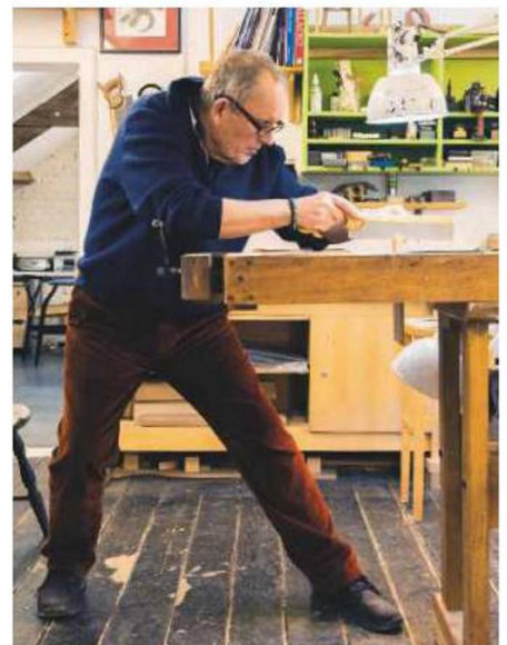
...aim for a stance that has the saw extending your arm in a straight line
