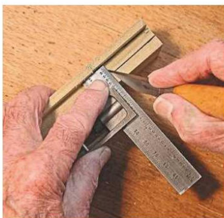
▲ Pic.8 Restoring the cut line removed by the rebate plane
