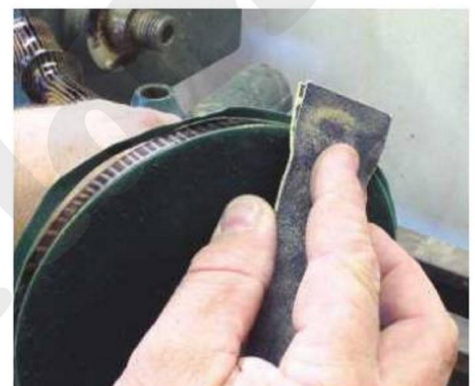
▲ Pic.26 Cutting the baize with abrasive produces a neat result
