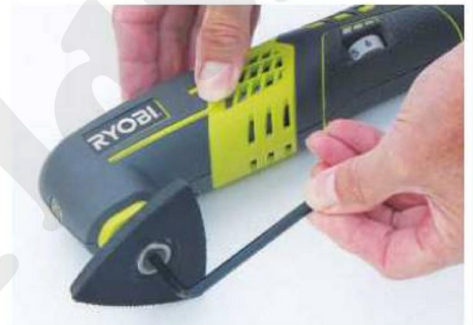
Changes are effected with a hex key
