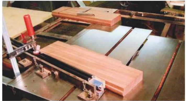
▲ Pic.2 Shoulder cutting on the dimension saw using the fence stops
