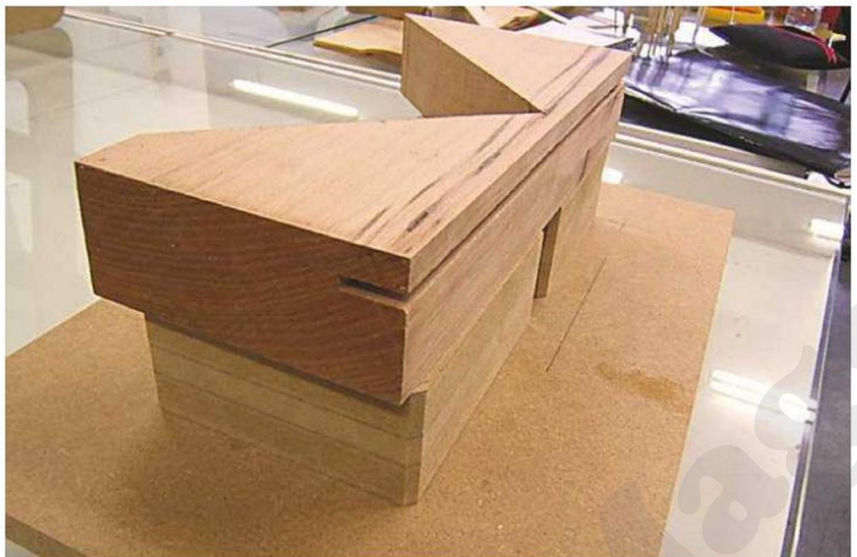
The walnut box tops simply slot into the jig which is passed across the cutter
