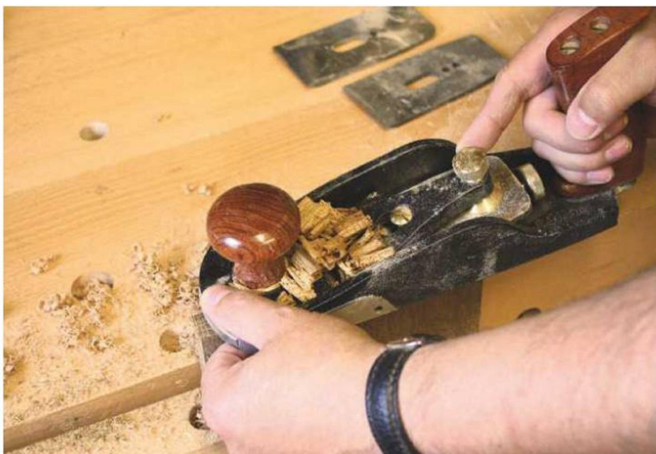
▲ Next stage was the end grain oak, with clean shavings still being cut
