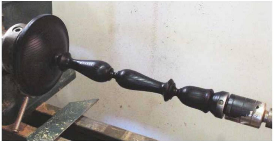
▲ Pic.20 Mounting the candlestick between centres on the lathe means your hands can be kept off the work while applying the gilding wax
