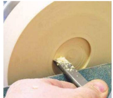
▲ Pic.5 The dovetail angle must closely match the one on the chuck
