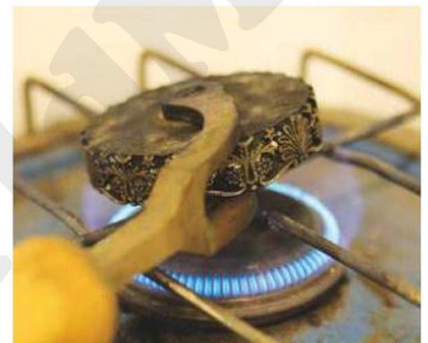
▲ Pic.6 The Greek key pattern embossing tool being heated
