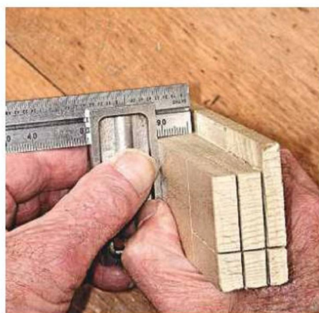
▲ Pic.9 Testing to ensure that the long shoulder squarely abuts the rebate's land
