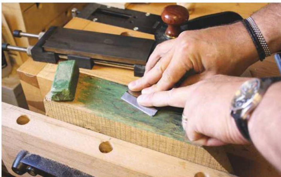
▲ The Andy King 'Scarcely Sharp' honing set up comprises a Trend diamond stone, some Veritas green honing compound and a piece of flat oak
