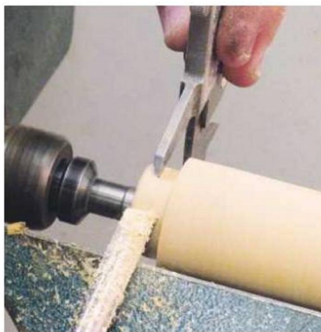
▲ Pic.13 With the callipers set to the diameter of the base hole, the left-hand end is turned down
