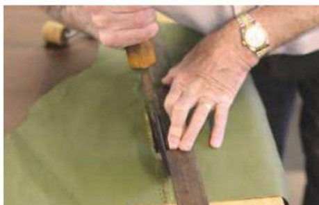
▲ Pic.12 ...and to finish runs a 'blind' line over the seam – perfect!
