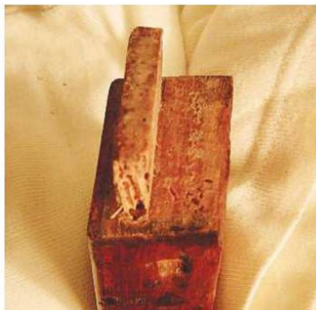
▲ Pic.10 The wormy-riddled 7.5mm tenon...
