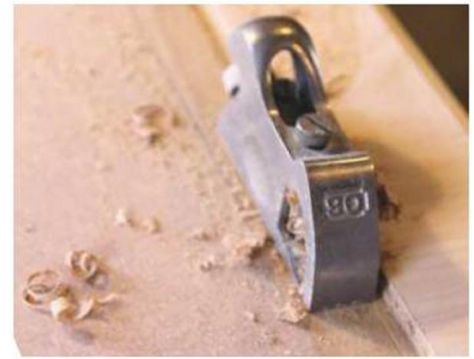
▲ Pic.16 ...and using a bullnose plane make a shallow chamfer down from the line
