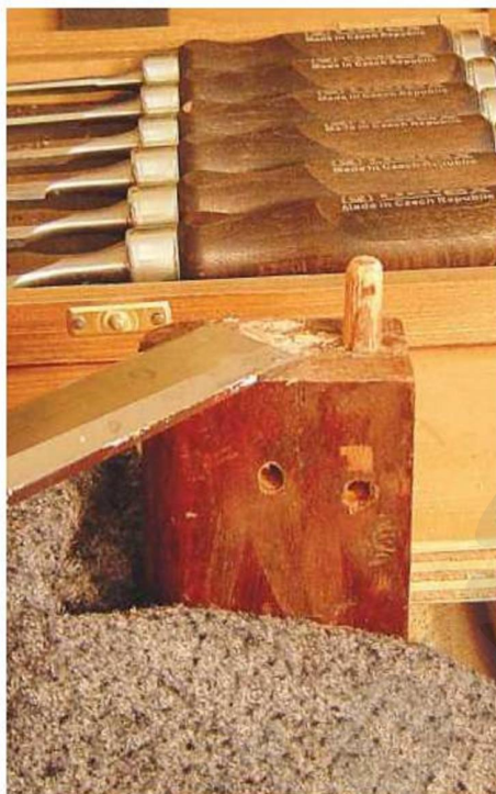
▲ Pic.6 Cut and trim the dowels
