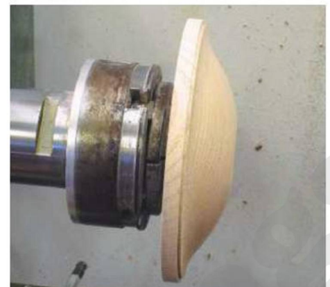
▲ Pic.7 ...a shape that requires just a small fillet and an ogee
