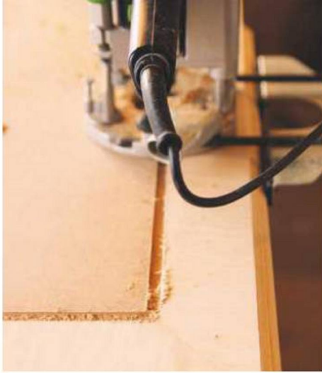
▲ Pic.14 Use a router to cut an 8mm by 5mm rebate...
