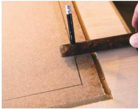
▲ Pic.15 ...then mark a line 30mm in from the rebate...
