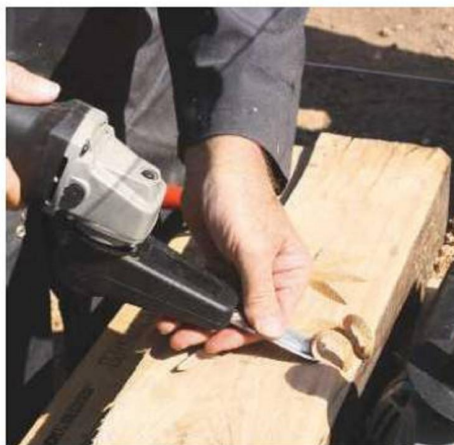
The Power Chisel makes carving lettering or adding detail a doddle
