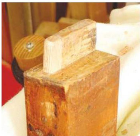
▲ Pic.11 ...and the 8mm dowel repair
