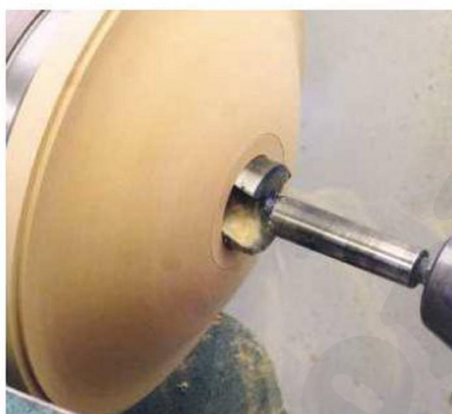
▲ Pic.8 The hole for the stem is 30mm diameter
