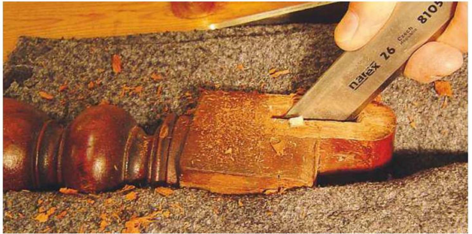
▲ Pic.5 Remove the broken tenon
