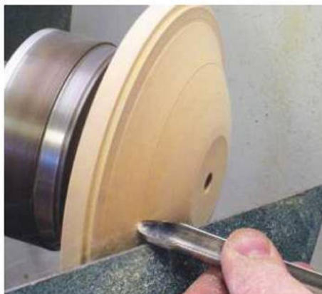
▲ Pic.6 Put the wood onto the jaws and get ready to turn...
