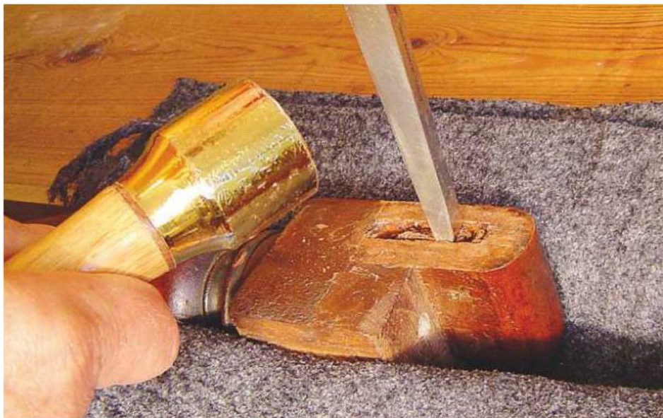
▲ Pic.8 The mortise in the stretcher had to be cut by hand
