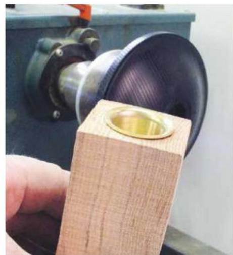
▲ Pic.12 The large hole requires use of a large-diameter point on the live centre
