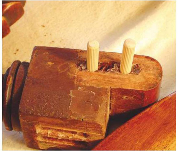
▲ Pic.3 Dowels in failed tenon
