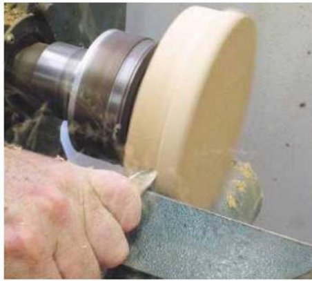
▲ Pic.2 The bottom surface needs to be slightly concave...
