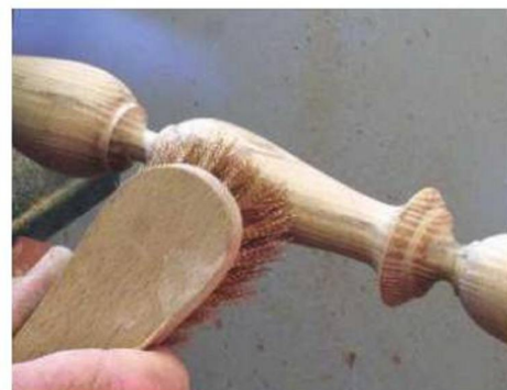
▲ Pic.19 ...to prepare the surface for the ebonising lacquer
