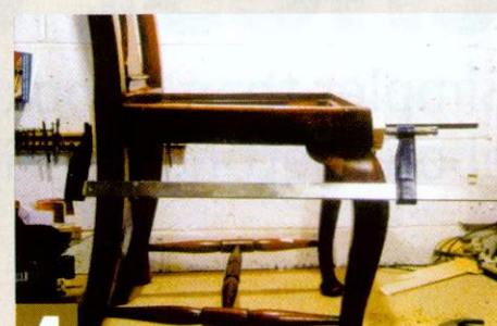
4 Cramp lightly to pull up the joints: a band clamp is very useful for these square-off situations. Put in the drop-in seat to check the cramping has not pulled the chair off square
