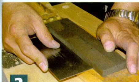
3 Polish the scraper faces to remove any burrs, repeating the edge stroke if needed
