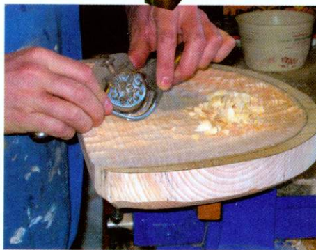
▲ Pic.1 A hollowing spokeshave is great for the final shaping and for a fine finish
