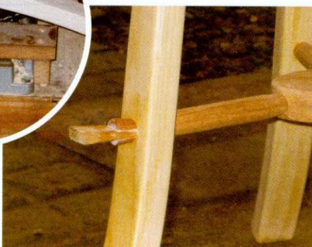
▲ Pic.8 The 1in excess on the tenons can be trimmed back later once the glue has set
