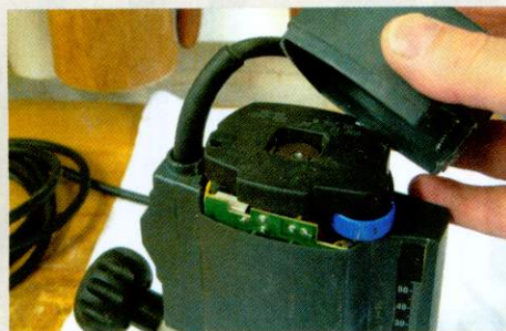
▲ Pic.2 This is the speed sensor mechanism. It does not need to be disconnected
