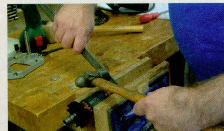
▲ Pic.10 The top bearing is a bit tricky to deal with. Be careful not to damage the armature
