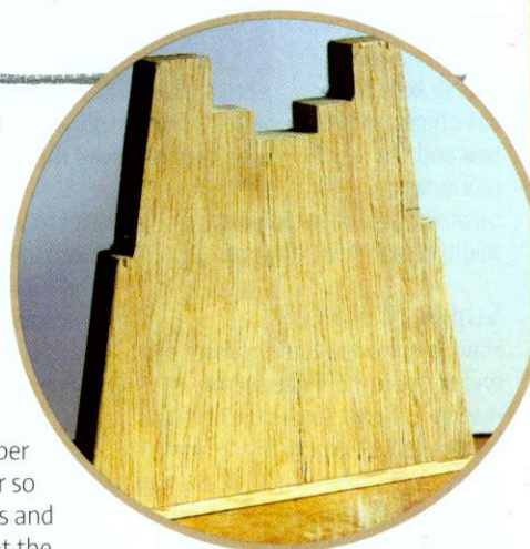
▲ The end support brace was cut from 1inch plywood
