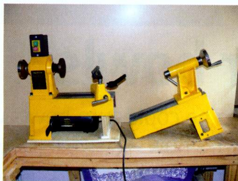
▲ Terry had to support his lathe at the cut part after he'd removed the legs from one end
