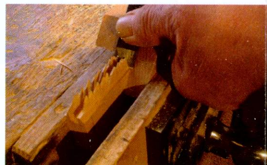
▲ Bill Newton was cutting the mason's mitre in grooved stock. He used the 45° guide to feather the stock first to make it easier to pare back to the line of the moulding
