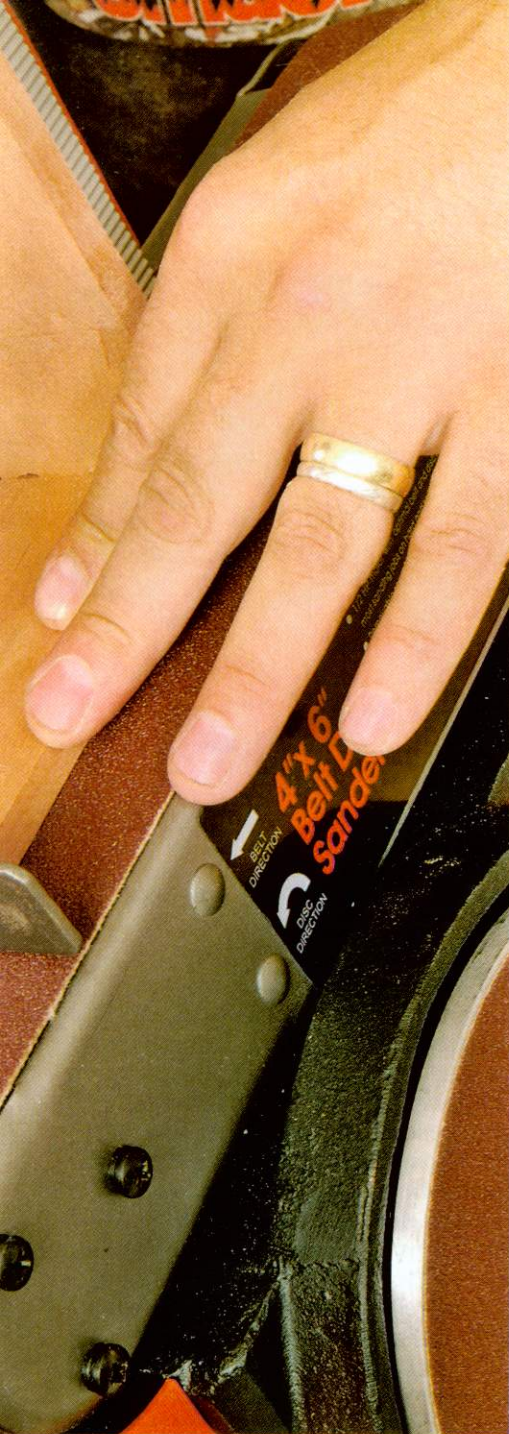
▲ There is a simple metal end stop that prevents any workpiece being dragged off the end of the belt
