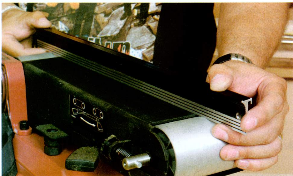
▲ The platens were tested for both flatness and twist, to ensure the accuracy of any work
