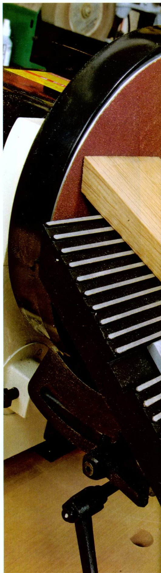
▲ This three-point bracket is used by the other sanders. It's still fully adjustable, but only supports one side of the table
