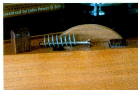
▲ Pic.3 The catch itself should be hard because it has to withstand wear during use
