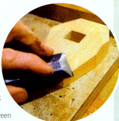
▲ Pic.1 Bevel the wallplate with a sharp chisel, or rout a moulding around the edges
