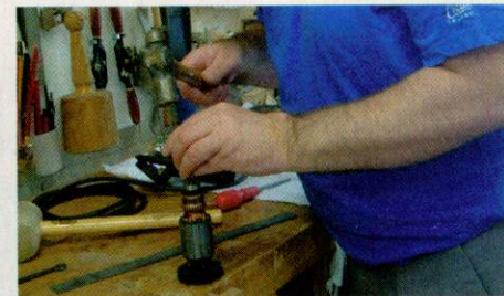
▲ Pic.11 Happily, replacing the top bearing is a bit easier than taking it out
