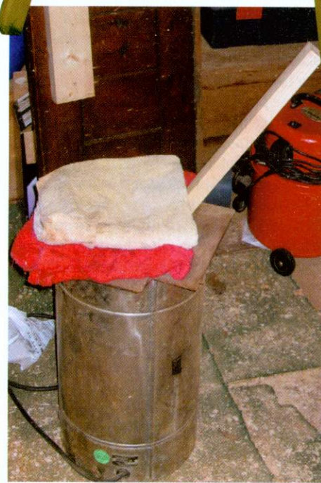
▲ Pic.3 Wade's steamer is a converted tea urn, with only a small part of the leg needing to bend
