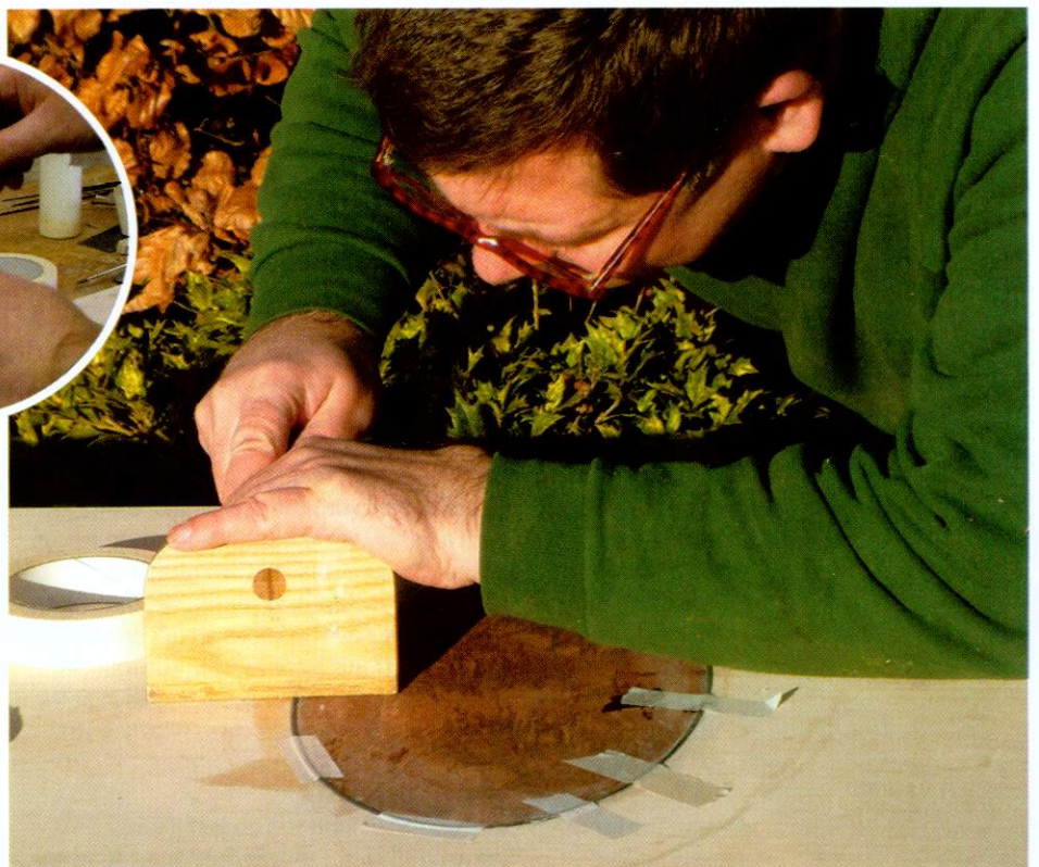
▲ Pic.8 The stringing is hammered in, then it can be persuaded in without breaking: it must be heated (inset) so that it can be bent to such tight curves
