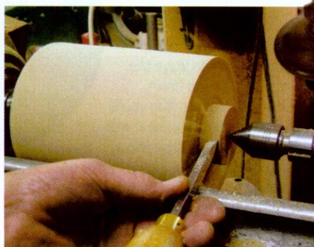
▲ Pic.6 Use the parting tool to turn the spigot for your combination chuck
