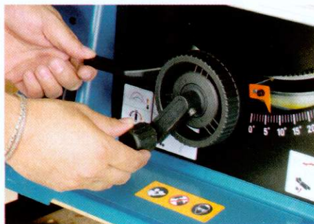
▲ All the blade adjustments are carried out from the front of the saw
