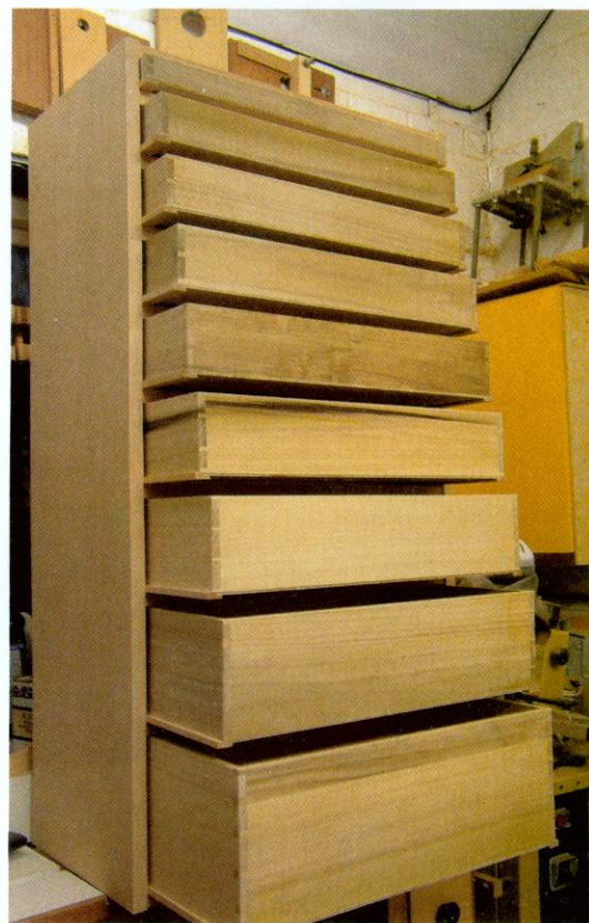
▲ Pic.5 The basic carcass is all rectilinear, making construction easier than it looks
