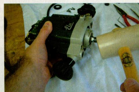
▲ Pic.8 Remove the four screws from the bottom casing to separate the two halves
