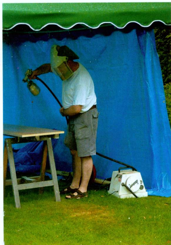
▲ The tarps hang with shower curtain rings, and boards hold them down. It's cheap and cheerful but quite effective for occasional use
