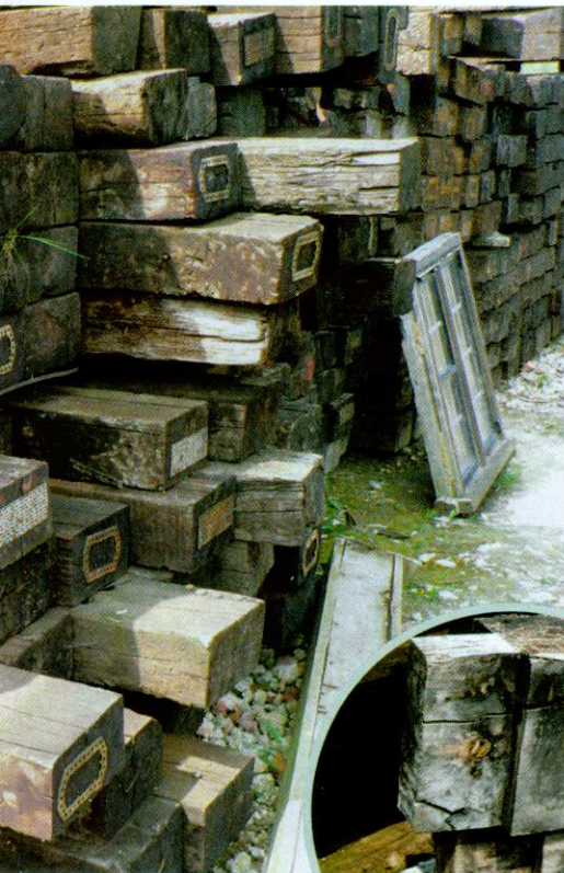
▲ Creosote-treated railway sleepers and (inset) old oak beams
