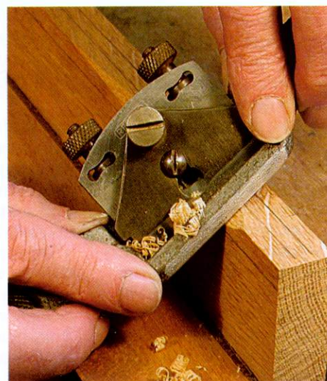
▲ Pic.5 If the spokeshave goes further than this, the apex of the curve will be spoilt
