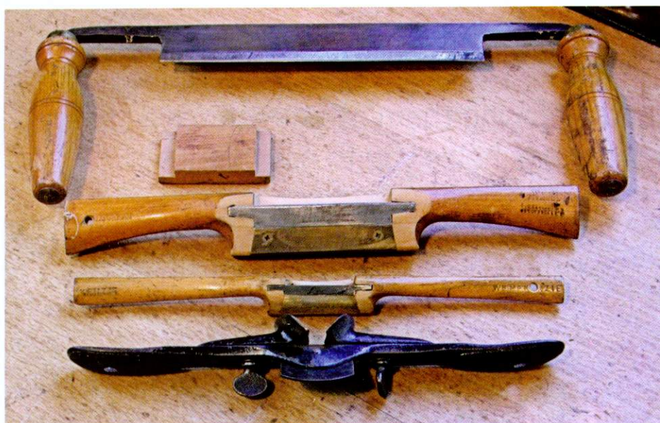
▲ Pic.7 Top to bottom: a drawknife; a simple pencil gauge; a flat-faced wooden spokeshave; a small round-faced spokeshave and, for the old-tool buffs, a Stanley spokeshave with wing-like fences
