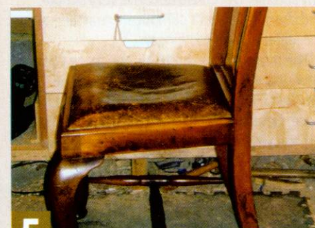
5 After screwing and gluing the corner blocks, with a little candlewax on the threads to help, the chair is finished.
