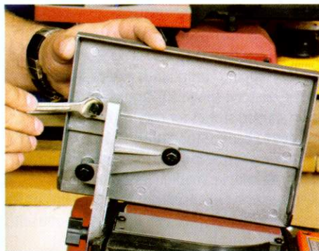
▲ This three-point bracket is used by the other sanders. It's still fully adjustable, but only supports one side of the table
