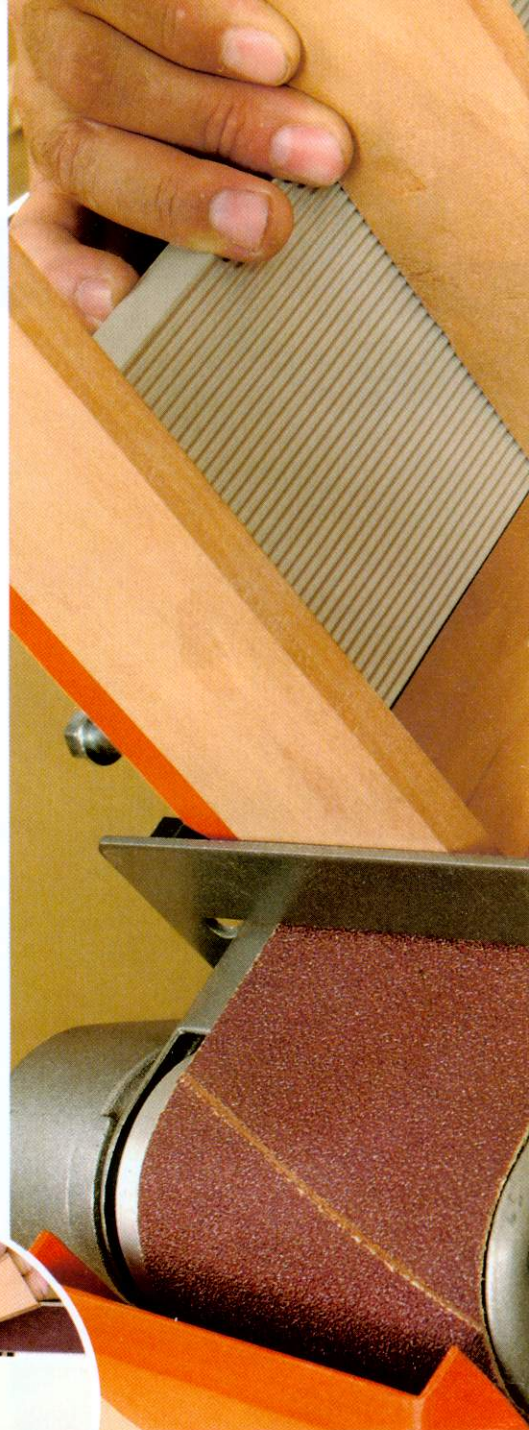
◀ The wheel of the belt is perfect for concave curves up to the diameter of the wheel itself
