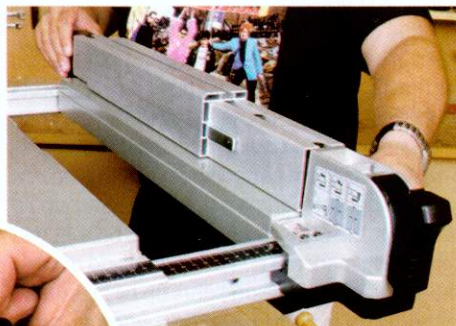
▲ The fence extends on rails to allow ripping up to 625mm ▲ The fence locks firmly at the front and rear with this cam lever
