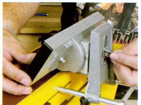
▲ This double post and trunnion found on the Perform and SIP models is far better, staying parallel as it alters
