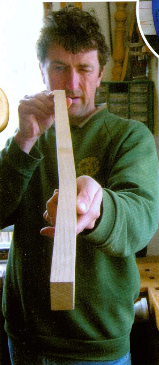
▲ Pic.4 Left for a night in the former the leg will be bent permanently
