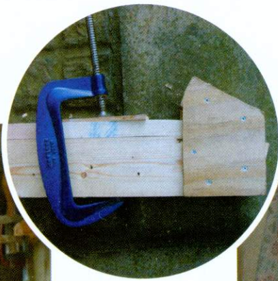
▲ Pic.5 The former is simply a piece of 4x2in pine with a cleat at the end to hold the part that's to be bent
