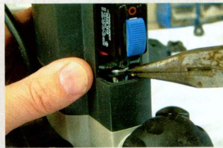
▲ Pic.5 With the plunge locked down, you can get access to this circlip from the switch box
