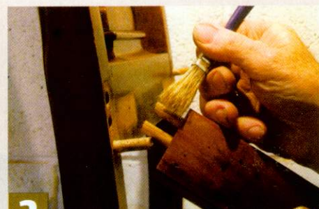
3 Apply hide glue to the dowels, which was the original adhesive, and is therefore 'restorer-friendly'. Assemble on a level surface to avoid adding wobble
