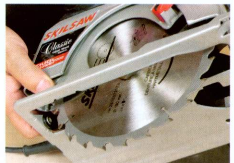
▲ With no riving knife it's simple to drop the saw through the centre of a board
