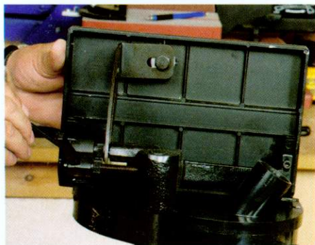
▲ Rexon and Axminster have a yoke to support both sides of the table. It's fully adjustable to get it parallel to the abrasive
