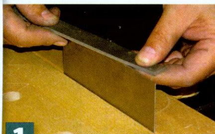
1 The edge of the scraper is dressed at 90° with a bastard-cut flat mill
