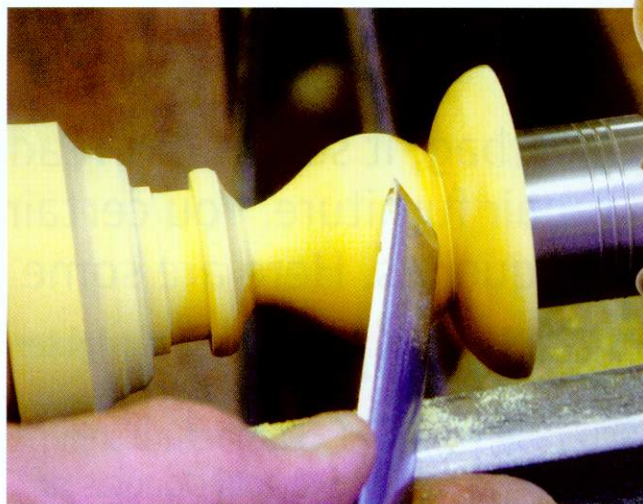
▲ Pic.8 Using the skew chisel like this will leave the surface with a good finish
