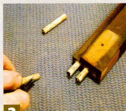
2 Take out the dowels, scrape them clean of the old glue and clean out the holes. If there are no grooves to allow surplus glue to exit, cut some as shown using a carver's V chisel
