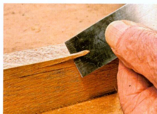
▲ Pic.2 If allowed to go too far, a split will ruin your chance of making a good chamfer
