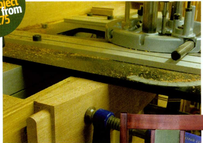
▲ Pic.5 Routing the housing in the back support: notice that waste is used to pack the piece accurately
