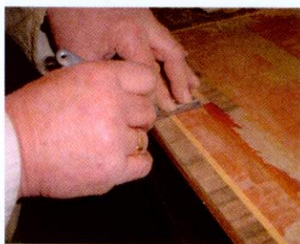
▲ Pic.26 Making the joints in the cross banding with a knife
