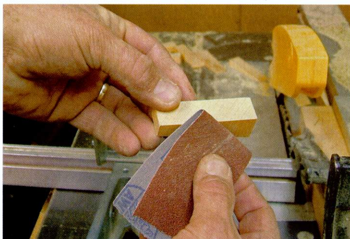
▲ Pic.6 De-nib the segments before gluing them together
