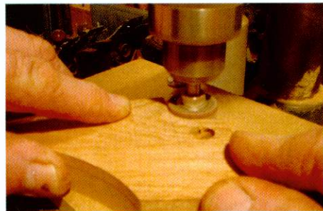
▲ Pic.5 Sanding the notches in the feet with a bobbinsander to get a smooth curve
