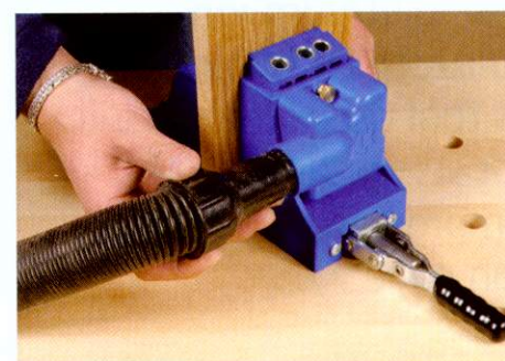
▲ Dust is minimised with the extraction port, but this makes setting the indent screw awkward
