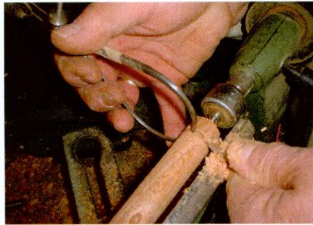
▲ Pic.3 Use callipers to size the tenons on the end of the legs and stretchers accurately
