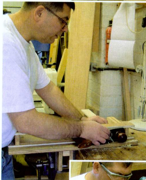
◀ Pic.2 The drawer components must be dead square, so a good shooting board is essential
