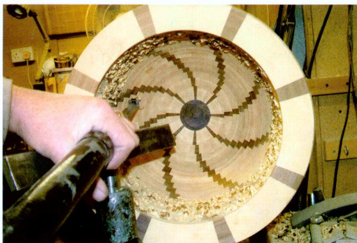
▲ Pic.13 Glue up about 19 rings, then turn and finish the inside
