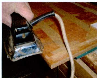
▲ Pic.24 Re-heat the glue to allow the removal of waste veneer
