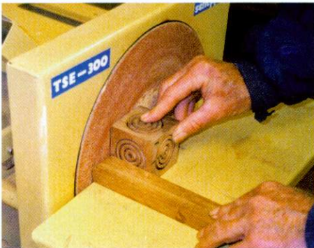
▲ Pic.4 Sanding the rings flush with the cube
