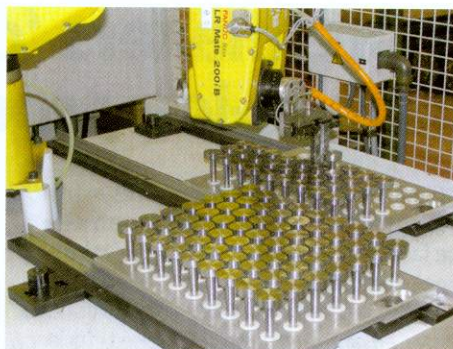
▲ Cutter blanks are automatically loaded into a machine to be ground before brazing
