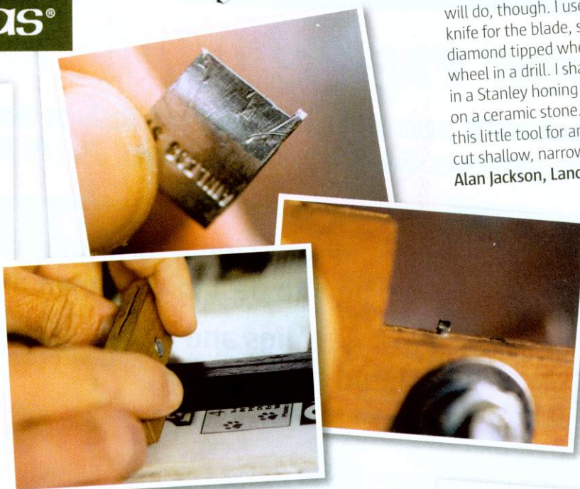
◀ Making the scratchstock using an old dinner knife as the blade
