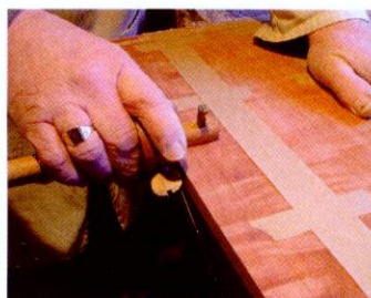
▲ Pic.21 Use a cutting gauge to cut the edge for the inlay and banding
