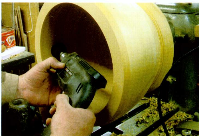
▲ Pic.15 A quick and efficient way of getting a good finish is to power-sand
