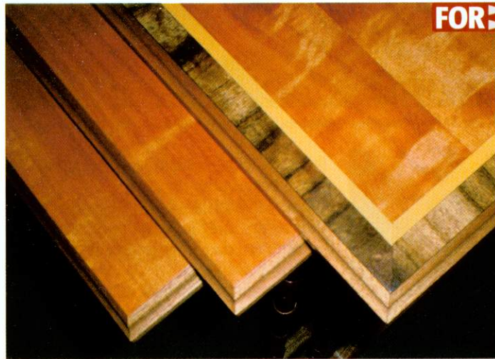
▲ Pic.20 Only the largest table has cross-banding and inlay
