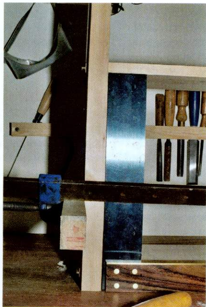
◀ Pic.4 Double-check the angles as you clamp because it's easy to push a large carcass out of shape
