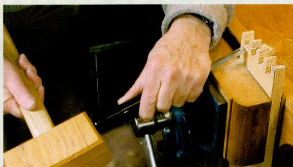
▲ Pic.6 Keep the workpiece low in the vice as you chisel
