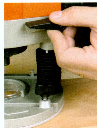
▲ A lever plunge is tricky to operate in some positions
