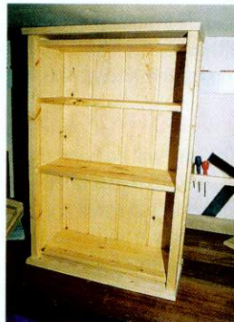
▼ Pic.5 An offcut of tongue and groove made the perfect back to the cabinet
