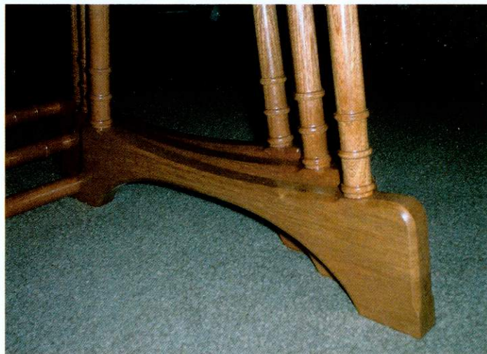
▲ Pic.15 Notice the stopped chamfers. These have to be routed accurately
