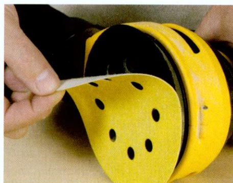
▲ The eight-hole plate takes standard hook-and-loop abrasives, meaning quick swaps
