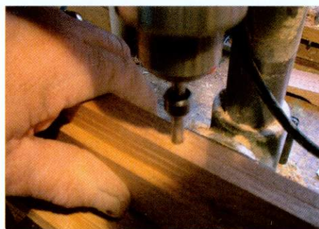
▲ Pic.13 Drilling the top rail for dowels to fix to the table top
