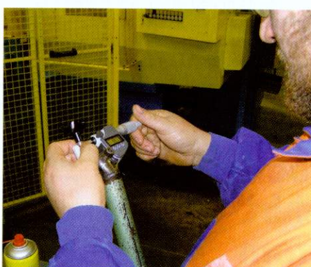
▲ One of many quality control checks that the cutters must undergo at the end of the process
