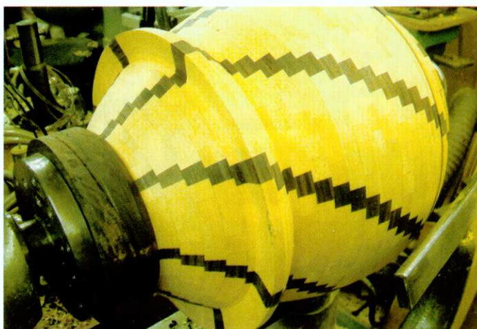
▲ Pic.16 I've left a couple of rings proud to help when I clamp the top on
