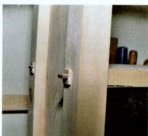
▲ Pic.6 The wedged joints are made with walnut to add a nice little detail to each one
