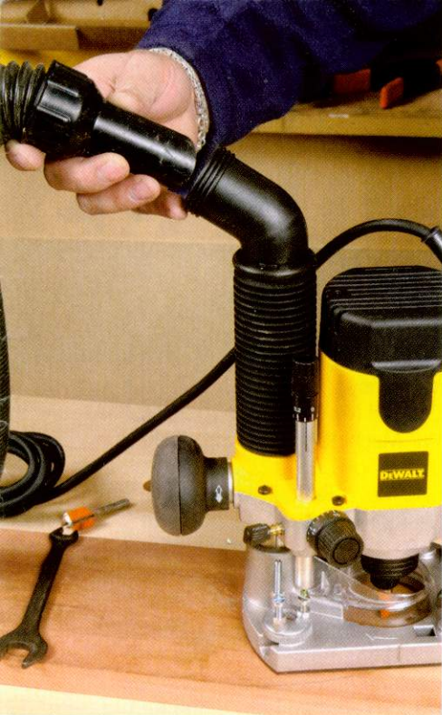
▲ Pulling waste up through the leg keeps the hose out of the way
