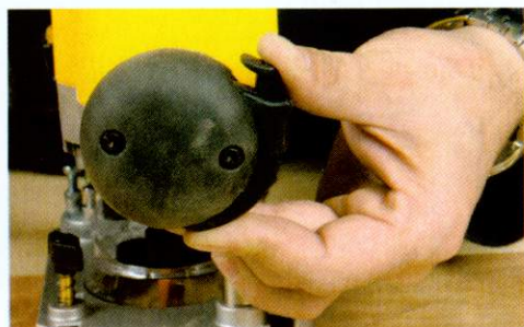
▲ The dual trigger locks in when necessary
