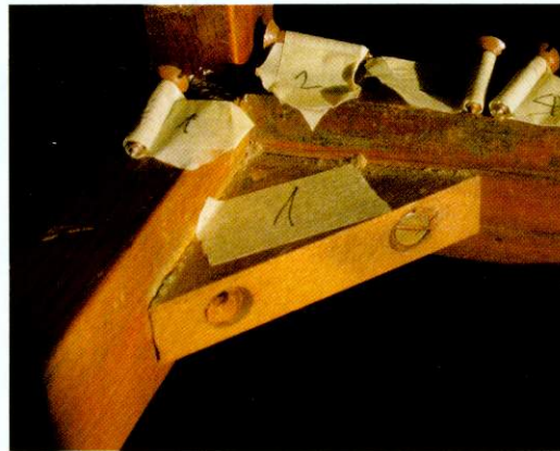
▲ Pic.1 Mark the screws with tape right after removal
