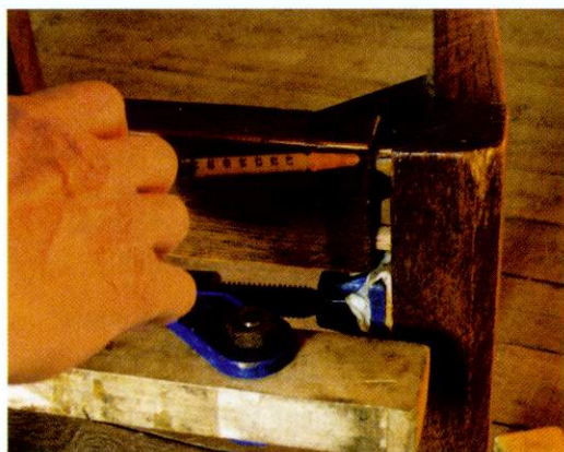
▲ Pic.3 Using a syringe to inject hot animal glue
