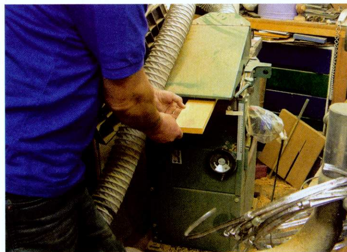
▲ Pic.4 My planer thicknesser came in very handy for making all the strips of pau amarello the same before I cut them up into small segments
