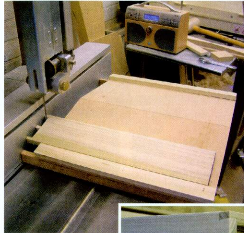
Pic.9 After this last cut, I notch the ends on the tablesaw like I did for the tails
