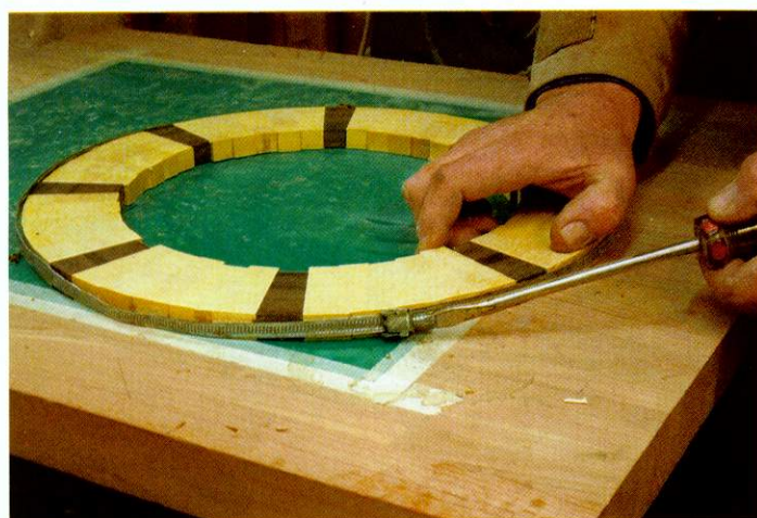
▲ Pic.7 Glue up the rings with PVA and clamp with a long jubilee clip
