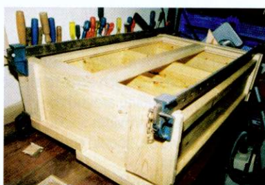
▲ Pic.7 Cramping on the base and lid. By this stage the carcass should be pretty secure, but still check the diagonals
