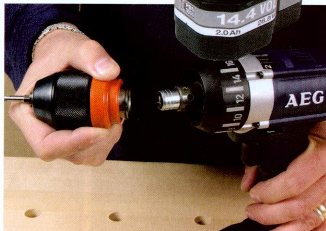
▲ The all-metal Rohm chuck has a quick-release system
