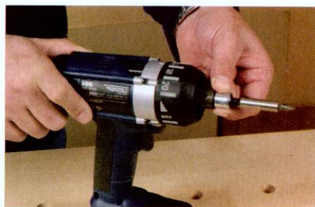
▲ The drill has a built-in hex shaft for screwdriver bits
