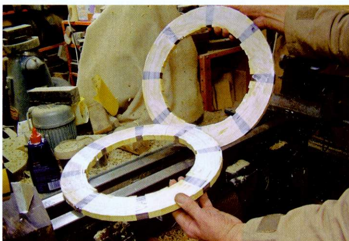
▲ Pic.9 Put the glue on both sides then clamp the rings together
