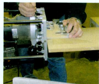
▲ Here the table is used as an oversized fence to push the router over the work
