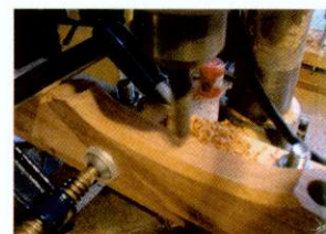
▲ Pic.12 Counter boring the top rail
