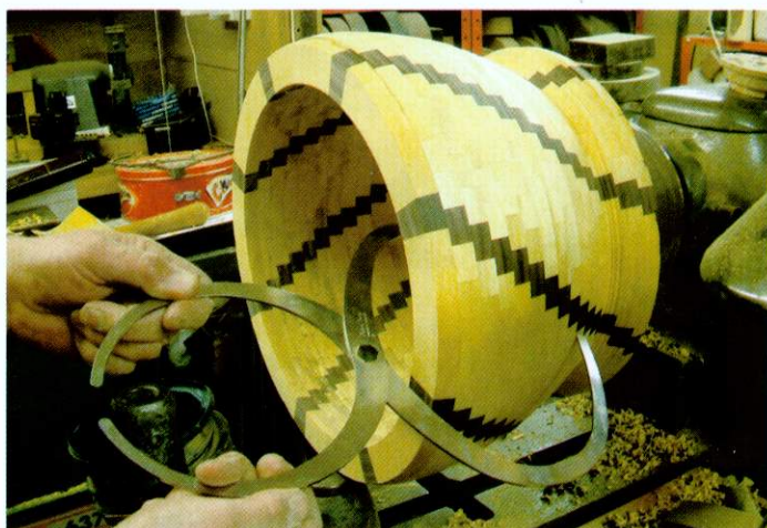
▲ Pic.14 Check the wall thickness with figure-of-eight callipers
