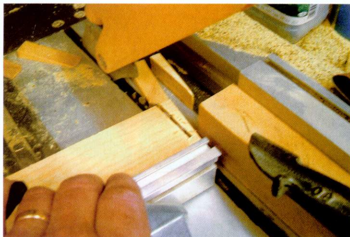
▲ Pic.5 Cutting the pieces: leave a gap for the segments to escape into
