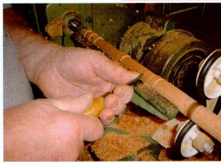
▲ Pic.7 Turning the legs using a steady to stop any vibration. You may have to use your hand
