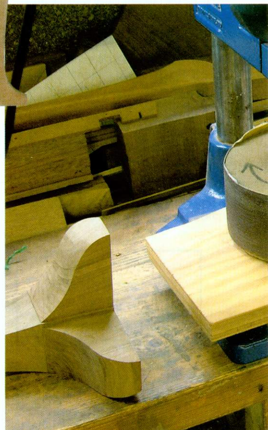
▲ Pic.6 Blend the cheeks in with the legs using a Make sure you always wear a dust mask or respirator
