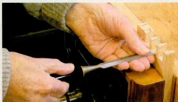
▲ Pic.9 A sideways shimmy may help the chisel to cut better
