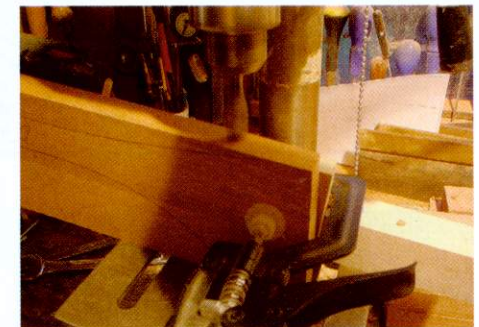
▲ Pic.9 It is easiest to drill the holes in the feet before shaping them
