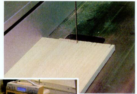
Pic.9 After this last cut, I notch the ends on the tablesaw like I did for the tails
