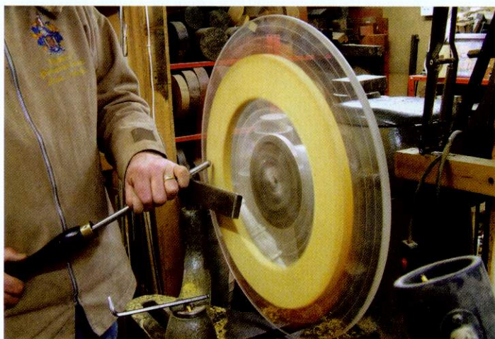
▲ Pic.8 Put each ring into a chuck and face up both sides
