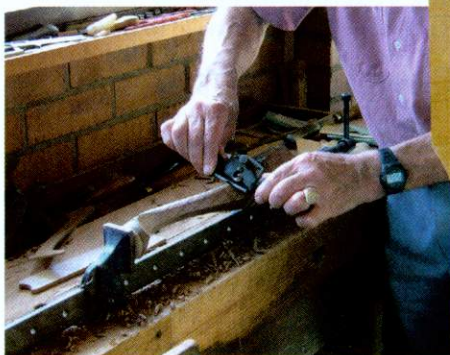
▲ Pic.2 Hold the cabriole leg in a sash cramp while you shape it with a spokeshave
