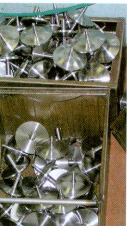
▲ The steel as it arrives: this is R48 stock, the same as Ferrari and Porsche use in their engines
