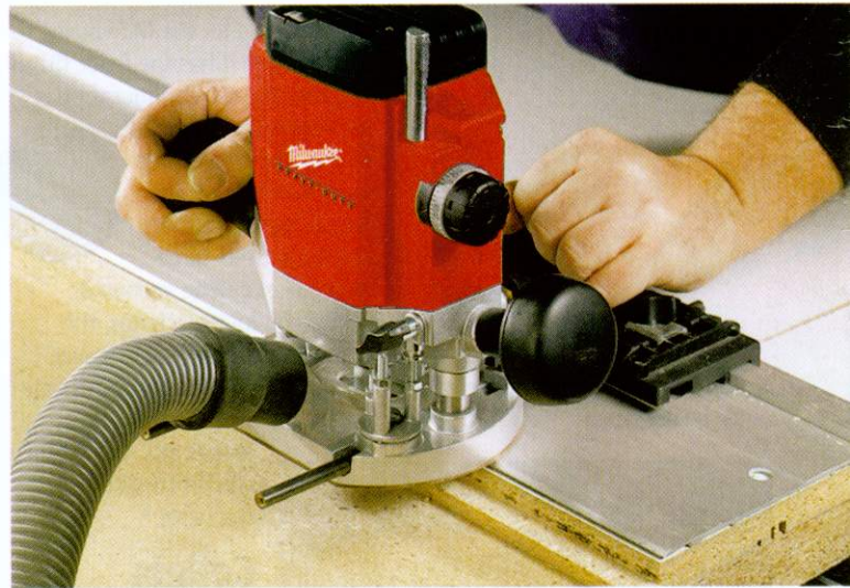
▲ Dust extraction low down can obscure vision and the hose can drag
