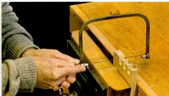
▲ Pic.5 Use a coping saw to within 2-3mm of the line
