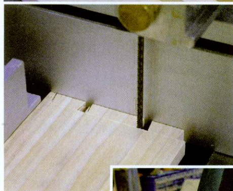
▲ Pic.4 (top) The ends are notched so that the bandsaw blade can enter between the tails Pic.5 (above) Use the bandsaw's own rip fence to bottom out the sockets
