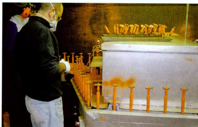
▲ The spraying booth, where the orange PTFE coating is applied
