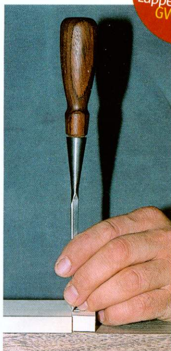
▲ Pic.5 Hold the chisel vertically as you start to chop
