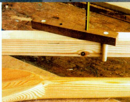
▲ A simple marking tool used in shaping oar blades, which are made from pine
