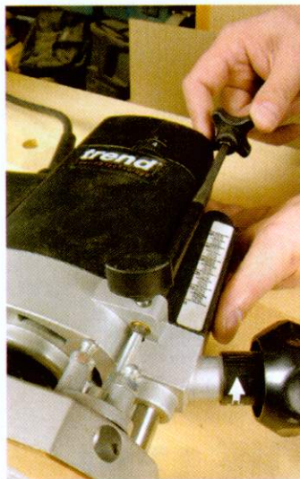
▲ With a fine adjuster like this, fast adjustment isn't easy on this Trend
