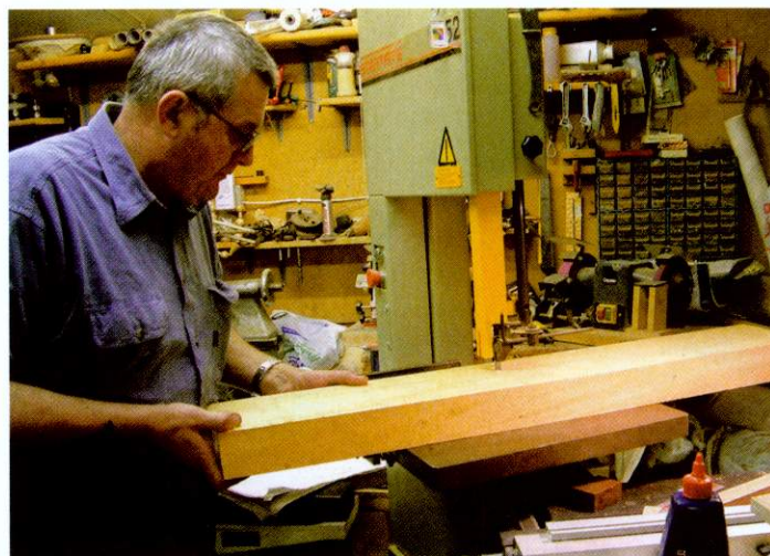
▲ Pic.2 Bandsawing the pau amarello into 22mm-thick strips ready to go through the planer thicknesser
