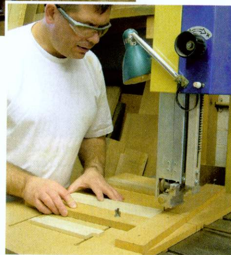
▲ Pic.3 The tails are cut first, then spacers are removed one by one, flipping the board to make the other dovetails
