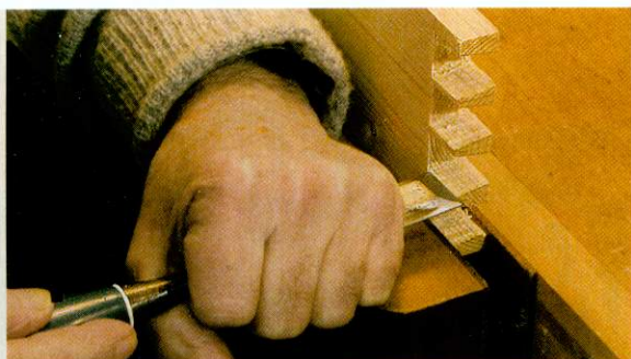
▲ Pic.4 Working horizontally across the grain to avoid splits
