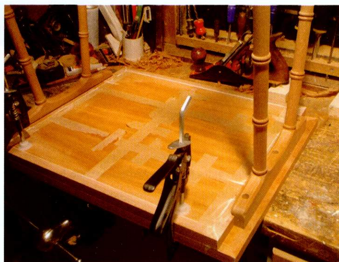
▲ Pic.27 Position one tabletop below its mate for fixing the top rail
