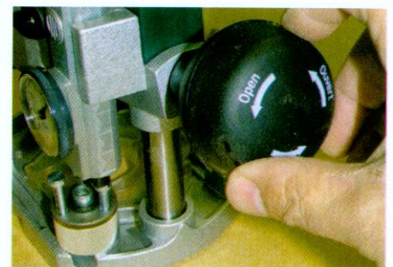
▲ Plunge locking handles are easy to control
