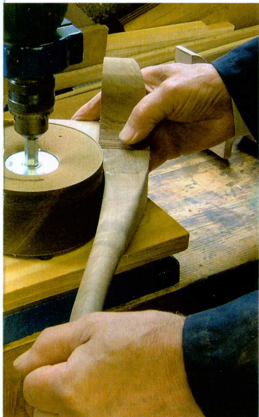
drum sander. This is a foam-filled drum, when doing this sort of sanding
