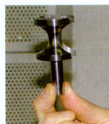
▲ A bit after brazing and ready to get its PTFE coating
