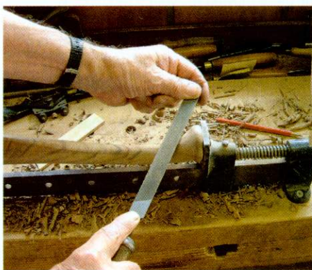
▲ Pic.3 Files and Microplanes are excellent for finishing the cabriole leg shape
