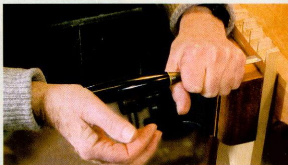
▲ Pic.7 A small thump helps as you start to level the land
