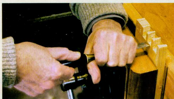
▲ Pic.8 Work towards the centre from each side
