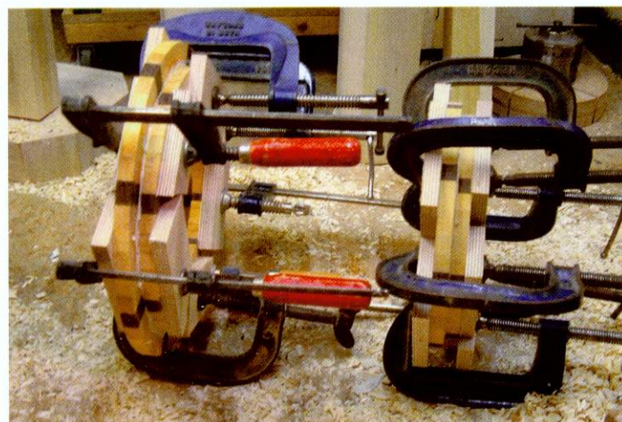
▲ Pic.10 Only clamp two rings at a time and don't forget the bits of ply
