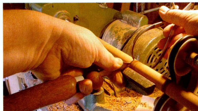
▲ Pic.10 Keep checking the diameters of the legs. Consistency is important
