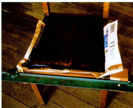
▲ Pic.4 Cork and paper padding helps avoid damage
