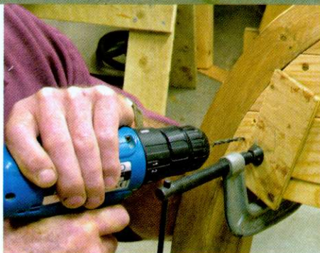
▲ Drilling into a larch plank to put a brass screw in the rebate of a partly repaired boat's oak stem
