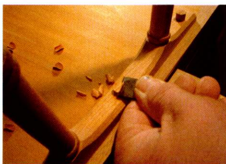
▲ Pic.27 Chisel back the plugs. Notice how Bill is working across the grain to reduce tearing
