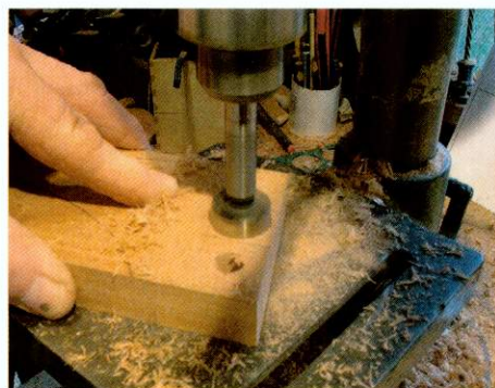
▲ Pic.11 If you drill 25mm diameter holes first, cutting the notches in the feet is much easier
