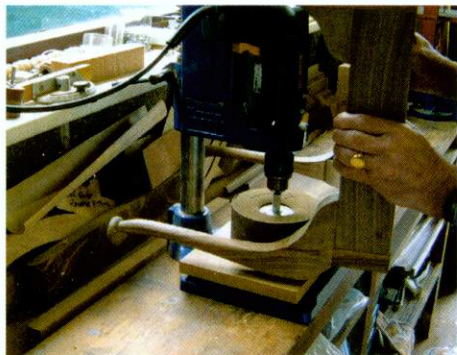
▲ Pic.8 Sand the inside of the legs with a drum sander. A drillstand will do for this job
