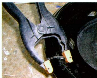
04 The wood inserted in the crack and cramped up with a soft-jawed spring clamp to exert pressure either side
