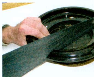
01 Time to be brave! Cutting the crack in the bowl with a panel saw to produce a slot
