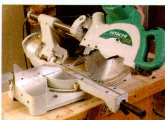
...or to the right. The upper part of the fence is removed first
