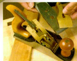
The lever cap of this Bedrock pattern plane is bronze
