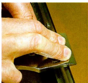
Lap the underside front edge of the lever cap so that it clamps down on to the cap iron correctly
