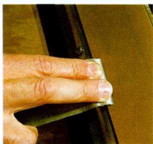
Hone the back of the cap iron to ensure a good fit with the blade
