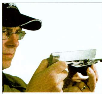
03 Check that the frog is acceptably flat. An engineers square is the ideal tool for doing this
