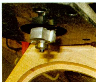
05 Smooth the edges then rout a rebate with the aid of a bearing guided rebate cutter
