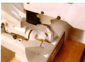
A neat splitter device stops thin offcut slivers being thrown about
