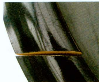
02 The slot is now parallel sided and ready to be filled with a sliver of matching wood
