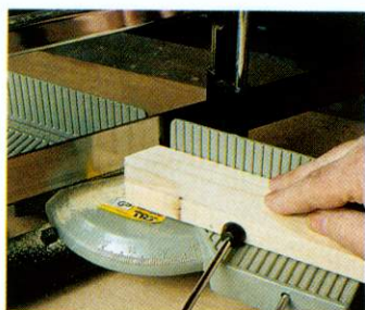
05 A hand mitre saw like this is very useful for small projects and cuts clean mitres
