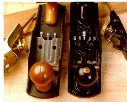
Lie-Nielsen use a Bedrock frog (left), while the budget and mid-range planes are Bailey pattern
