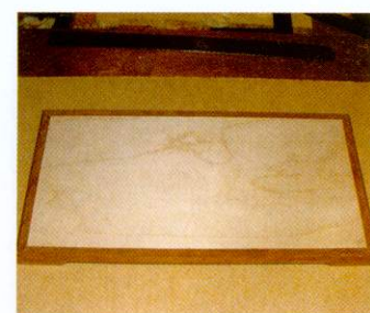
08 The bottom sits in a rebate routed in the top edge of the base. This is slightly deeper than the ply's thickness
