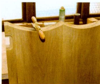
11 With all jointing finished you can now start shaping the seat with spokeshaves and sanders
