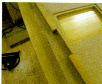
14 Lip the assembled table top with hardwood then cut a recess for the handle on the mounting rod assembly
