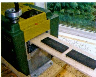
03 Passing sections of African blackwood mounted on a backing board through the Proxxon thicknesser.
