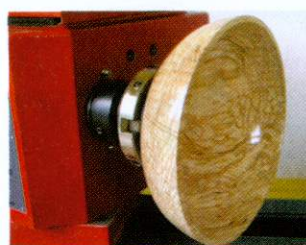
The marbled beech bowl on the lathe after polishing
