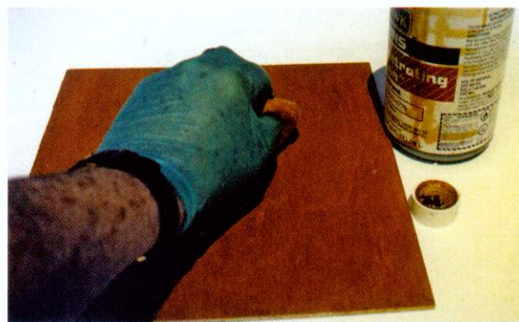
Dye stain being wiped over a panel that has been solvent soaked
