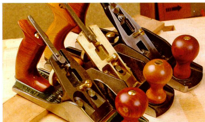
Clifton, Lie-Nielsen and Veritas planes with cap irons and blades removed. The Veritas combines a traditional lateral lever with some innovative features
