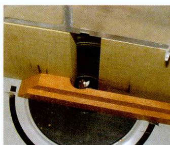
06 Bandsaw the waste between the two holes then rout to a clean finish on an inverted router with a straight cutter
