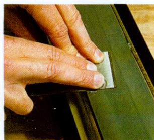
Work the back of the blade (cutting iron) flat before honing
