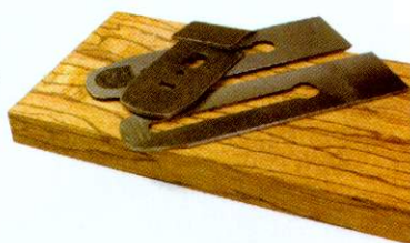
The Clifton two-piece cap iron reduces cutter chatter when planing and speeds up honing. In front is a Japanese blade, with a Victor iron behind
