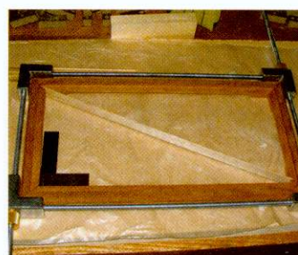
07 Frame cramps such as this from Axminster are the perfect way to clamp up small mitred sections for boxes
