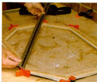
05 A strap cramp will pull the octagonal frame together but check matching diagonals are equal to ensure square
