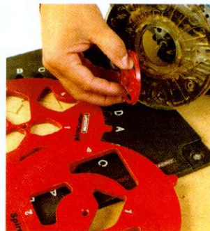
Four guidebushes are provided, enabling you to make patterns like this quite easily
