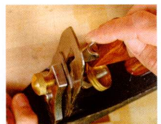
The lever cap is folded pressed steel and a bit flimsy
