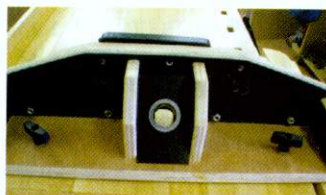
Coachbolts locate the fence in the T slots in the table. Note the dust port
