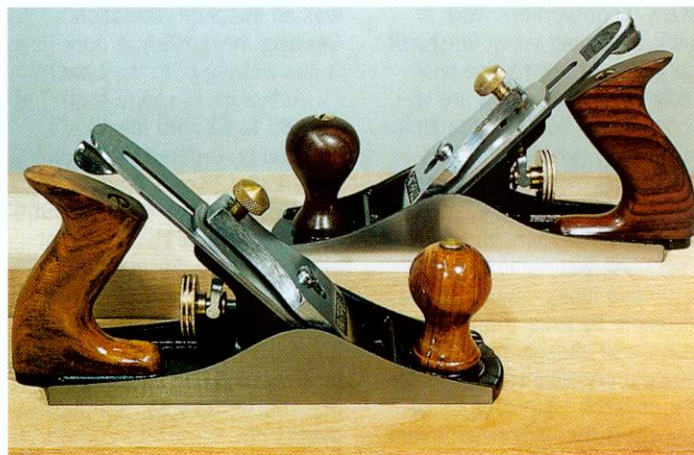
The Faithfull plane fitted with a replacement Japanese laminated blade. Behind is a fully tuned smoothing plane (right)
