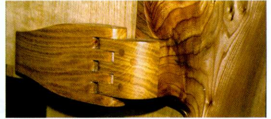
David Lilley retained the natural edge of the English elm door for this unique wall cabinet. Inner carcass, shelves and hinges are from oak, while the finish is Danish oil
