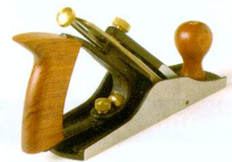
A Norris-style depth rod doubles as the blade lateral adjuster
