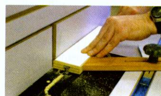
Routing a T slot in a fence section with a key hole cutter
