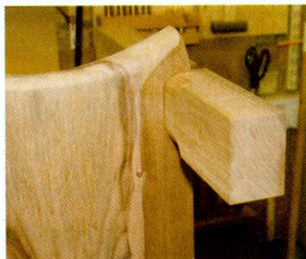
14 The front legs are jointed while in the square then the shape refined both before and after assembly
