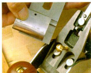
A two-piece cap iron reduces chatter and makes honing faster
