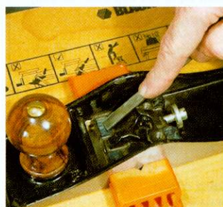
05 Clamp the body in a Workmate and use a homemade scraper to get the seatings flat
