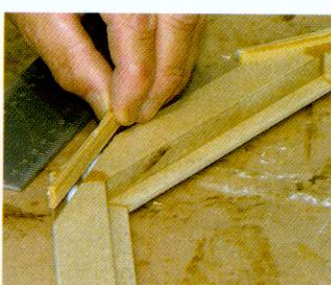
07 ...then planing a thin strip of timber to fit and gluing in place. Trim the ends when dry and plane flush
