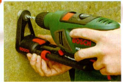
Not only does it collect dust efficiently, but the box ensures you drill squarely
