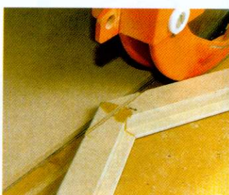
06 The fragile glued mitre joints are reinforced by first making a saw cut across the joint with a radial arm saw...
