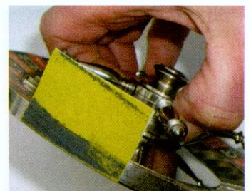
06 J-flex abrasive stuck to the side of the rim with double sided tape is rotated with the spinner to act as a sanding drum
