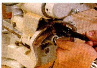
You lock the mitre angle via a solid Bristol lever at the back
