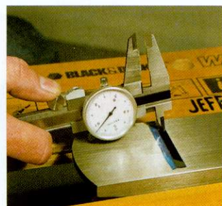
06 When widening the mouth, use vernier calipers to gauge that the opposite edges remain parallel
