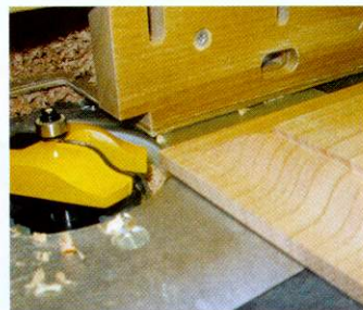
07 It's best to finish the panels before you assemble the frame in case they shrink insitu
