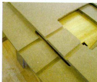
13 Rout matching grooves in the two pieces that make up the top to form the holes that take the mounting rods
