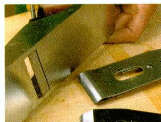
The frog forms part of the mouth, and can be reduced for finer cuts
