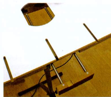
The bars slide through two recesses routed in the table before assembly
