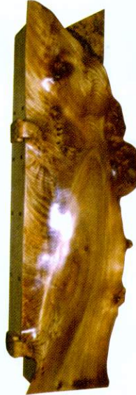
David Lilley retained the natural edge of the English elm door for this unique wall cabinet. Inner carcass, shelves and hinges are from oak, while the finish is Danish oil
