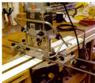
Simple jigs like this can help with accuracy when routing mortices
