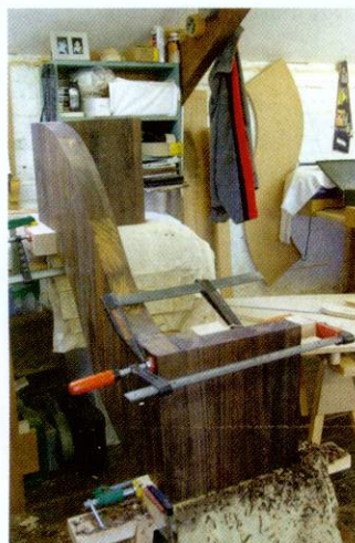
The 45° chamfer twists around its axis as it follows the curve of the top
