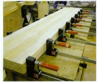
08 Use biscuits to reinforce and align the other sections for the main top assembly. Glue up and trim to length
