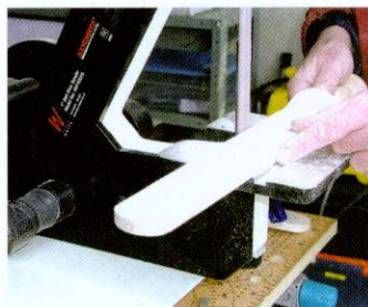
06 Form smooth convex surfaces and rounded edges on the blade with the belt sander. Avoid the belt digging in
