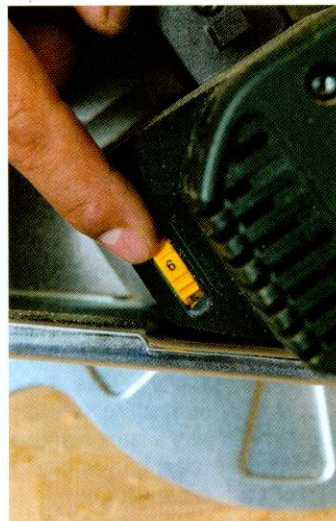
The inclusion of variable speed is an innovation. A dial is on the housing
