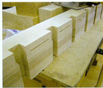
06 These two sections are then biscuitted together for strength and to align the top edges perfectly
