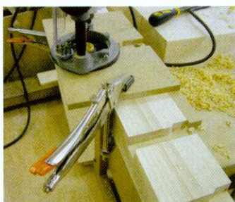
05 Use your template to rout the dog holes in the rear half of the two dog bench pieces
