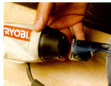
The small fabric dustbag simply pushes on to the extraction port
