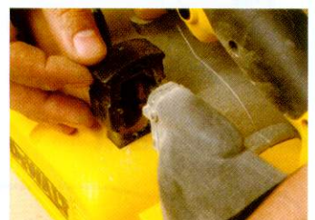
Dustbag is well supported but you need an adaptor for an extractor
