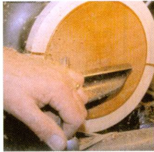
06 Use a glue chuck to hold the base while you work on the edges, then fit to the cylinder...
