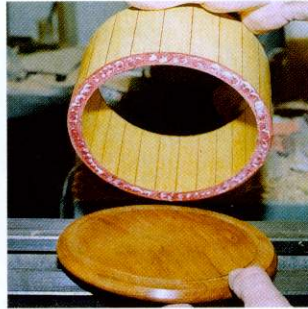
07 ... and form a slight rebate before finishing off held in the MDF jaws to flatten the surfaces
