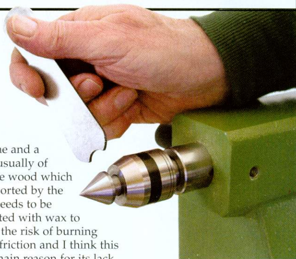
Sorby hollow revolving centre with the tool which is used to remove the interchangeable heads
