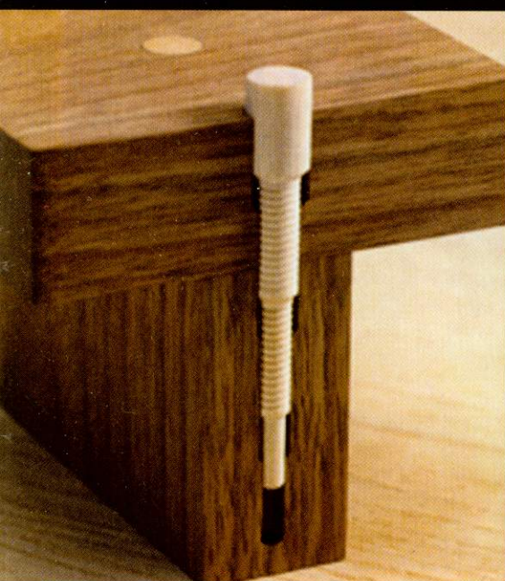
1. Drill stepped pilot hole with TruFit drill bit.
