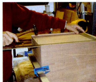
15 The back board is cut narrower to allow the bottom panel to be slid into its grooves from the rear
