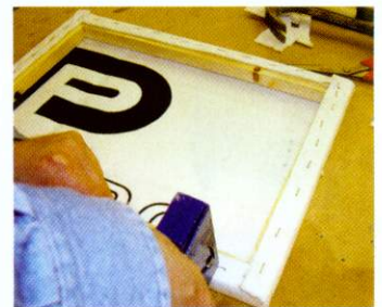
12 Staple a needlefelt filter fabric over the frames as shown. Make sure you allowed for this when making the frames
