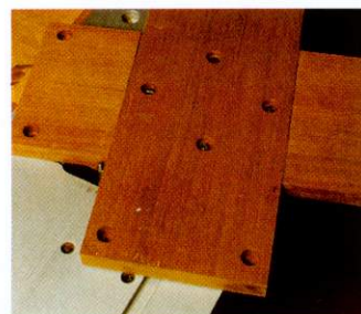
05 Drill both halves for fixing screws for the uprights. The central ones will be hidden by the bottom of the joint
