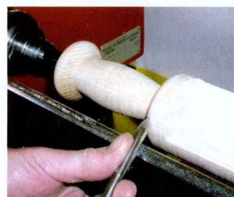
03 Shape the handle to a diameter to suit a small child's grip. Shape the blade's end virtually up to the centre point
