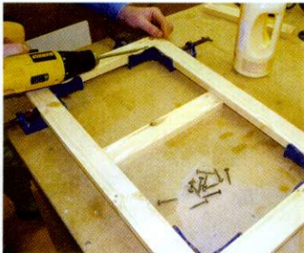
06 Assemble the frames and screw together. Note that the two internal battens are central here
