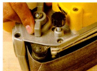
The turnbuckle lever lock on the belt drive is easy to operate
