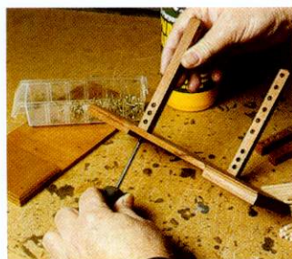
06 Begin assembly by fitting the centre uprights to the top part of the base, then assemble the half lap
