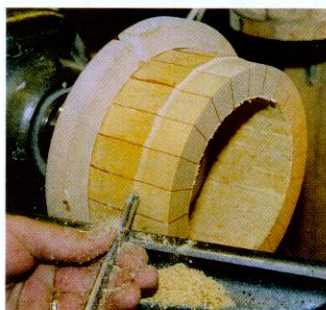
01 Face up the top edge then shape half the side, inside and out, then flip and repeat for the other edge
