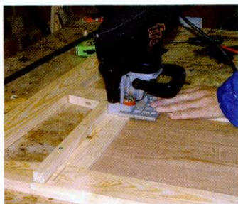
05 The bottom panel sits on a support and is also biscuited to the side frames. Index the jointer off the batten...
