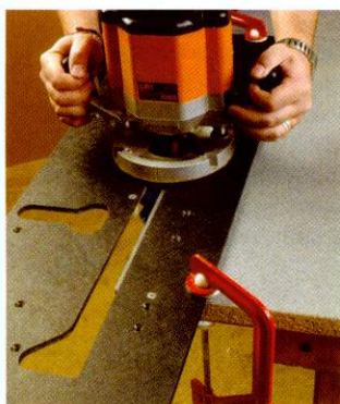
We detailed how to cut worktop joints with a jig in GW 148
