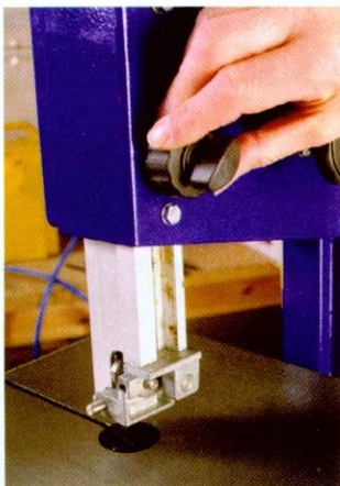
Rise and fall of the upper guard is operated with a rear knob
