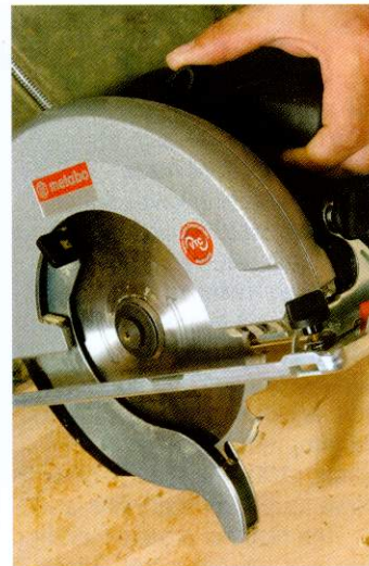
A red cursor on the front of the steel base is adjustable to suit the kerf
