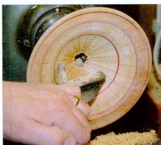
13 Leave a slight lip on the outer edge of the lid to fit over the outside of the bottom of the box
