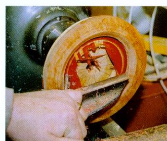
12 You turn through the veneer section as you start to shape the inside of the lid
