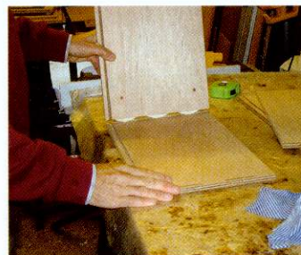
14 Drawer carcasses are biscuitted plywood. Make sure the sides overlap the back and front for strength
