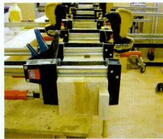
07 Make sure that the end face of the assembly is perfectly square and aligned, apart from the dovetail
