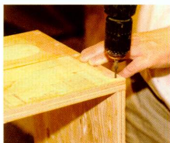
06 Plasterboard screws are perfect for screwing ply as they do not split the veneers and the hold is excellent
