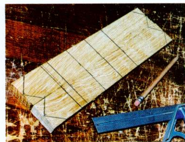
01 Mark out both sets of legs as one pair to ensure the joints and shelves match up on each
