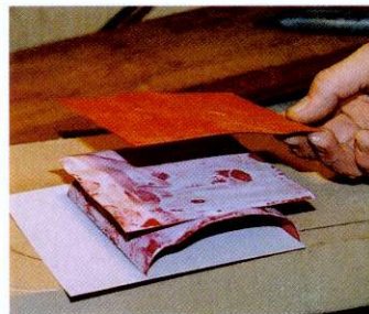
07 Make up a piece of ply for the upper ring in the lid by sandwiching together three pieces of red veneer
