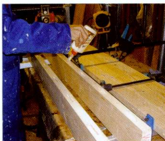
13 The top is made up from a series of narrower boards biscuitted and glued. Plane smooth and cut to length
