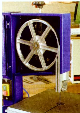
As the machine is so small the tension knob is easy to reach
