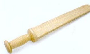
07 Paint the handles but varnish or oil the blade. Blade edges will need re-sanding from time to time to remove any splinters
