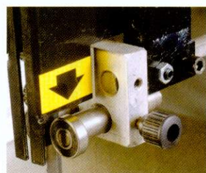
Upper side rollers are eccentric on the ESY machine, and easy to adjust with a hex key. Beneath the table brass rods are used instead. Both rear thrust wheels are locked with knobs
