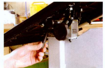
Bristol lever and tilt knobs are soft-grip and easy to reach
