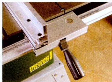
The fence has a hairline magnifier, though the metric/imperial scale was 4mm out...
