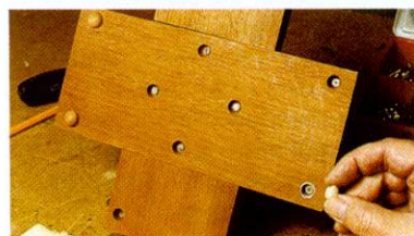
Hide all the screw heads by counterboring the holes for Plug It domes
