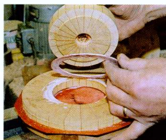
11 while accommodating the veneer ring. Glue up the assembly and clamp, making sure the lines match up
