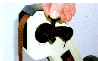
The tracking and self tensioning device is very effective
