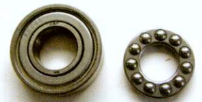
A thrust race (left). Good quality revolving centres have a radial ball-race to take the axial load (right)
