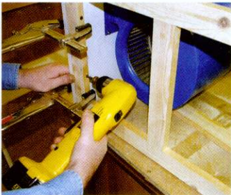
07 These two frames are screwed directly to the front panel containing the fan, with the edges flush
