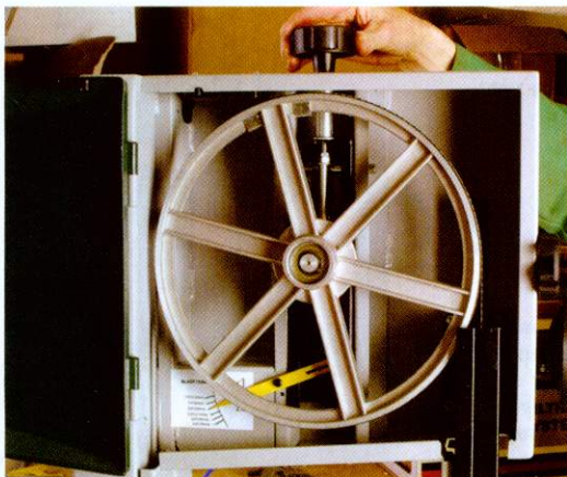
A steel pointer behind the bandwheel indicates the correct blade tension for a range of sizes
