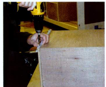
16 Standard metal drawer runners require 12mm clearance between carcass and drawer each side
