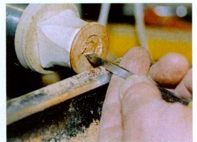
16 Now turn a small collar to fit the spigot on the finial support. A glue chuck is useful here, mounted on a screwchuck
