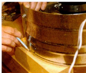
09 The fan is held in place with blocks, mark the radius directly from the fan housing
