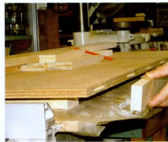
07 The front edge of the bottom panel will also need biscuiting to attach a front rail cut to the same length
