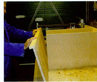
08 Carcase assembly starts by adding the top frame and bottom panel to the two vertical MDF drawer dividers...
