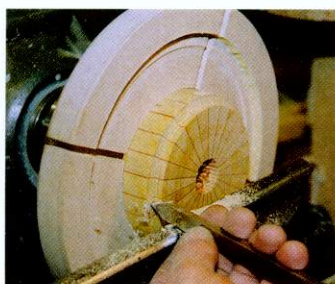
10 Face up the upper lid section then turn a small spigot to locate into the lower lid section...
