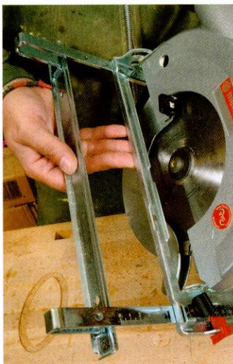
The longer fence on this saw makes it more accurate for ripping cuts
