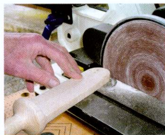
05 Sand off the waste (and marks from the centres) at the top of the handle and the blade end on the disc sander
