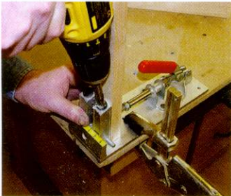
05 Two side carcass frames are jointed with a pocket hole joiner. You could mortice and tenon these or butt screw
