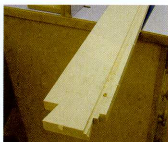
11 The rear rail is grooved to take the tool well bottom ply and dovetailed to fit the breadboard ends
