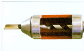
The Apollo revolving ring centre for long hole boring has a large area cut out to allow shavings to escape
