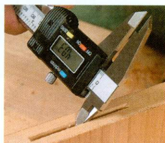
A handy tool for accurately measuring slot widths and mortices
