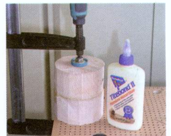
08 Gluing and cramping up 2 blanks for the finial. Titebond II is strong and waterproof. Cramp up for at least one hour
