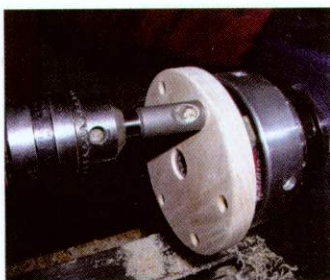
05 The Planet 'snail' countersink has a hole in the side which allows the shavings to escape
