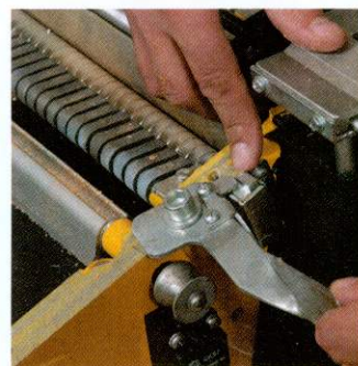
The dust hood or table must be in place for the micro-switch to work
