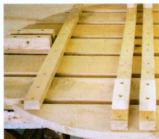
07 Support battens on the underside hold the top together and also locate over the legs
