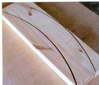
05 The middle rail is cut from a wider block too. Again, mark out for the slats and central muntin before cutting
