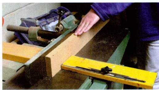
4. Close up the guard to leave no gap. Keep firm pressure down on the table and into the fence at all times
