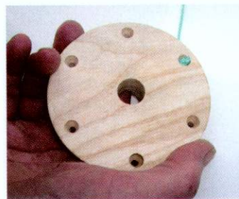
06 Countersink both sides. The holes on the top should be deep enough for the knots or the finial will not be flush
