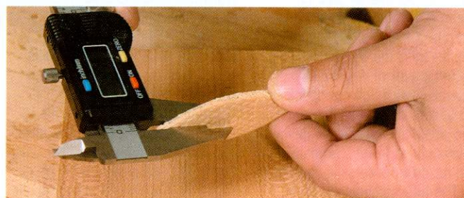
You'll find biscuits are not always a consistent thickness... A digital readout is far easier to read than a traditional scale
