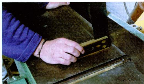
1. Check the fence is square to the surfacing tables. Make sure your square is accurate, though
