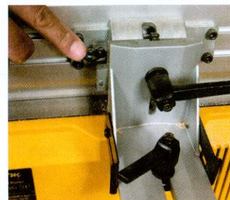
A flipstop on the back of the fence enables it to tilt either way (above)
