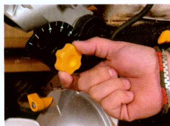
A protractor scale means you can quickly set blade depth for trenching
