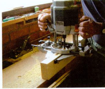
07 A pair of fences will centre your router on the timber as you rout with no fear of it drifting
