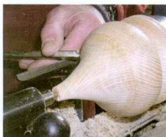
09 Turning the finial to shape. Tailstock support is given with a Planet Slimline revolving centre
