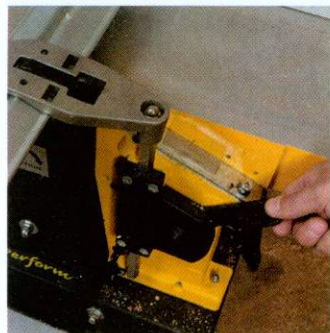
You adjust the bridge guard with a rack and pinion-action lever
