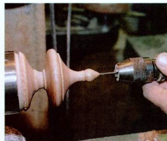
07 Before parting off, drill a 3mm hole through the centre with a bit mounted in a Jacobs chuck
