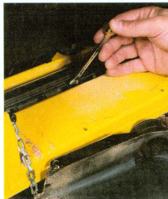
Access to the cutterblock is good. The cover attached to a chain
