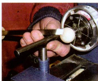
10 Turn the decorative ball for the top of the finial. The Selbix toolrest allows turners to work close to small scale work
