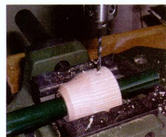
12 Drilling through the top collar into the pole so that a woodscrew can be used to secure the collar
