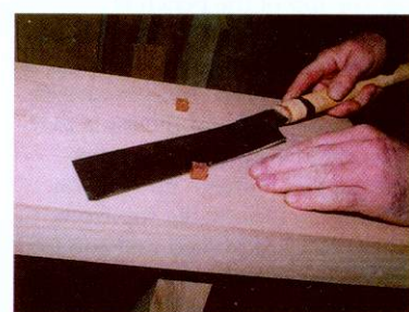
09 Use a Japanese pullsaw to remove as much of the excess mahogany as possible, without scoring the bench top
