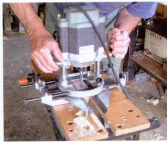
06 The mortises for the loose tongues are routed. A spiral cutter with an up-cut is the most useful for this depth
