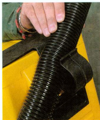
The flexible hose can be clipped out of the way of timber being machined
