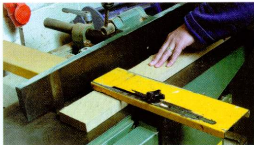
2. Plane the concave face first, working with the grain to avoid tearout. Start with both hands behind the guard
