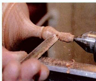
06 Turn the clanger to shape on a screwchuck, using the tailstock for support. A 9mm gouge will suffice
