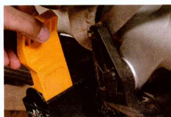
The compound angle locking lever faces forward, so access is good
