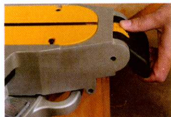
The front paddle lever enables you to use a thumbwheel for indexed angles
