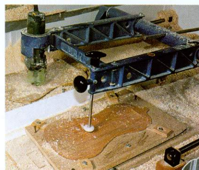
This American Marlin copy router enables a violin front or back to be initially shaped
