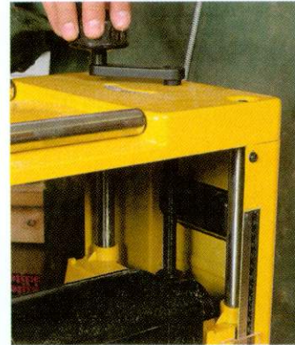
The winding mechanism has twin threaded rods, plus four corner posts
