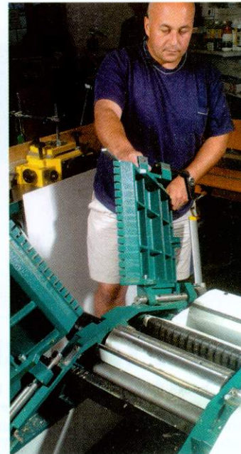
On Rojek's MSP 310M planer thicknesser (tested in GW 140) there's a choice of fixed or flip-up tables
