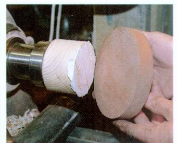
08 Use a glue chuck to hold the flat blank for the top disc while you face up the underside of this
