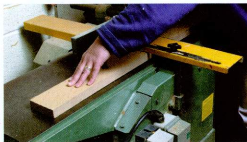
3. Transfer left hand to the front to keep wood firmly down on the outfeed. Don't pass hands over the cutters
