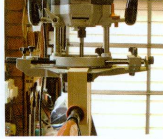
08 You'll need to cramp extra support for the router base onto the timbers as you rout the ends of these
