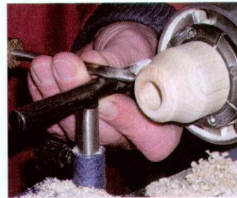
07 Turning the collar to shape with a 9mm spindle gouge. This was drilled out first in the centre to fit the pole
