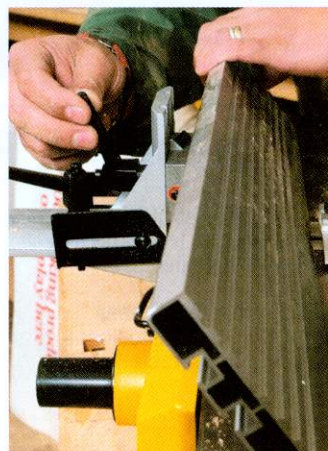
A flipstop on the back of the fence enables it to tilt either way (above)
