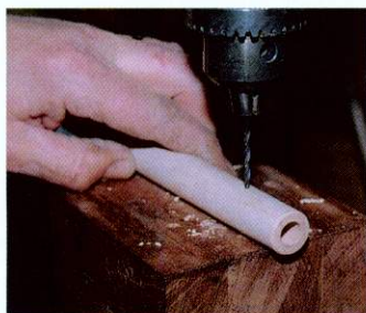
05 Drill a small hole near the top of each tube for the fixing cord. This should go through both sides
