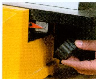
Depth of cut is easy to set with a knob below the infeed table (above)
