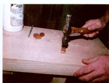
08 Glue and fit the mahogany pieces into the squares and then lightly hammer them into place
