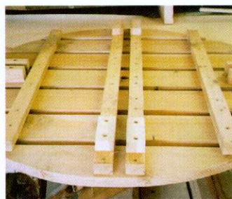
06 The circular top is made from 7 lengths of 150x32mm, cut to shape with a jigsaw and then cleaned up
