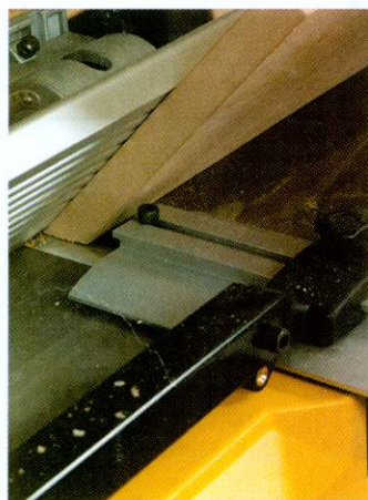
Depth of cut is easy to set with a knob below the infeed table (above)
