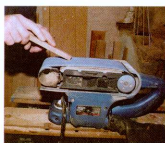
07 Prepare a length of square cross section mahogany to the same size as the hole, with the edges bevelled to fit
