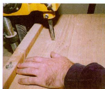
05 To fix the legs to the benchtop, first cut a small square hole in the top with a morticer to accept a covering plug
