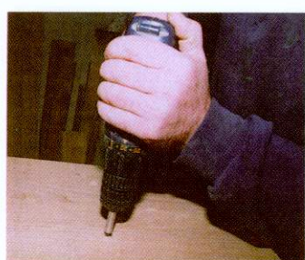
06 Drill a central screw hole in each of the mortices for the main fixing screws
