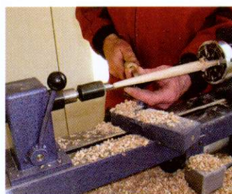
11 Turn the taper for a peg. The blank is held with the jaws in compression and supported with a revolving centre
