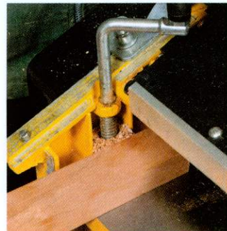
A cranked handle is used to adjust the thicknessing depth
