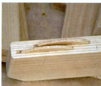
10 The slats are joined with a single biscuit but the main frame has two parallel biscuits for more strength
