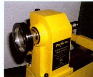
Remove the protruding grub screws on the flywheel and file the bottoms
