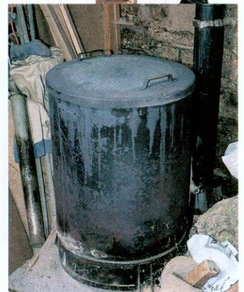
This Fulgora stove runs on timber waste and keeps the workshop at a reasonable temperature
