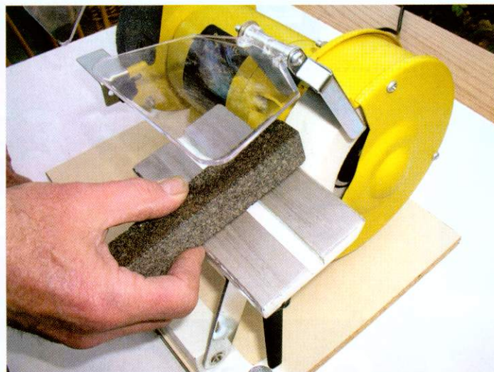
Dressing the white wheel on the Perform lathe with a devil stone
