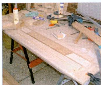
09 The side and front seat rails are made up from a sandwich of oak and ash boards edge jointed together
