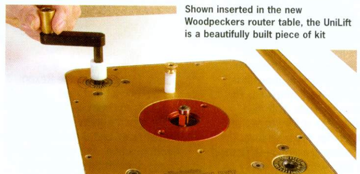
The reducer rings lock in place and are released with the tool provided
