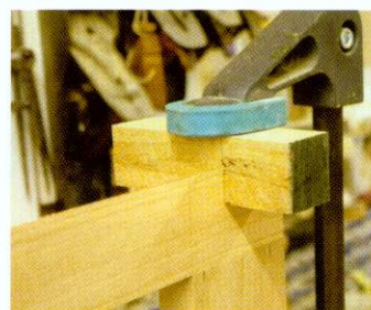
07 The bevelled stile edges made it awkward to glue up. Consider bevelling the frame after assembly
