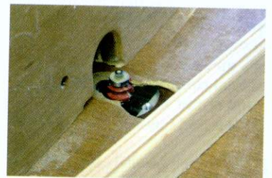
Cut the beadings by moulding the edge as shown then cutting to thickness/width
