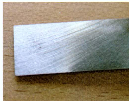
Top: Striations on a chisel back from the coarse stone. These will go as you polish
