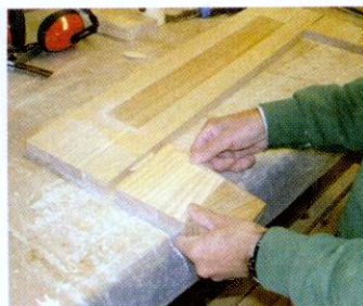
10 The front leg sections are butt-jointed on in a similar manner to form the complete leg rail section
