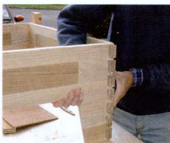
06 Through dovetails joint the front and side seat rails. Cut these by hand or use a dovetail jig. James used a Trend jig
