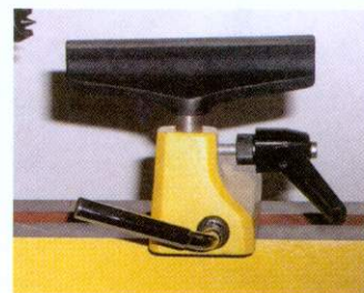
The toolrest tilts to the left. It should be in line with the axis of the lathe
