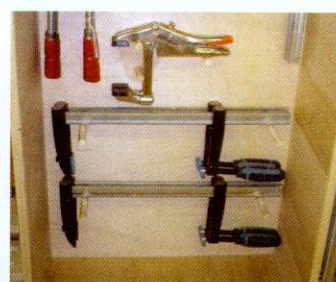
16 Drill holes for dowels around the centre board to take your other cramps. Cut the dowels to suit
