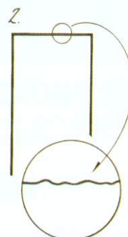
Left: Magnified coarse ground surface
