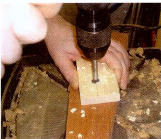
10 Make the supports by drilling out the centre then bandsawing to create slots for the cramps
