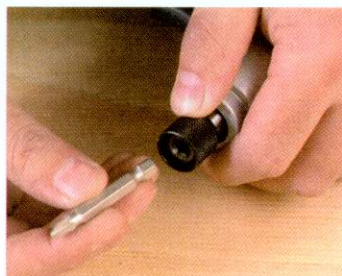
A knurled sleeve on the chuck is pulled forward to release the grip on the bit
