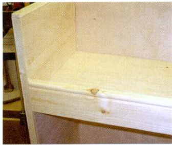
12 Plant a front onto the shelf to help retain all the clutter of screws and glues that will store here
