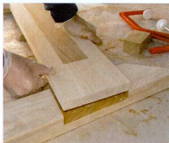
05 Check the fit of the rail. The end of this will be angled to sit flush with the leg's rear edge
