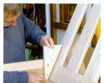
12 A spacer piece screwed and glued to the side rails and backrest will then support the rear arm rest cradle
