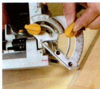
The twin fence can be adjusted for locating over acute mitred edges
