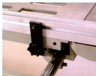
The crosscut fence locks with two knobs and can be removed easily
