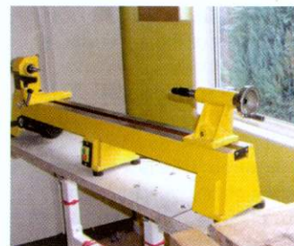
Fitting the extension bed is simple and gives a good long lathe
