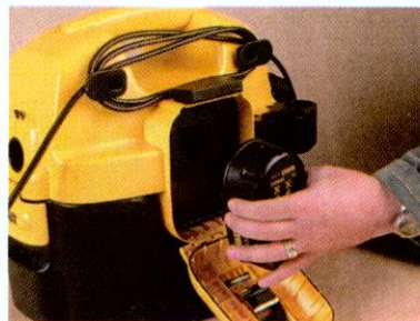
You release a latch to open the battery compartment cover. The battery slots in
