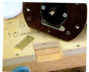
12 Hinge jigs are worth the trouble to make if you use the same size hinges regularly and allow accurate work
