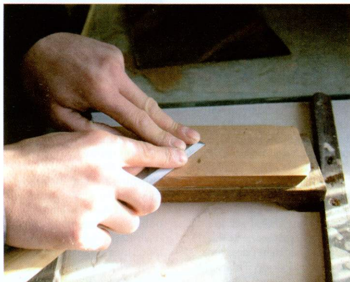
Left: Working the chisel back on a polishing stone
