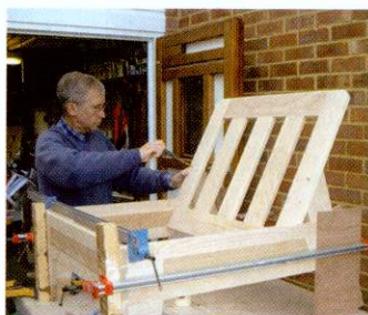
11 The assembled frame notches over the side rails and is then screwed to the back legs
