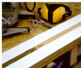
06 The finished mortises. You could cut the mortises in the rail ends for the loose tenons in the same manner
