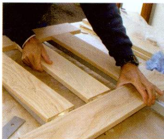
09 The backrest consists of a frame and slats biscuit joined together. You could use mortice and tenons if you prefer
