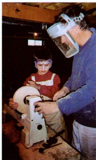
The small size of my Jet lathe meant that the top was 10in in diameter, the largest that can be swung over the bed
