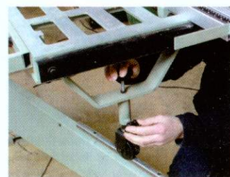
A jockey wheel below the sliding table runs on the outrigger
