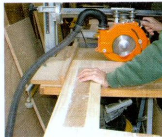
11 Crosscut the finished panels square and to exact length ready for dovetailing the front leg joints
