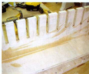
14 Glue the comp to a back support and add a pair of triangular braces into the joints
