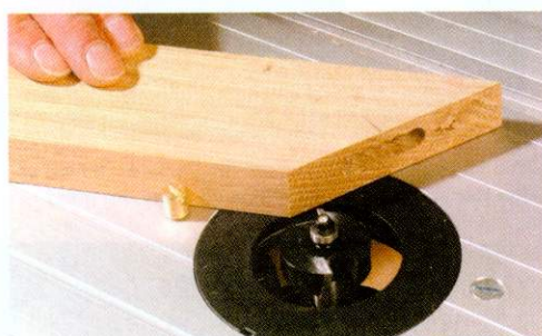
The Trend table is the only one with a lead-in pin. This is handy for routing with bearing-guided cutters
