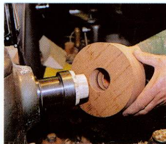
06 You'll need a jam chuck to support the collar. Drill a hole to match the column spigot then a chuck to suit.
