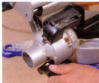
The protractor scale on the saw's tilt facility is large and easy to read
