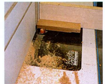
08 Rout a groove the length of the cursor block to clear the tape then rout the ends to accept the perspex plates
