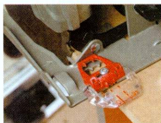
A hinged cursor can be adjusted to follow the left or right side of the cut
