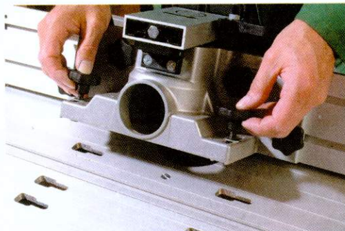
Slots enable the fence assembly to be fitted in three positions. The centre table extrusion can be removed
