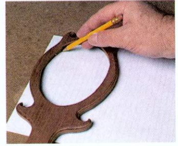
08 Mark out for the mirror retaining plate with a pencil before completing the finishing
