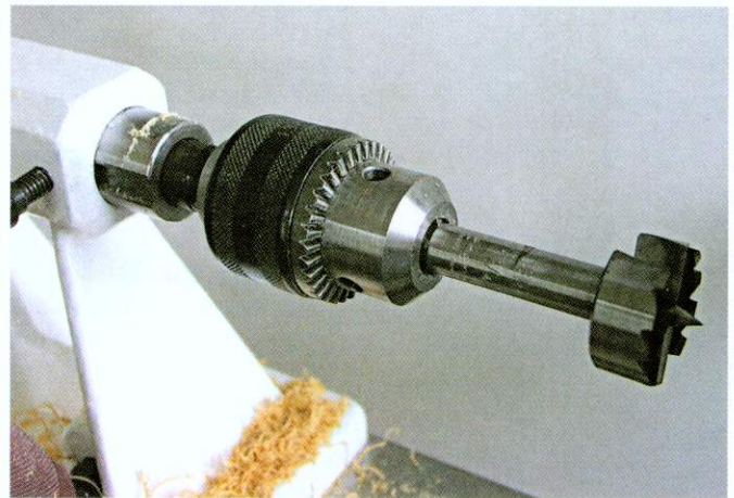
A short-shanked Trend bit mounted in the tailstock. These short shanks are particularly useful where distance between centres is limited
