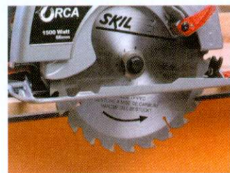
The biggest potential drawback to the Orca is its lack of a riving knife
