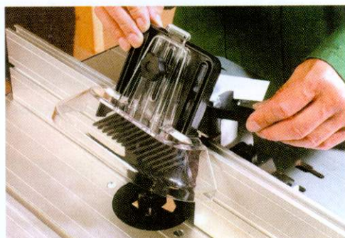
You tilt back the clear plastic guard and hold-down for cutter access. A lever locks it in the closed position
