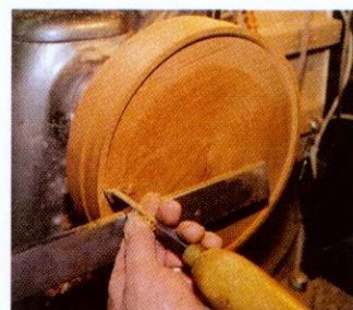
08 Face the underside of the top then mount on a jam chuck. Rough out the rim with a parting tool
