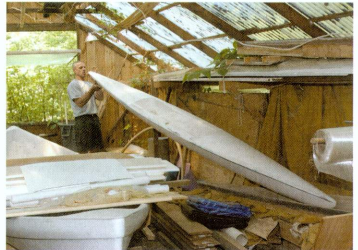
One of the part complete boats that adorn the floor in the workshop. A small rowing skiff, it has yet to be outfitted with sliding seat and oarlocks. The larger boat is a whaler type that is being built for recreational rowing
