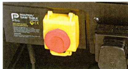
The switch can be padlocked off, but the mounting panel is rather flimsy
