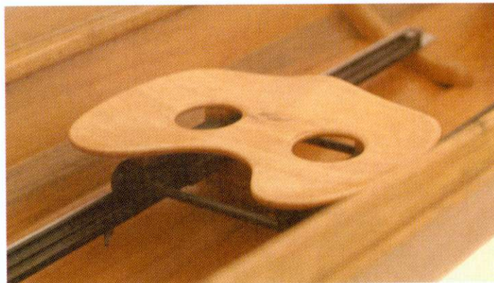
Some years ago John built a small rowing skiff for his son. I was unable to get a picture of the boat in its entirety but was stuck by this detail of the sliding seat. Lightweight yet functional it is good study in laminated construction
