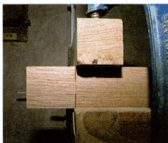
05 When cutting tenon shoulders by hand I often cramp a timber to the line to act as a guide for the saw
