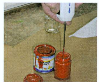
16 A small, battery operated mixer makes mixing the paint properly for airbrushing an easy task
