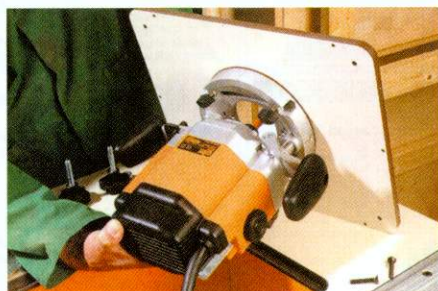
The router is mounted on an insert plate in the CMT , Performance Pro and Charnwood tables
