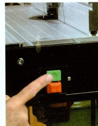
Trend's NVR switch is more robust than most of the others
