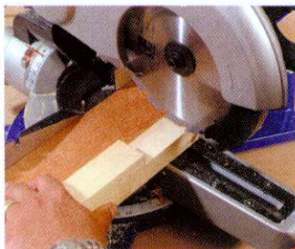
You'll need to pack timber off the fence for flat-bottomed housing cuts
