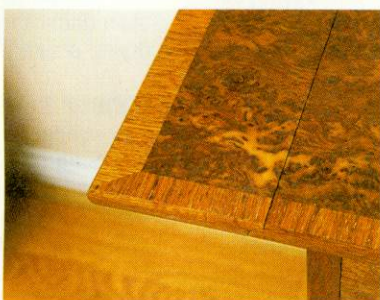
The central burr veneer is bordered by edge banding. Note how the veneer design runs across the entire table top and flaps
