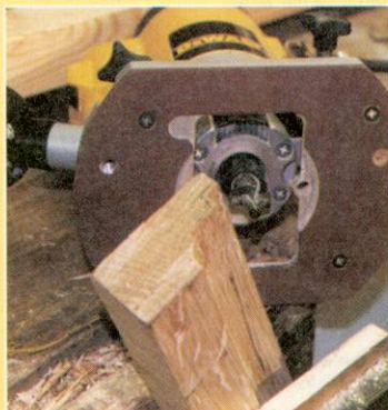
9 Make the mouldings by routing from the solid or by building up several thinner moulded sections
