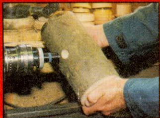
I mounted the blank on a 1in expanding mandrel for my Multistar Duplex chuck
