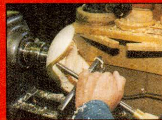
Turn the inner surfaces from the centre outwards to the rim
