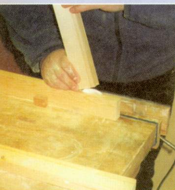
1 The carcass frame can be biscuitied together rather than morticed and tenoned. Use 2x1 PAR pine
