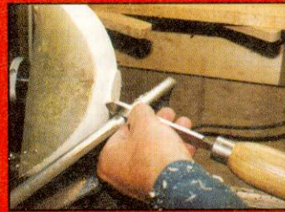
Turn the exterior to shape and form a dovetail foot for your combination chuck
