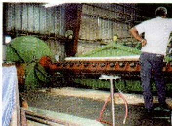
A veneer slicing machine at work as seen at www.fpl.fs.fed.us
