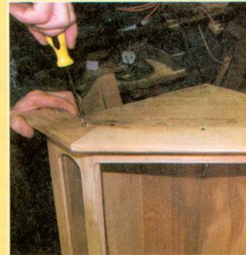
12 The top mouldings overhang the carcass by the same amount for a balanced look. Screw these in place
