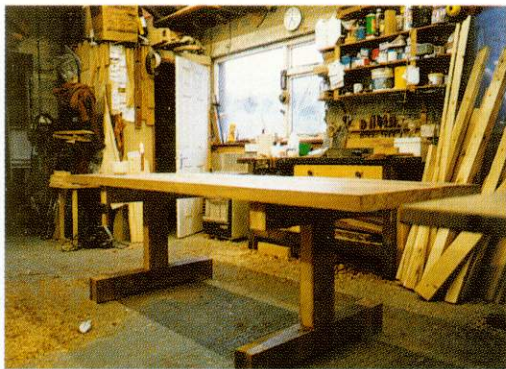
3 The first mock up to check the proportions, the height etc... When I first decided to take on the job I had not anticipated the sheer weight and length the table would be
