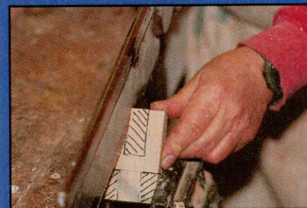
The scratching part of the post joins the base board with a yoke. Shade the waste and then cut to form the tenon and the bridle joint
