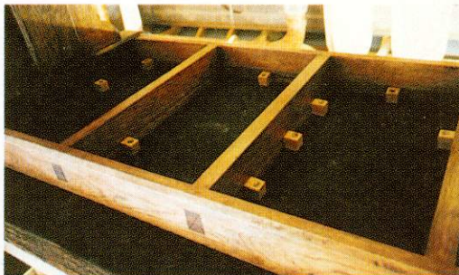
8 First fitting of the top. With the table upside-down the whole underframe was positioned and the buttons, which I had made previously, were fitted. All the screws were greased
