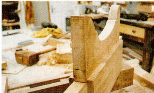
4 The packing pieces or stiffening knees are trenched into the trestle upright for \frac{1}{4} in. The top is lighter than the bottom and the curve decreases its radius as it falls
