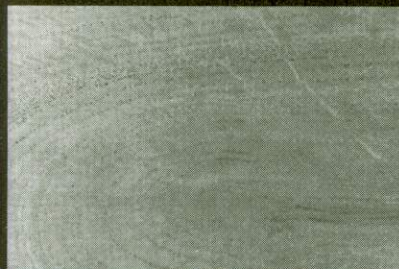
AFTER. With a well-tuned smoothing plane, working against the grain is no longer a problem and you can eradicate all those tears in the oak
