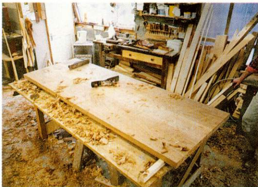
7 After roughing across the grain with jack planes, I worked it with a 24in fore plane. Satisfied with the flatness, I used a fine cut smoothing plane, a dumscape and sandpaper
