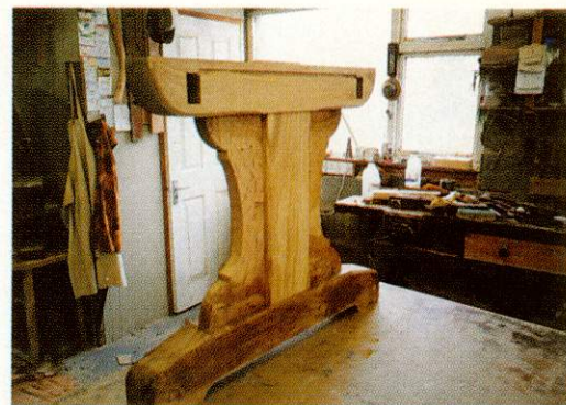
5 A complete trestle except for the main mortice for the beam. The beam was 8x2 \frac{1}{4} in but when held in position it proved too heavy and finished finally at 6x2 \frac{1}{4} in
