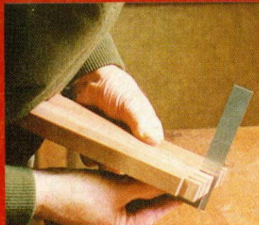
Check that the socket floor is square to the face side. If it is not you will need to mark the line again and chisel the floors all square
