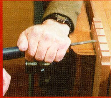
A thump with your hand should be sufficient to propel a narrow chisel. Notice how the left forearm is supported on the vice
