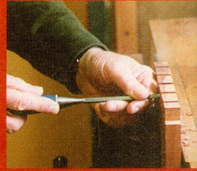
For finishing off the bottom of the pin socket you need a more delicate touch. Support the chisel with your left hand
