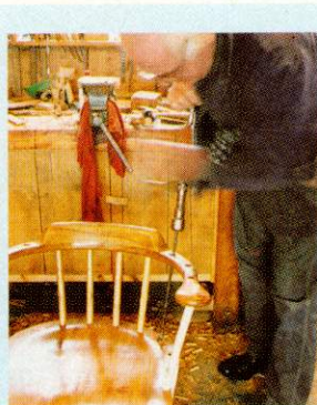
↑ 14 A way of accurately boring the seat. The two front posts are temporary to hold the arm in place
