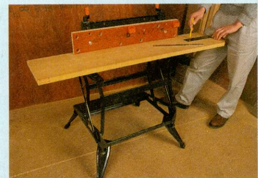
The Black and Decker WM800 has a swivelling front jaw. This is great for holding work but not so good for gluing up work at 90°. The jaw does not stay at 90° as you tighten the handles
