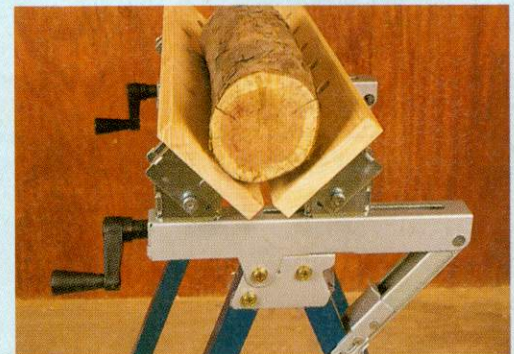
For holding cylindrical items, tubes or logs you can tilt the jaws on the Richmond bench to 45°. Vertical clamping is possible. Huge plastic dogs are supplied, and are a bit too tight for the holes
