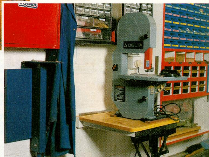
Finding a place for the bandsaw was almost impossible. Tony devised a folding table on which the bandsaw could stand while in a working position. The table could then be folded up and stored against the wall when not in use, and the bandsaw stored on the main workbench
