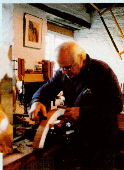
↑ 14 A way of accurately boring the seat. The two front posts are temporary to hold the arm in place
