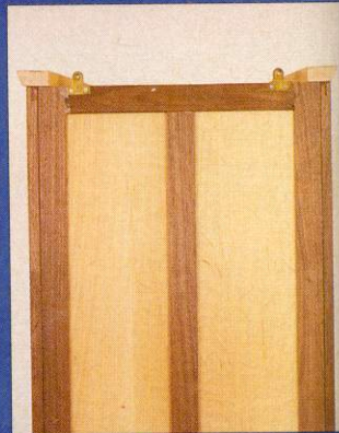
The back panel has two stiles on either side, a rail top and bottom and a central dividing stile
