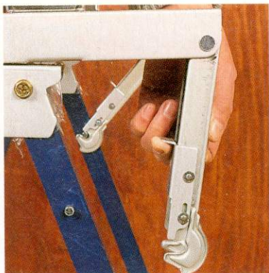
The Richmond BW99/0200 bench has spring-loaded arms to lock the A-frame legs in place. You slide a lever upwards on each folding arm
