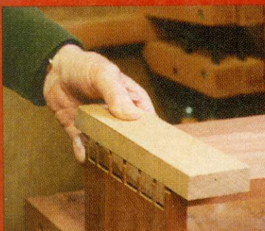
In the early stages of dovetailing you might want to dry assemble first. Make sure the tails are bedding down evenly
