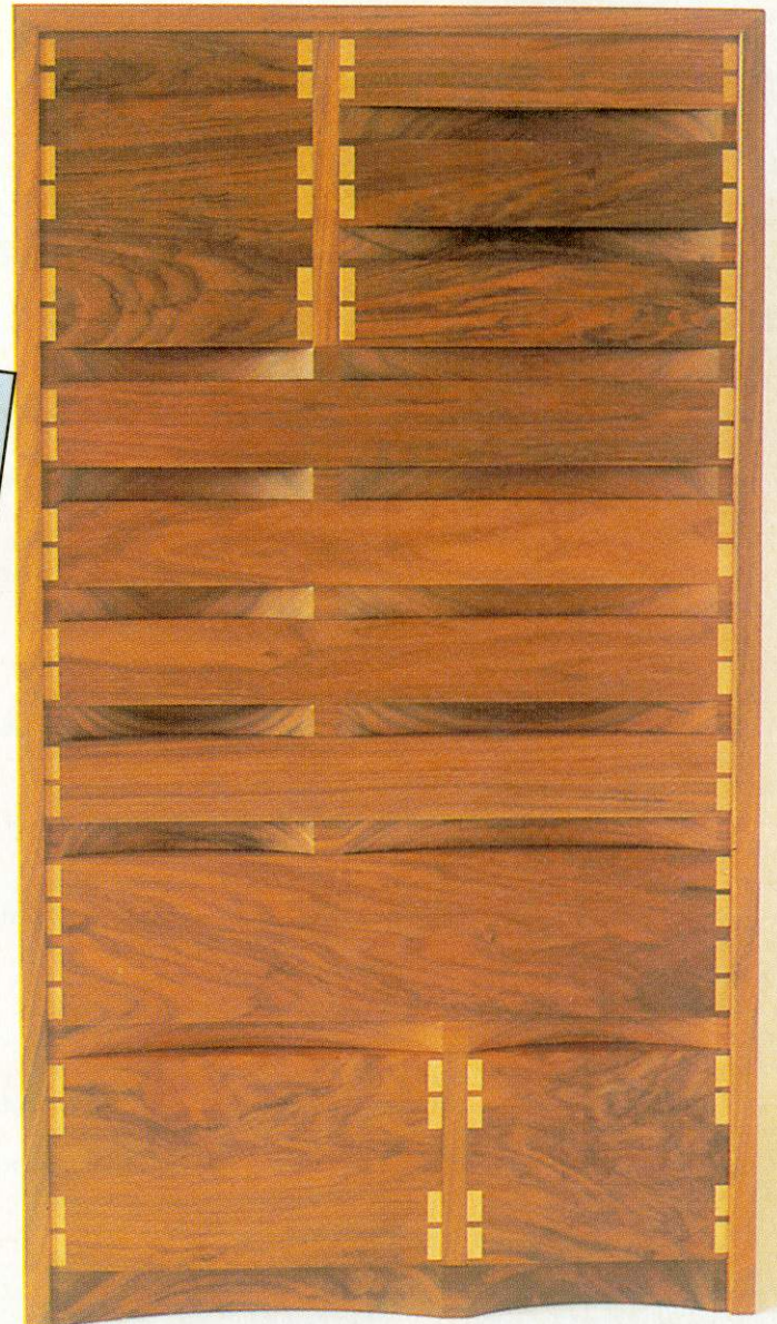
The front of a walnut chest shows how Alan Peters uses the contrast of sycamore and through dovetails in the drawers to distinctive effect. Alan favours the use of oak drawer sides with dark woods, and Honduras mahogany (from old furniture) with lighter colours
