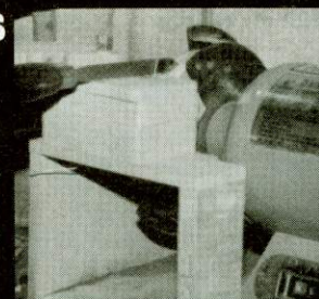
When grinding tools L. Purcell has a stack of MDF leaves as a tool rest
