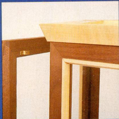
The mitres are strengthened with walnut splines. Assemble these frames before you plane the long bevel on the stiles
