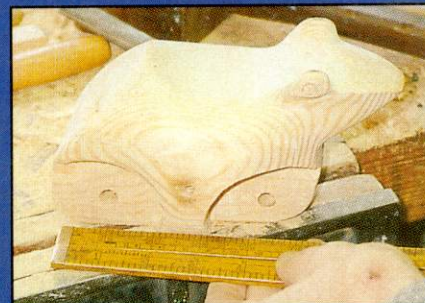
Shape the body of the frog after you have drilled the recesses for the wheels and the holes for the axles
