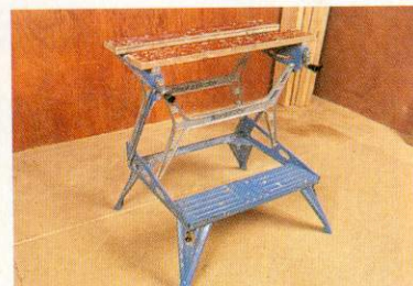
Early Black and Decker Workmates had alloy H-frames supporting the vice jaws. In its lower work position the feet had fine height adjusters
