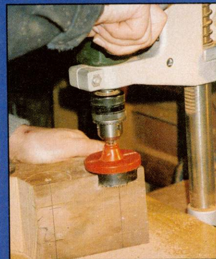
One way to remove waste from the frog body for the wheel arches is to use a hole-cutter. It is best to have the drill in a drillstand for this operation
