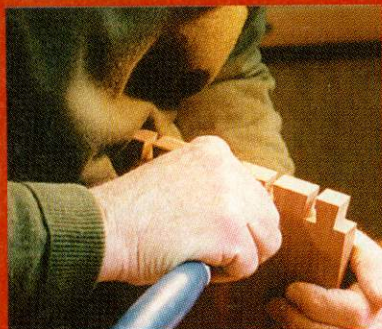
Rectify any inaccuracies with a chisel, then sharpen any corners so they are sharp for a good fit. Use a light to show what is happening
