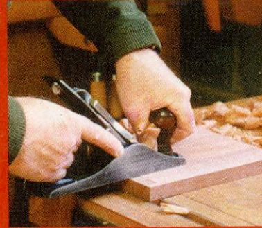
Having made the joint with the faces proud of the joint by a whisker you can clean up by planing back the sides
