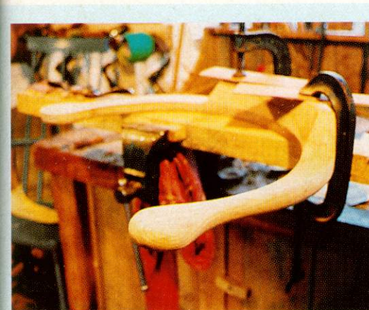
↑ 12 One half of the arm is shaped. The piece of 4x2in in the vice makes a good platform from which to work. It is important to get nice flowing shapes
