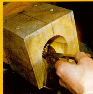
5 Use a shear scraper, having drilled the core and then removed the bulk with a skewed, straight-ended scraper
