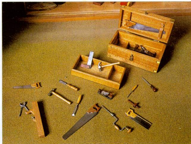
Making the tiny tools is easier than you might think: the hammer heads are cast, the brace is made of piano wire and most blades come from craft knives
