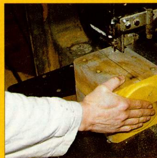
4 Cut a short section off the block. This will be the base of the jug, and will be fitted to the mould last
