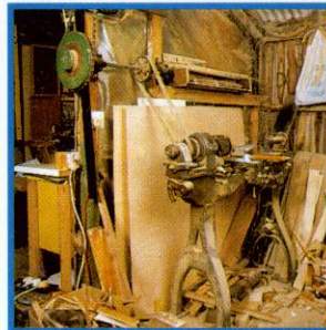
Once a turner, Brian cut away part of the bed of his lathe for bowls
