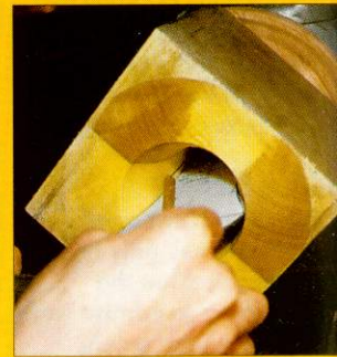
6 Use the pattern to check the shape, pencilling areas that need more work. Copying pencils work best, not HB
