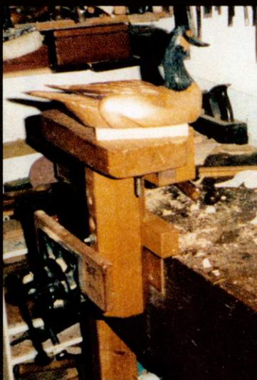
Ted Jenner's carving platform is best made of hardwood for the strength and to stop wear
