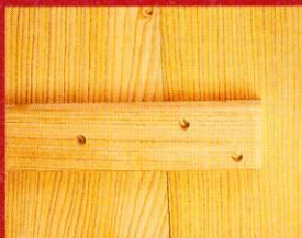
The top piece on the classic bedhead needs the support of a brace to ensure it stays still
