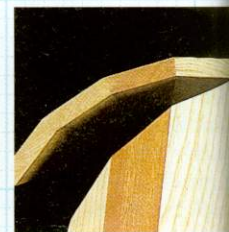
The angle on the edges of the strips is 9° for a 90° curve
