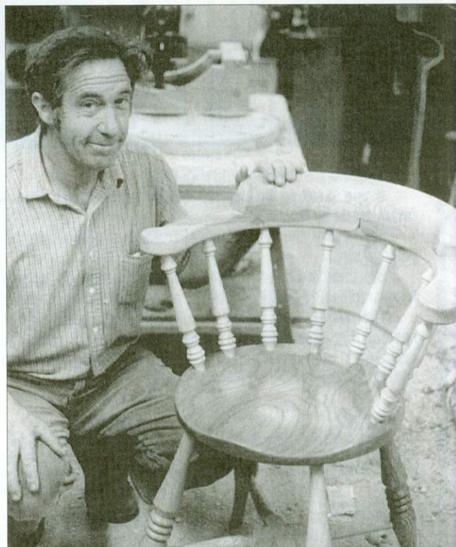
Derek Bailey has been able to make a series of country chairs with his chair hollowing jig, which creates a horseshoe seat, with little cleaning up needed
