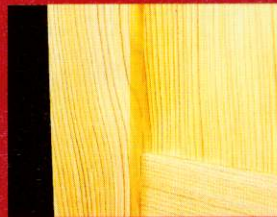
The box bedhead boards fit in the groove. The boards and groove are the same width as the rail tenons
