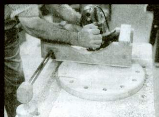
Then fix the seat again, with the axes lined, and start moving the carriage out along the rod, till you finish the seat
