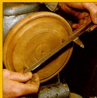
3 Fix a wooden plate to your faceplate and cut a mating register to match that cut on the initial block
