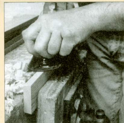
2 Mark the ends and faces of the strips for the angle, and plane carefully. It is essential you do not taper the strips and put the lid in wind
