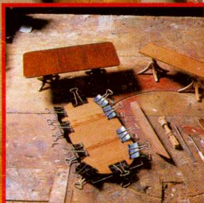
Bulldog clips, crocodile clips and rubber bands make good cramps. He uses bamboo skewers for dowel
