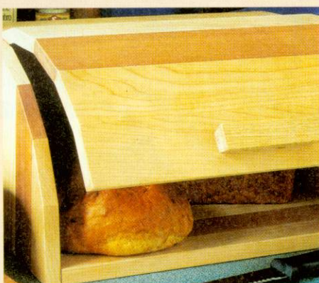
The breadbin is made from offcuts, with the hinging lid coopered to produce the curve through 90°. You could equally make it from PAR softwood
