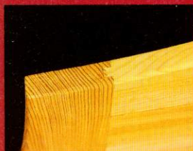
The haunch is visible on the top of the leg on the tent bedhead. You can use a hidden haunch (GW 11:60)
