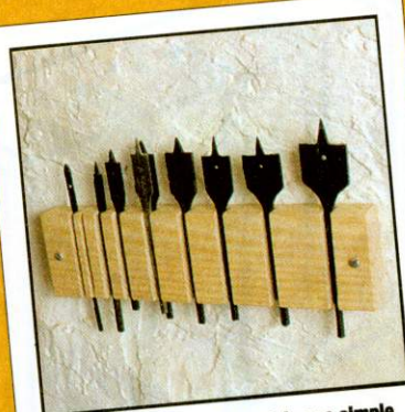
Jeremy Broun's flatbit rack is one simple step towards keeping your workshop tidy, and it can be made in less than an hour
