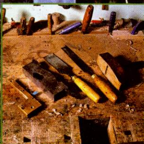
A boxwood scratchstock and pattern-making chisels are used regularly
