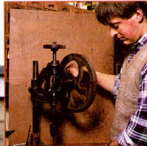
The Bradston No.1 hand-powered pillar drill has automatic feed
