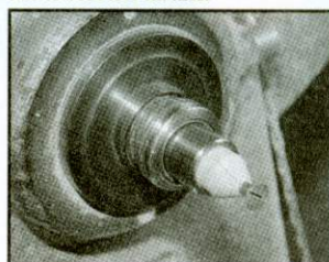
5 Screw a woodscrew into the point. As you can see the point split because we turned it too early
