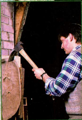
Philip's wall clamp makes using his Wm Greaves No.2 adze less back-breaking
