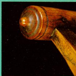
The back leg nipple tops are as typical as the spindles. Only the top back rail needs to be pegged, and then only from the back
