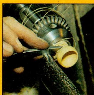
5 Having rounded the rim for a good pop fit, shape the outside of the lid down to the handle
