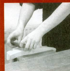
5 Clean up the sides of the fly box with a cabinet scraper, before cutting off the ends
