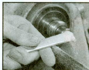
3 For the tailstock centre we started by turning the point, but this is best left till later
