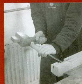
3 Chop away the waste with a chisel and mallet, working from both sides to stop splitting
