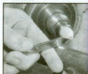
6 Cut off the screw head and turn the shank to a ring and point for the most stable centre
