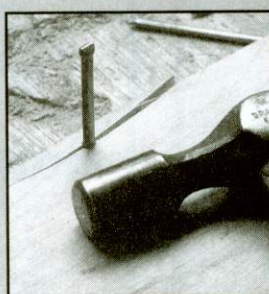
Do not use a nail too close to the edge, especially where the grain curves out towards the edge
