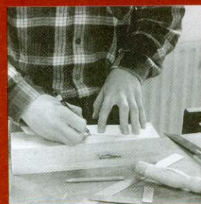
1 With the three pieces stacked up, mark out the top and bottom shapes from a card template
