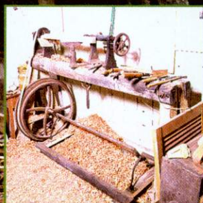
The 19th century treadle lathe gives the marks found on old chairs
