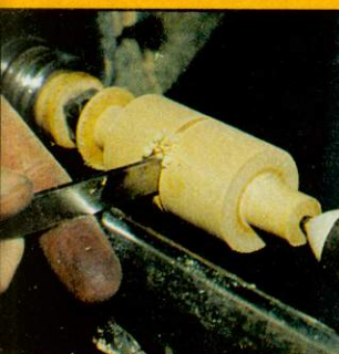
2 Parting off between centres can be dangerous, so complete parting when the blank is in a chuck
