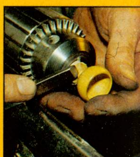
6 Sand and polish the lid, and shape the handle, before parting it off with the long point of a skew
