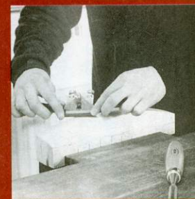
4 Use a flat-bottomed spokeshave on one side, but you will need a convex sole model for the other
