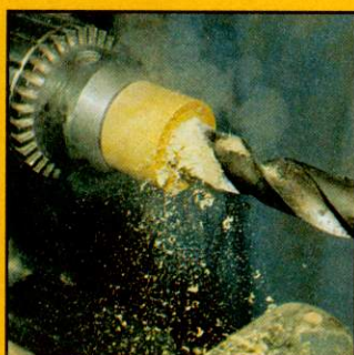
3 Drill into the lid to reduce the hollowing needed. Use Sellotape as a depth stop on the drill bit
