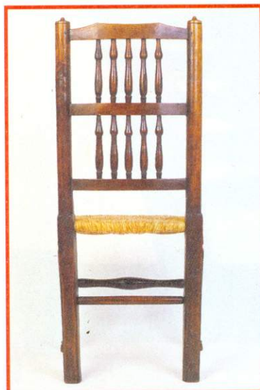
The back legs not only have a rake of about 5° from the shoulder of the turning upwards, but because the timber was turned green it has bent considerably where the grain changes
