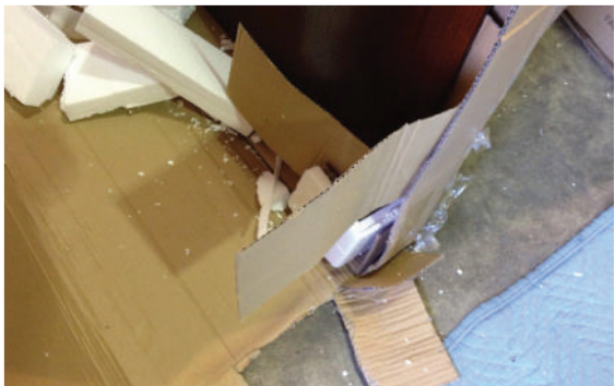
Damaged frame: The leg is completely broken. Reorder of the complete item took over two weeks. Damaged Packaging: Upon opening carton, prior mishandling was obvious. Foam Corner Blocking: Carton was dropped somewhere along the supply chain causing the foam block to crack.
