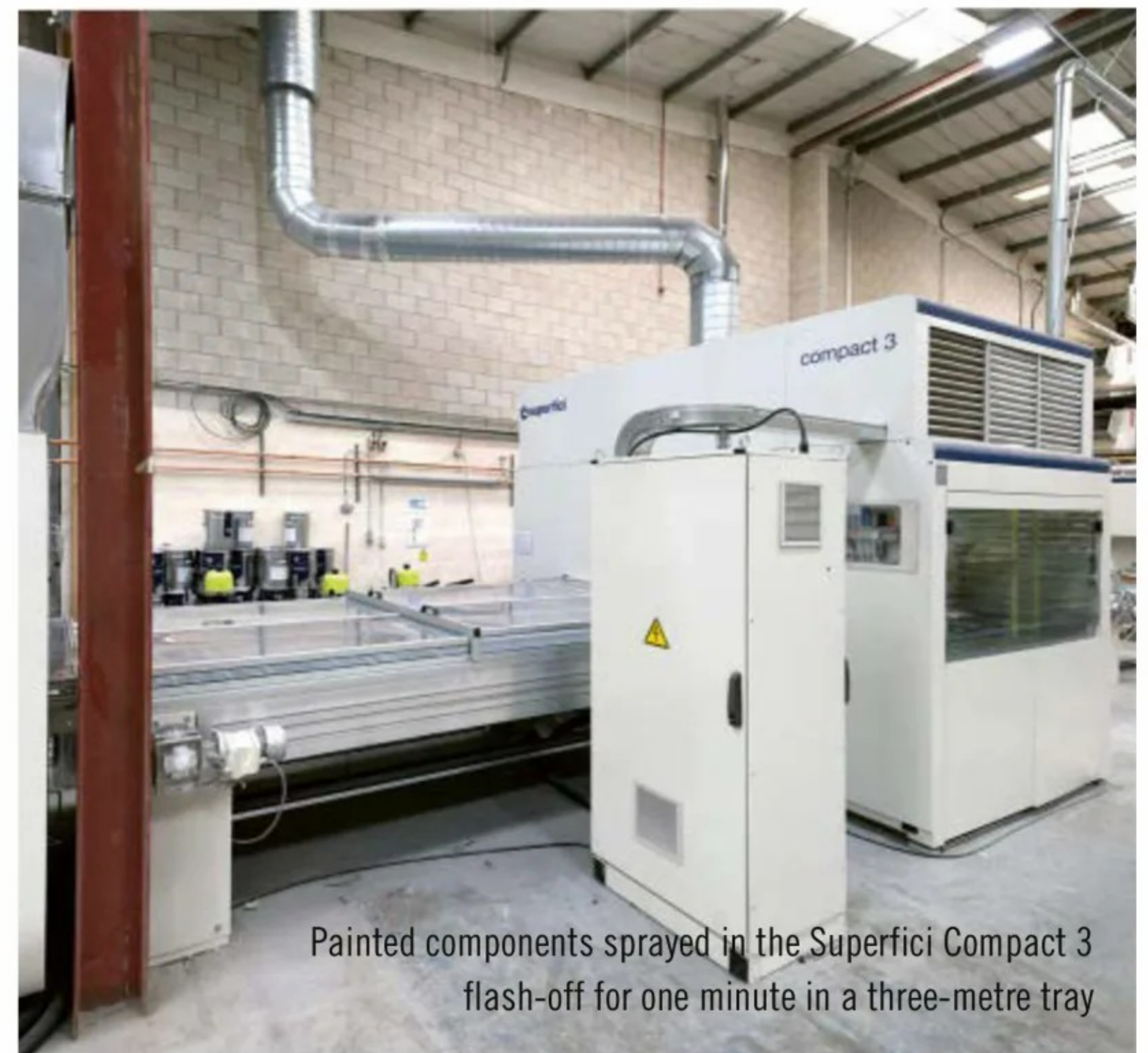
The Superfici Compact 3 is equipped with 12 guns grouped in fours and a paperless recycling system
