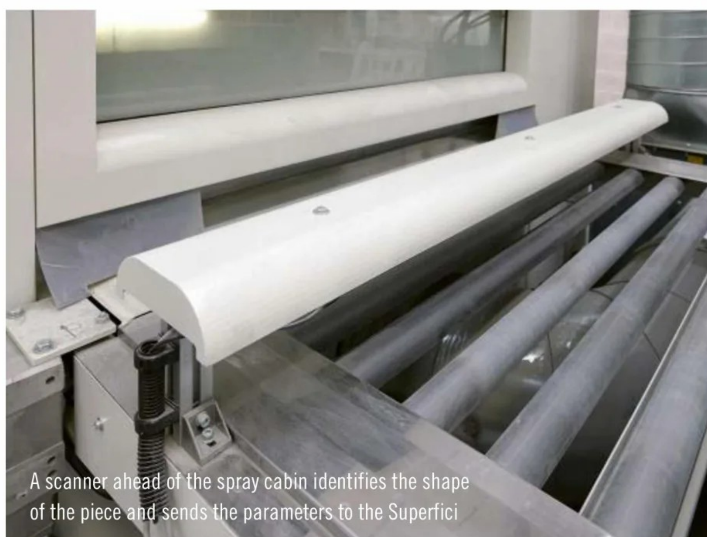
Frames from the sander pass beneath an extractor that removes any dust and are then cleaned and heated with infra red before entering the spray cabin.
