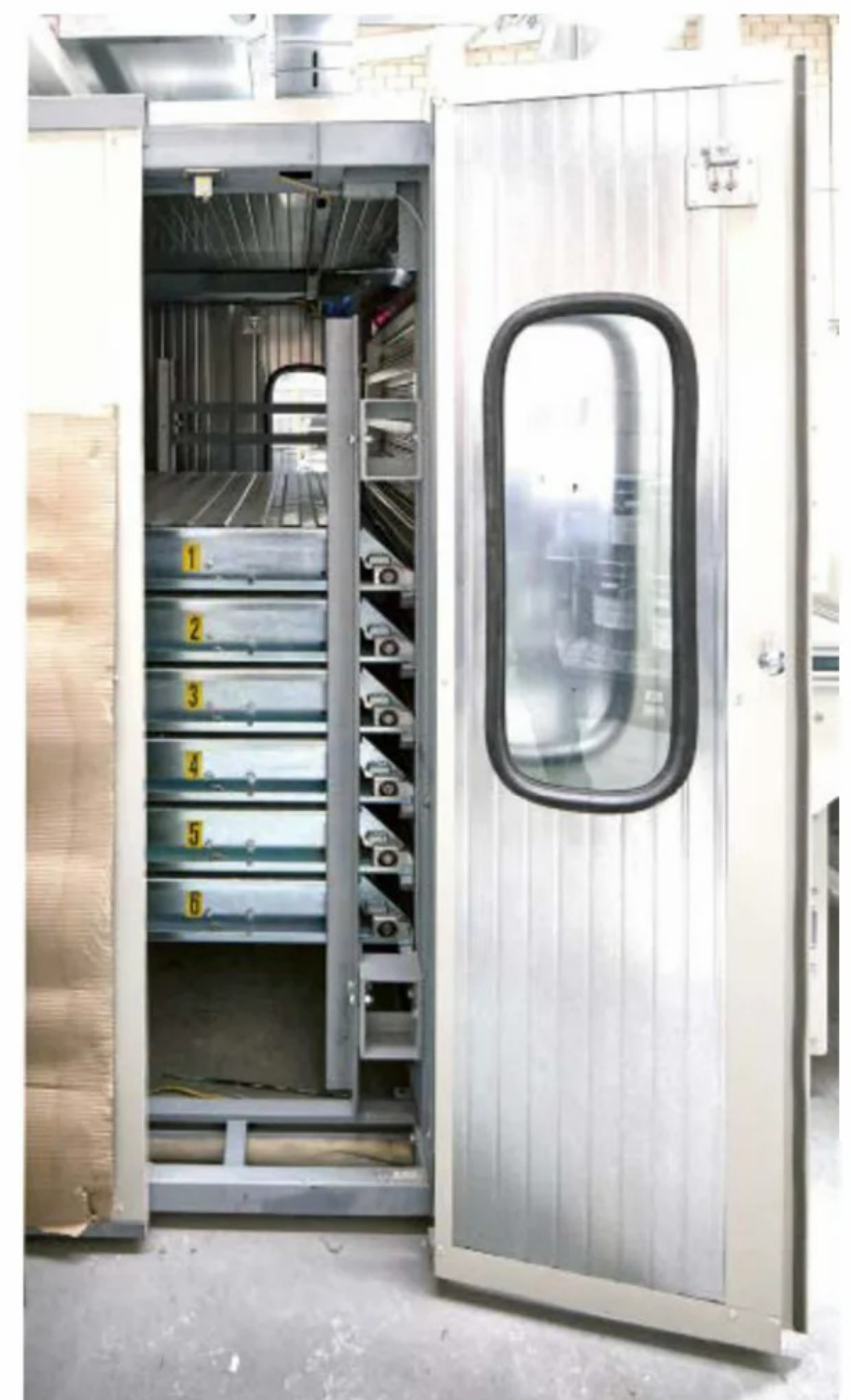
Painted components sprayed in the Superfici Compact 3 flash-off for one minute in a three-metre tray
