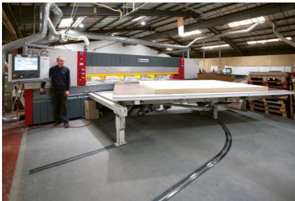
When the machine does its head cut and pushes the panels out, the operator presses a button and the turntable turns the whole stack around so it can be pushed in again.
