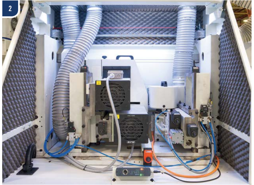
2. Compact double-hogging and anti-chipping units. Different solutions are available in the panel preparation zone.
