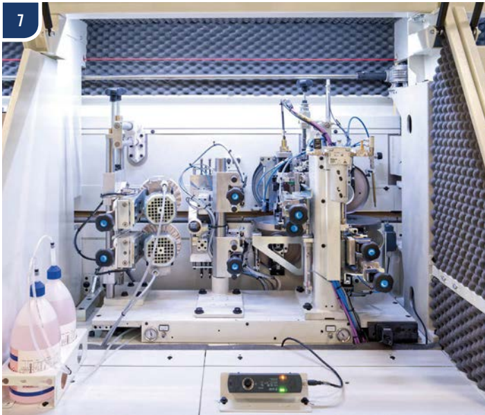
7. Finishing station with edge scraping unit, multileaf glue scraping unit and brushes
