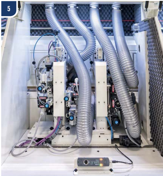
5. Finishing station with trimming and fine trimming units
