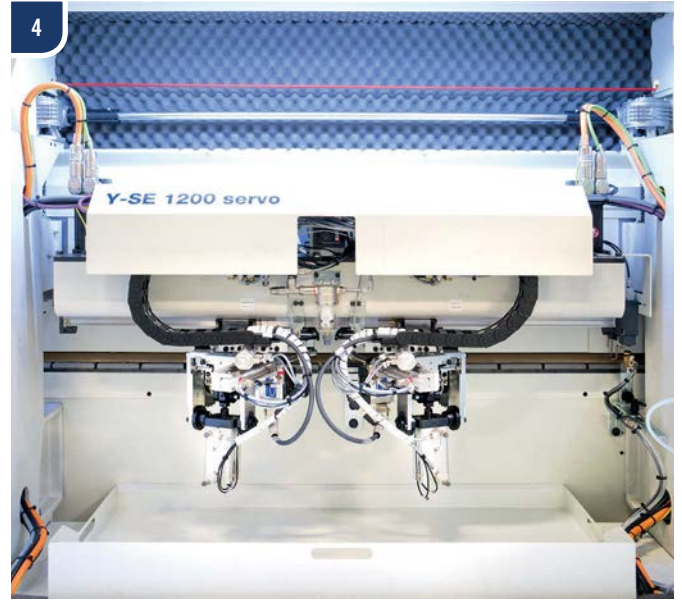
4. Electronic end-trimming unit suitable for delicate materials.
