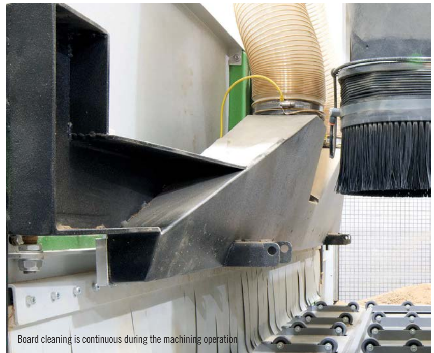
The vacuum is so strong that it's enough to suck through two boards.
