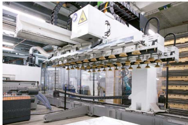
The Synchro operates along a track, loading and unloading two panels at a time.
