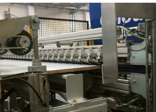
Cleaning of chipboard prior to camera-based inspection
