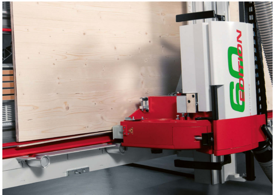
Striebig Edition 60 bottom trim (above) and clamps (below).
