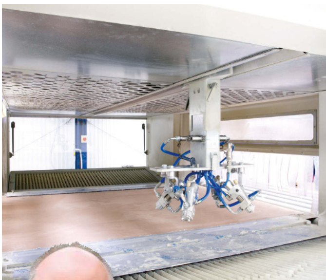
The infeed is 1300mm wide and Mark's Superfici Mini P uses paper rather than having the optional recovery or hybrid systems.
