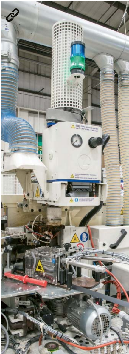
Above: Stefani's fast changeover SGP glue pot and PU BOX L pre-melter.
