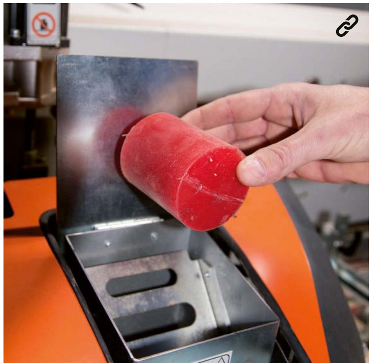
Main image: Lumina 1598 with Return-Master 5920 panel return system. Above right: GJ702 GluJet system. Right: Cleaning chamber and cartridge for neutralising PUR.
