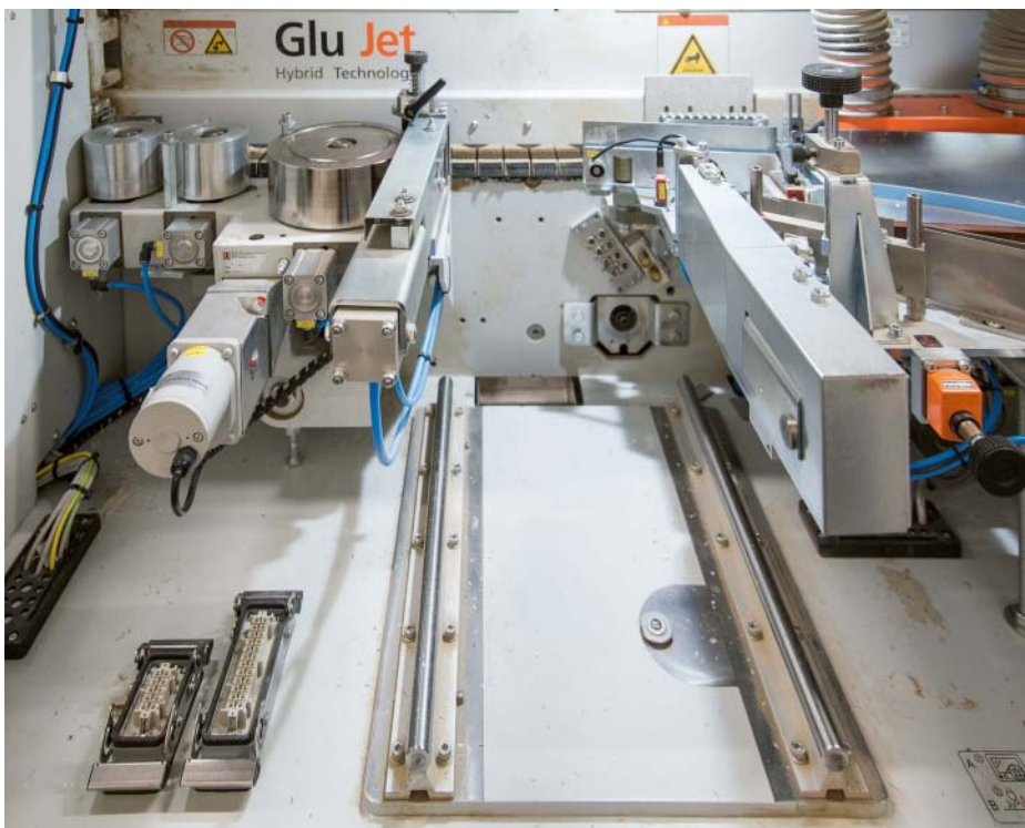
Top and left: Changeover from the GluJet system to the Ltronic laser is fast and efficient – slide one out, slide the other in.
