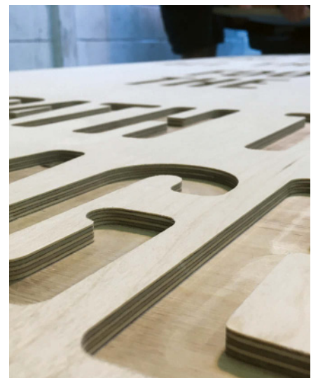
The cross-layered veneers that form a sheet of plywood make it incredibly stable even when patterns are routed out.
