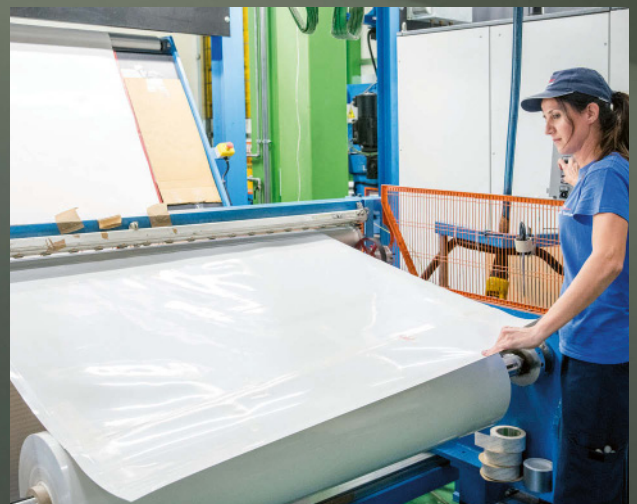
Bonlex Europe has three inspection lines and every roll is carefully controlled for quality, both by camera and by specially trained quality inspectors.
