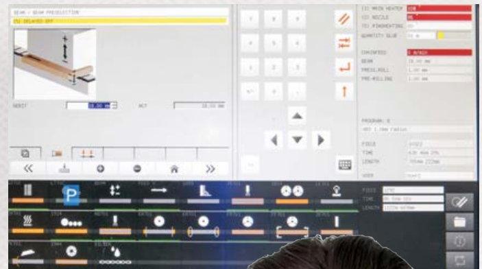
Below: From the controller, the laser edging is selected from a database and set up of energy requirement is automatic.
