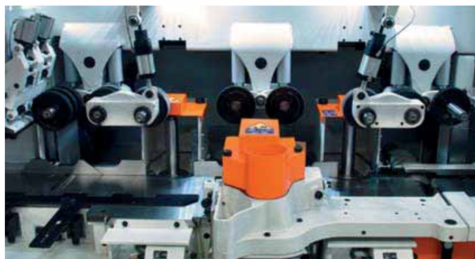
Configuration with two right vertical spindle on Superset NT
