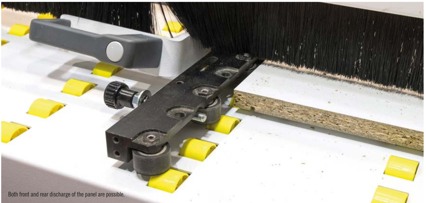
Vertical and horizontal drilling, routing and boring from below.
