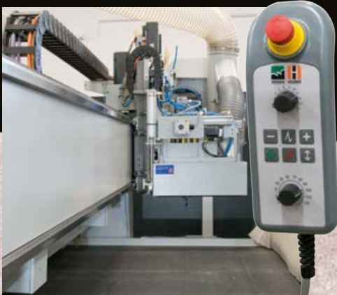
Transport to the processing table is automatic, via a pull-in device with side positioning, and suction cups remove the panels.
