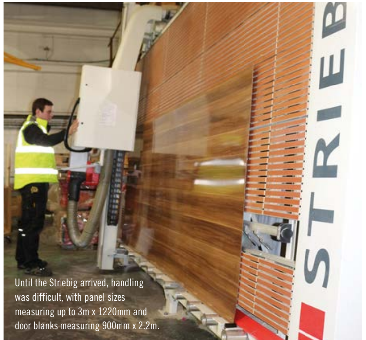
A digital measuring system on both axes, programmable control system and automated cut cycle were just some of the reasons Trovex chose the Striebig Control 4216.
