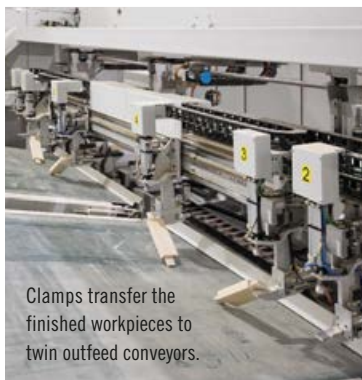
The twin outfeed conveyors are beam controlled.
