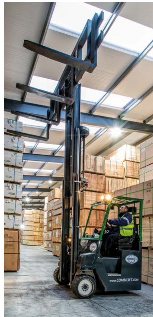
A spreader bar makes easy work of moving five-metre lengths.
