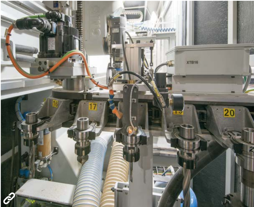
Left and above: A Balluff chip and reader tool identification system identifies and automatically manages the tools and tool data.
