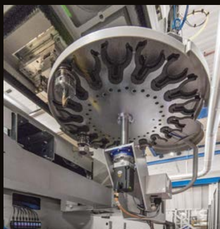
Above: Silentnight's Dynestic has an 18-position tool-changer and Holz-Her's "Touch Tool" tool length detection system.
