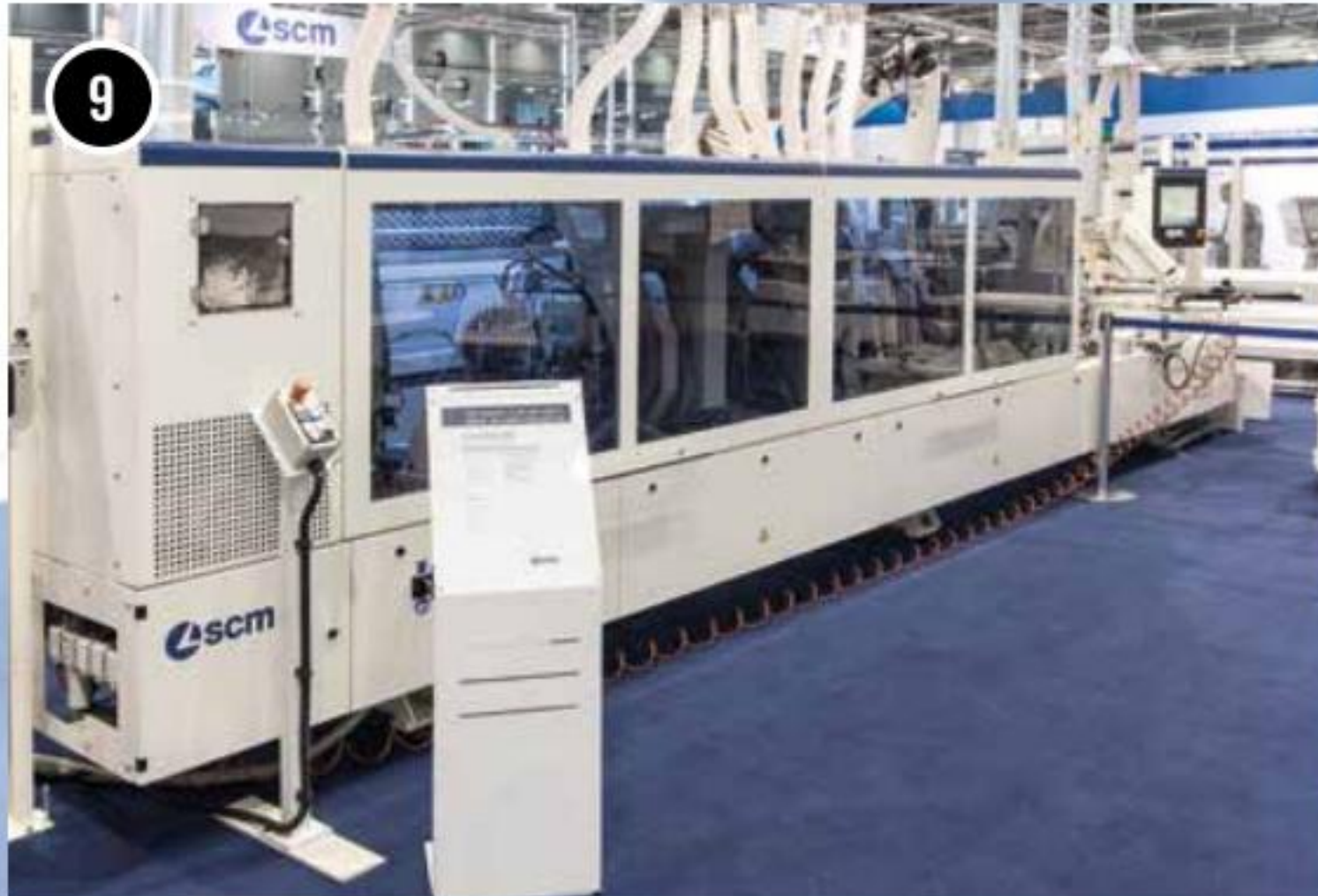
9: The Stefani XD edgebander (left and below), chosen for its multi-tape feeder. The edgebanded panel is returned to the robot (below left).
