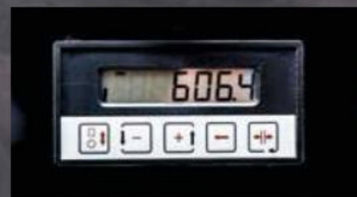
The Standard S is equipped with a digital measuring unit.
