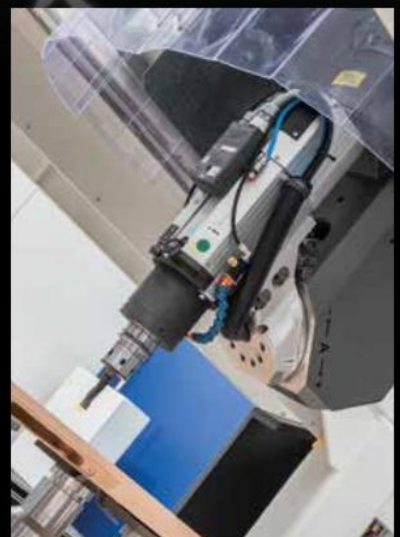
Maka's standard five axis head on a PE90.
