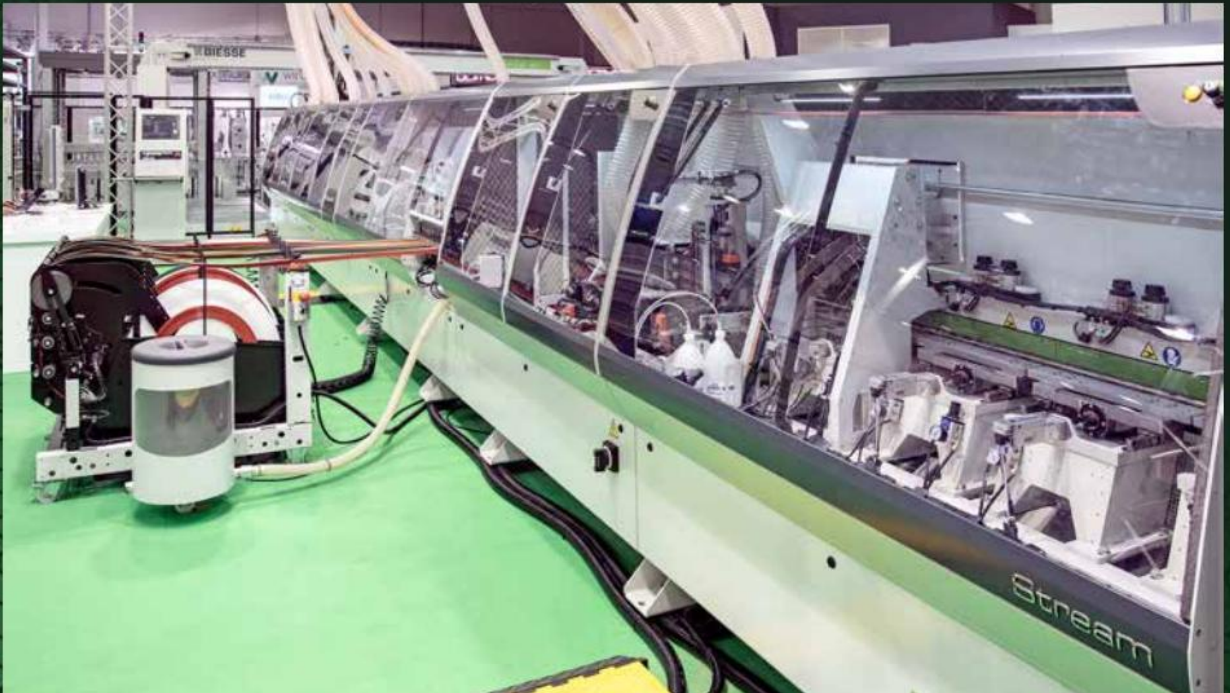
The new quick changeover system uses adhesive in cartridge form and can accommodate 0.25kg or 2kg slugs.
