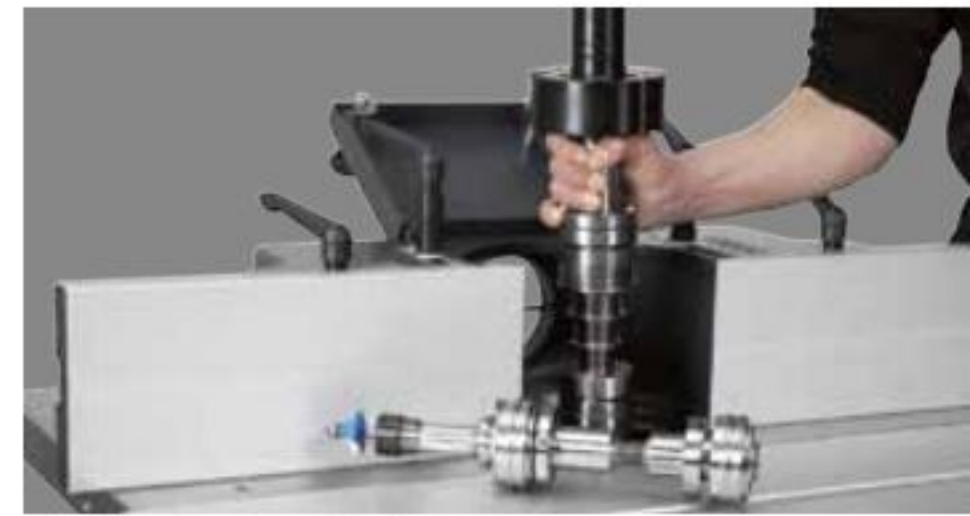
Quick change spindle system - Change over without tools
