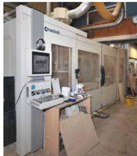
Left: Cross and Sansam's largest Routech Chronos HT is equipped with a five-axis Prisma Q machining head.
