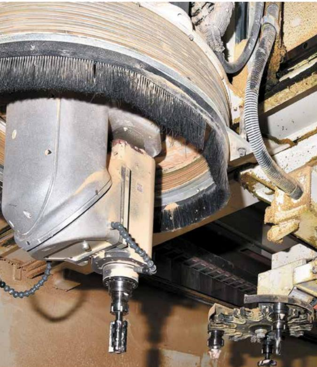
Left: Cross and Sansam's largest Routech Chronos HT is equipped with a five-axis Prisma Q machining head.
