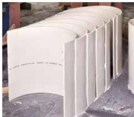
Clarendon chose Hi-Macs, which they formed with a Curvomatic system, to make the nine-metre tapered columns for a contract project in London.
