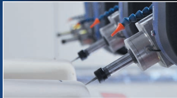
Above. A multi-head, twin table, five-axis Maka machining four high gloss finished curved fascias simultaneously.
