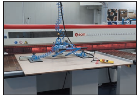
Below. SCM's lifting device ensures easy panel handling.
