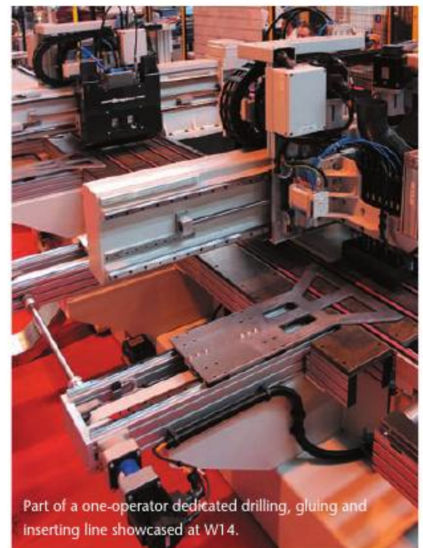
Custom built drilling and routing heads.
