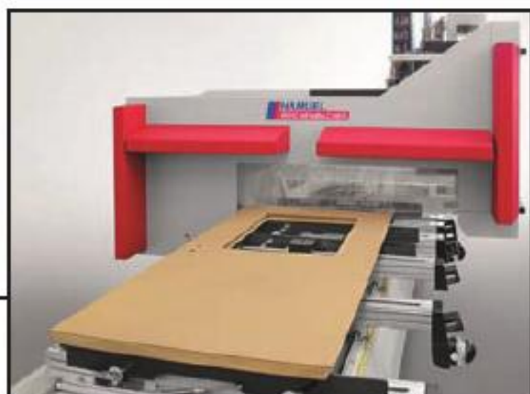
Above and below. The Primus offers a choice of grooved or beam tables with four to six manually adjustable units.
