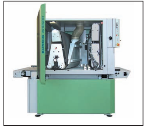
Left. Kündig's BoTop 6 and the extremely popular Brilliant 2 (above), showing the oblique sanding head configuration clearly.
