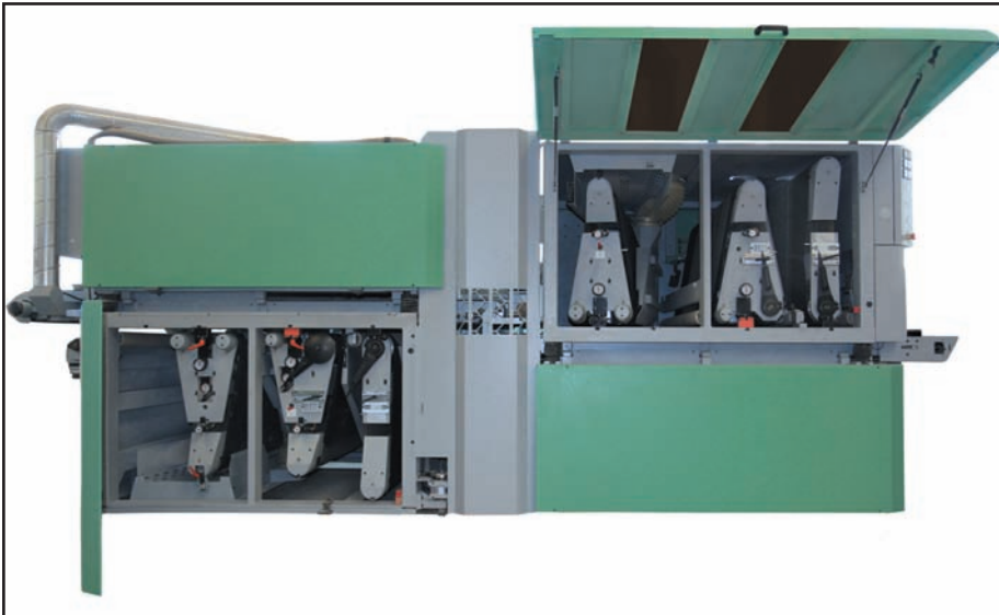
Left. Kündig's BoTop 6 and the extremely popular Brilliant 2 (above), showing the oblique sanding head configuration clearly.
