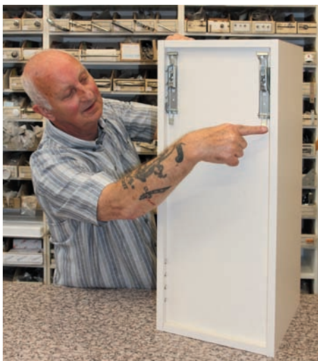
"It can't be that easy. But it was. It really was." The joints simply click together, the back slots in and a thump on the last panel secures the cabinet.
