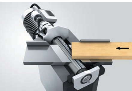
Below: The 30°-angled straightening spindle significantly reduces planing "snipes" and "dips" (Powermat 2400 XL).
