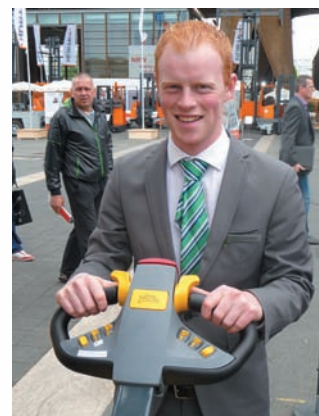
Above: The multi-position tiller (patent pending) enables the operator to remain at the side of the truck instead of between racking and truck.
