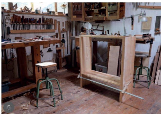
1 Making the rebate for the carcass 2 Fine-tuning the rebate with the shoulder plane 3 Dimensioning the front stiles 4 Using a sliding dovetail plane to make the males 5 Dry fitting the carcass 6 Half-blind dovetails and detail of the stiles
