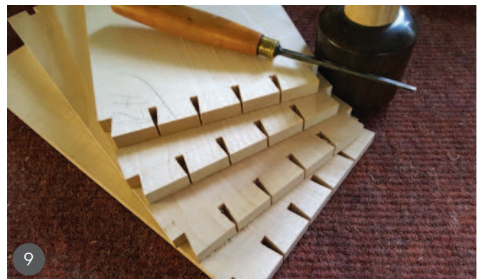
5 A dark timber was chosen for the drawer fronts 6 & 7 The Australian walnut was then prepared for the drawer fronts and fitted into the carcass 8 A sharp plane was used to prepare the drawer sides for fitting 9 The tails were finished with a 4mm chisel
