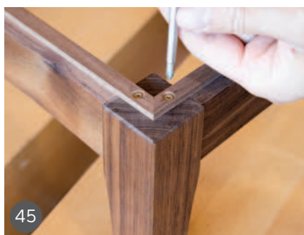
39 A further detail of the gallery 40 Transferring the drawer opening on the small cupboard 41 Determining the shelf location 42 The veneering set-up with a vacuum bag 43 Fine-tuning the fit of the slant front 44 A finger recess was carved to open the front 45 Installing the spacer for a floating effect 46 Shrinkage buttons allow for wood movement 47 The finished piece before leaving the workshop
