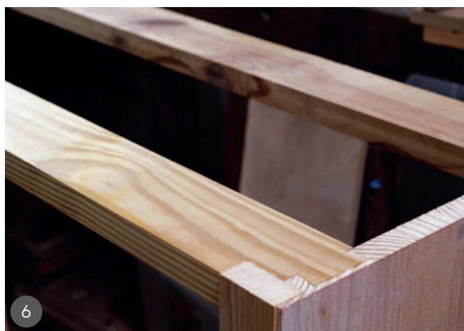
1 Making the rebate for the carcass 2 Fine-tuning the rebate with the shoulder plane 3 Dimensioning the front stiles 4 Using a sliding dovetail plane to make the males 5 Dry fitting the carcass 6 Half-blind dovetails and detail of the stiles
