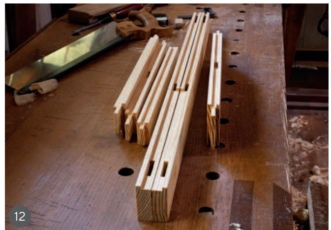
7 Shaping the sides to make the legs 8 Gluing and checking for squareness 9 Gluing the front stiles 10 The carcass glued up 11 Preparing the door pieces 12 The joinery for the doors
