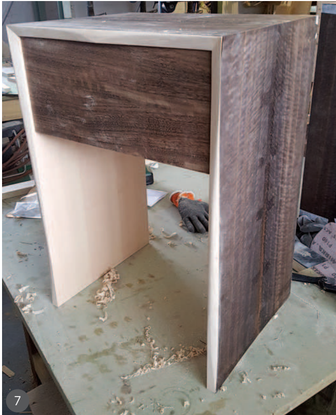
5 A dark timber was chosen for the drawer fronts 6 & 7 The Australian walnut was then prepared for the drawer fronts and fitted into the carcass 8 A sharp plane was used to prepare the drawer sides for fitting 9 The tails were finished with a 4mm chisel
