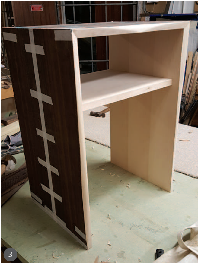
1 Detail of the shaping on the top edge 2-4 After shaping, the carcass was glued and clamped
