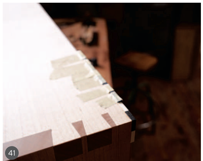
32 Working on the bridle joint tenons 33 Working on the mortises 34 Dry fitting the frame 35 The red cedar for the panels 36 Detail of the back 37 The finished back, fixed into the carcass 38 The ebony and holly sticks for the edge inlays 39 Gluing the corner pieces 40 Detail of the corner pieces already planed flush 41 Gluing the rest of the pieces
