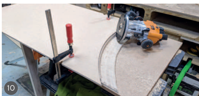
8 Biscuit-jointing the stacking sections 9 Laying the completed wing sections across the rod 10 Cutting the rebates on to the wing sections 11 Test-fitting the three main sections 12 Final fitting of the central hub section 13 Cutting Domino joints into the hub and wings
