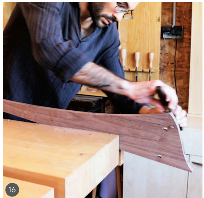
13 Routing the rebate for the mirror 14 Shaping the component with a flush-cut router bit 15 The components are almost finished 16 Shaping the edges with a spokeshave
