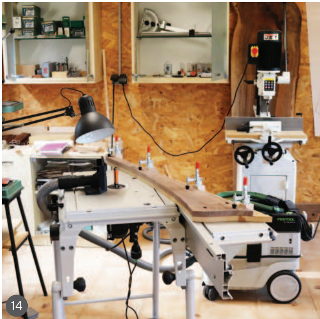
13 Routing the rebate for the mirror 14 Shaping the component with a flush-cut router bit 15 The components are almost finished 16 Shaping the edges with a spokeshave
