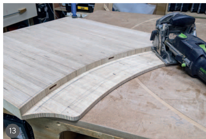
8 Biscuit-jointing the stacking sections 9 Laying the completed wing sections across the rod 10 Cutting the rebates on to the wing sections 11 Test-fitting the three main sections 12 Final fitting of the central hub section 13 Cutting Domino joints into the hub and wings
