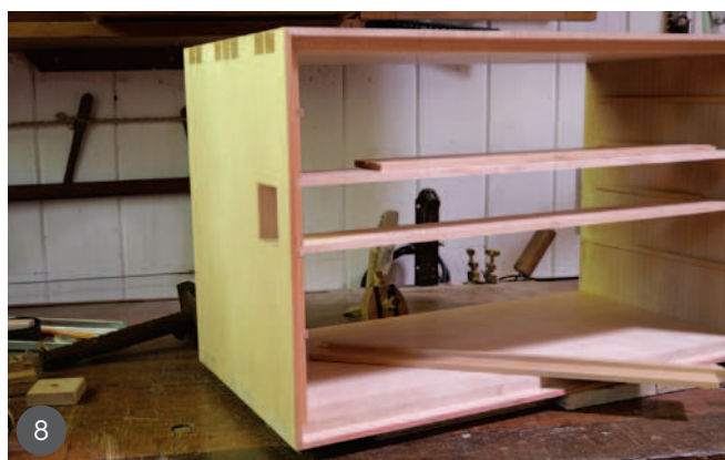
1 Making the dovetails for the carcass: adjusting the tail shoulders 2 Paring the tails 3 Transferring the tails to get the pins 4 Dry fit of the carcass 5 Details of the carcass dovetails 6 Rebates for the drawer guides 7 Rebates for the back and opening for the side drawers 8 Working on the side drawers' carcass
