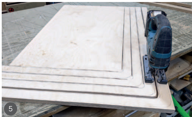
3 The braced leg template on a sheet of ply, doubling up as a forming jig 4 A track saw made the bulk of the straight cuts 5 Finishing the release cut with a jigsaw 6 Routing the leg shapes with a bearing-guided router cutter 7 The completed longer outer leg sections
