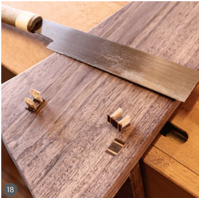
17 The clamping must be even and allow for driving the wedges in place 18 Flushing the wedges with a Japanese flush-cut saw 19 & 20 Installing the mirror with the backing and fixing strip 21 The piece is best appreciated from the side
