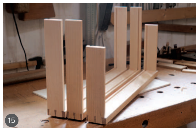
9 Detail of the opening for the side drawers 10 Structure for the side drawers 11 Making rebates for the inlays 12 Carcass glue-up 13 Testing the drawer fronts 14 Detail of the tails 15 Dry fit of the drawer fronts and sides
