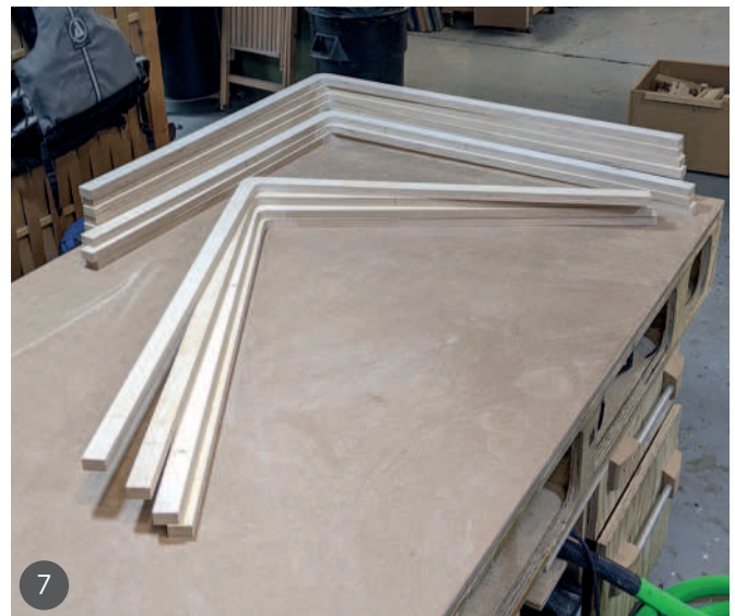
3 The braced leg template on a sheet of ply, doubling up as a forming jig 4 A track saw made the bulk of the straight cuts 5 Finishing the release cut with a jigsaw 6 Routing the leg shapes with a bearing-guided router cutter 7 The completed longer outer leg sections
