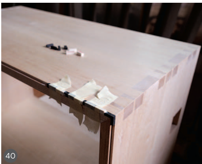
32 Working on the bridle joint tenons 33 Working on the mortises 34 Dry fitting the frame 35 The red cedar for the panels 36 Detail of the back 37 The finished back, fixed into the carcass 38 The ebony and holly sticks for the edge inlays 39 Gluing the corner pieces 40 Detail of the corner pieces already planed flush 41 Gluing the rest of the pieces
