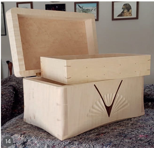
13 & 14 The trays were assembled and fitted into the box 15 & 16 Turquoise veneer was used for the tray bases
