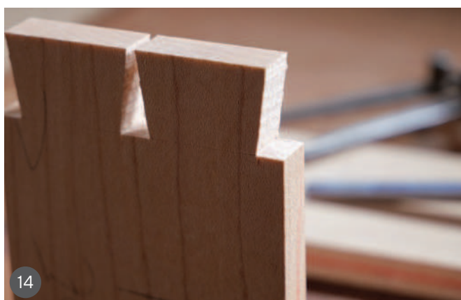
9 Detail of the opening for the side drawers 10 Structure for the side drawers 11 Making rebates for the inlays 12 Carcass glue-up 13 Testing the drawer fronts 14 Detail of the tails 15 Dry fit of the drawer fronts and sides
