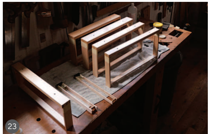
16 Making grooves for the drawer bottoms 17 The sliding dovetails to join the backs 18 Cleaning the drawer sides after glue-up 19 The drawers before adding veneer 20 & 21 Fine-tuning the drawer fronts after veneering 22 Sawing red cedar for the drawer bottoms 23 Applying shellac
