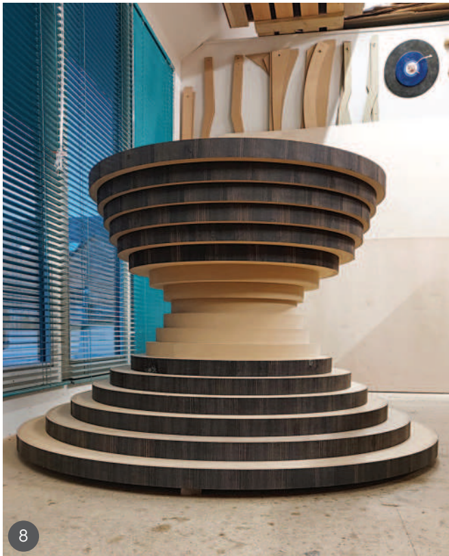
1 & 2 A computer render and a scale mock-up of the table 3 The base rings and ply cores were shaped by a CNC specialist 4 & 5 The set-up for veneering the edging strips 6 & 7 The strips were glued and clamped to the base rings in stages 8 All of the strips were now in place on the table base 9 & 10 The extendable table top features a 72-piece Macassar ebony sunburst
