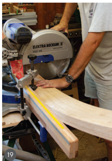
17–19 Machining and cutting the staves to length 20–23 Finishing the stave's curve and cutting to width 24 A sacrificial stave was made from offcuts for the tapering jig 25 & 26 This stave was fitted on to the central panel and set to the slat using the flexible ruler
