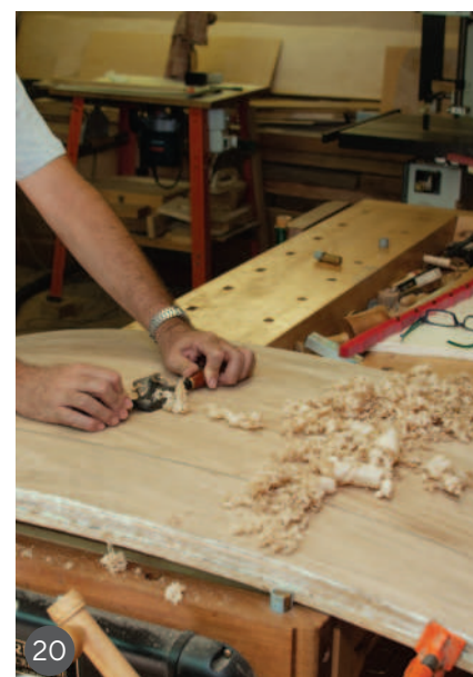
17–19 Machining and cutting the staves to length 20–23 Finishing the stave's curve and cutting to width 24 A sacrificial stave was made from offcuts for the tapering jig 25 & 26 This stave was fitted on to the central panel and set to the slat using the flexible ruler
