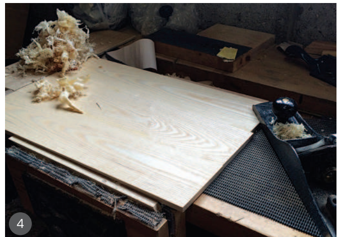
1 Initial sketch ideas 2 A more detailed elevation drawing for the client in watercolour 3 Selection of sawn kiln-dried ash 4 Planing down central panels to side frames using a hand plane
