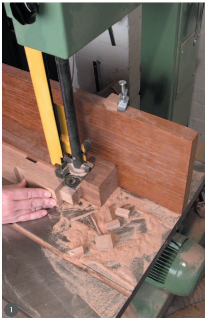
1 Cutting tenons on the bandsaw 2 Cleaning out the angled mortises 3 Clamping blocks located with double-sided carpet tape
