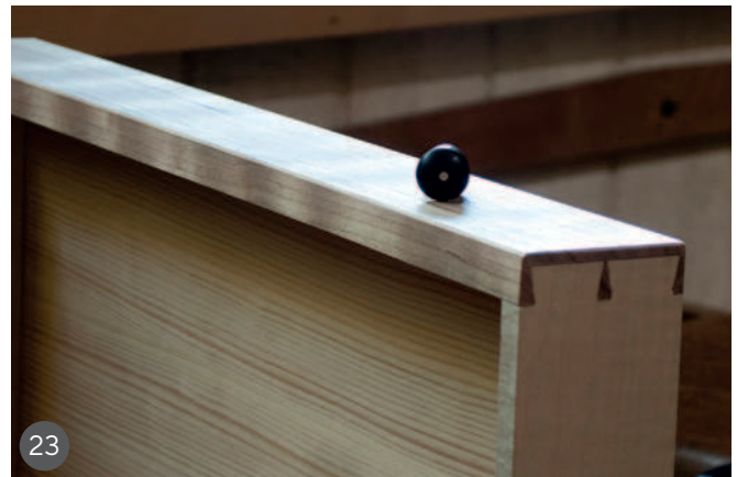
12 Test fit of the dovetails 13 Rebate for division and the mortise for the stile 14 The stile and divisions 15 Making the grooves for the panels 16 Detail of the haunch that will cover the groove 17 Detail of the mortise fit 18 The bevelled panel 19 Testing the door before glue-up 20 Gluing up the doors 21 The shelves in place 22 The ebony door pull 23 The drawer dovetails and ebony drawer pull
