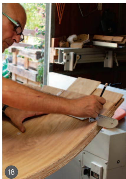
17–19 Machining and cutting the staves to length 20–23 Finishing the stave's curve and cutting to width 24 A sacrificial stave was made from offcuts for the tapering jig 25 & 26 This stave was fitted on to the central panel and set to the slat using the flexible ruler
