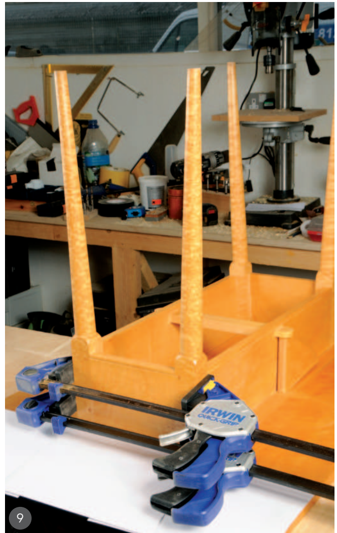
6 Shaping the leg down to start the taper using a spindle gouge 7 Planing the taper with a skew chisel – extra care must be taken near the leg’s shoulder 8 Bandsawing a tenon – note the marking at the top where the haunch waste will be cut away 9 An end frame glued and clamped
