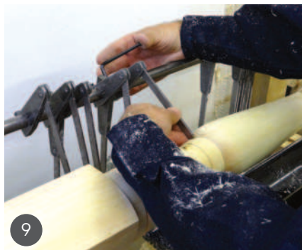
6 Using the template to mark the positions of the details 7 Sizing with spring callipers and my beading and parting tool 8 Knots and pine go hand in hand but, turned carefully, they shouldn't cause too much trouble. This knot shows the finish straight from the tool 9 Setting the duplicating fingers 10 The duplicating fingers in action 11 Turning the sphere detail with the spindle gouge
