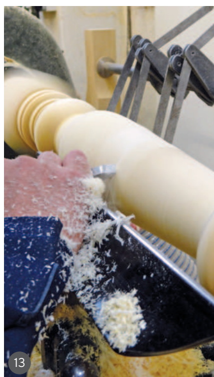
12 Defining the main shape with the roughing gouge 13 Planning cut with the beading and parting tool 14 Forming the coves with the spindle gouge
