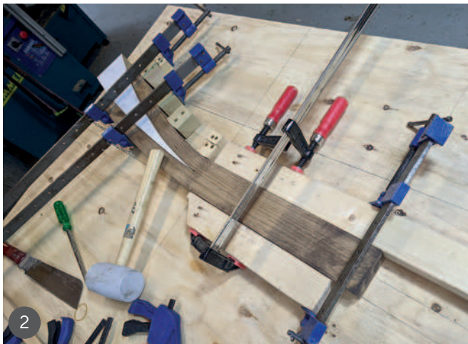
1 A 1:5 scale model was made to test the design 2 Bending jig for steaming attempts 3 A failed steaming attempt
