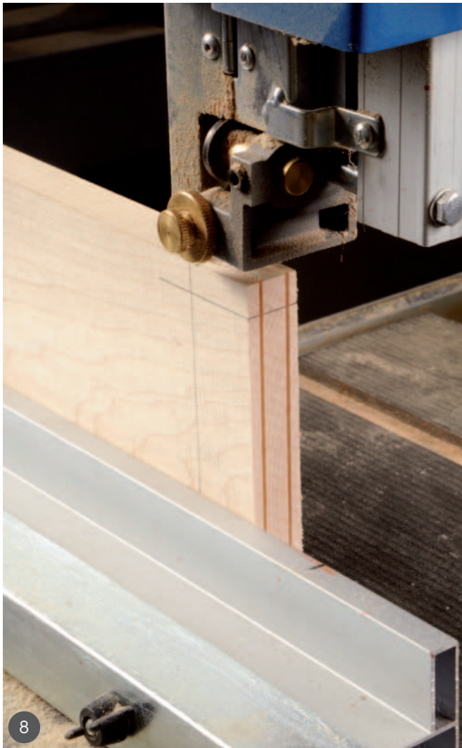
6 Shaping the leg down to start the taper using a spindle gouge 7 Planing the taper with a skew chisel – extra care must be taken near the leg’s shoulder 8 Bandsawing a tenon – note the marking at the top where the haunch waste will be cut away 9 An end frame glued and clamped
