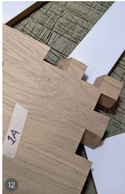
4 Failed test bends 5 My steam box made from ply and insulation board 6 The laminations gluing up on the former 7 A good collection of laminations for the four legs 8 Gluing the two different bends together 9 The tablesaw jig for the long mitres 10 A guide to position the legs right on the corner 11 Letting the legs into the table top 12 One corner finished with through-leg notches cut on both sides 13 Creating the stretcher rails
