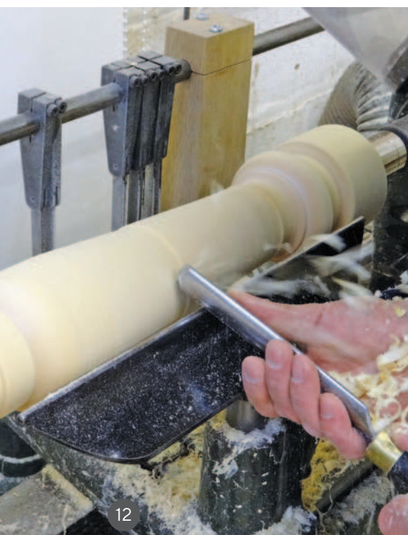
12 Defining the main shape with the roughing gouge 13 Planning cut with the beading and parting tool 14 Forming the coves with the spindle gouge
