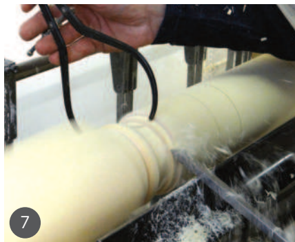
6 Using the template to mark the positions of the details 7 Sizing with spring callipers and my beading and parting tool 8 Knots and pine go hand in hand but, turned carefully, they shouldn't cause too much trouble. This knot shows the finish straight from the tool 9 Setting the duplicating fingers 10 The duplicating fingers in action 11 Turning the sphere detail with the spindle gouge
