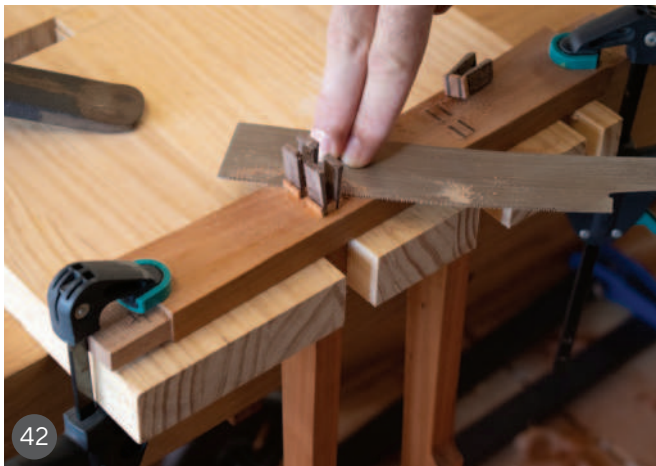
40 & 41 A removable box was made from contrasting timbers 42 The box's mortise and tenon joints were wedged or pinned with walnut
