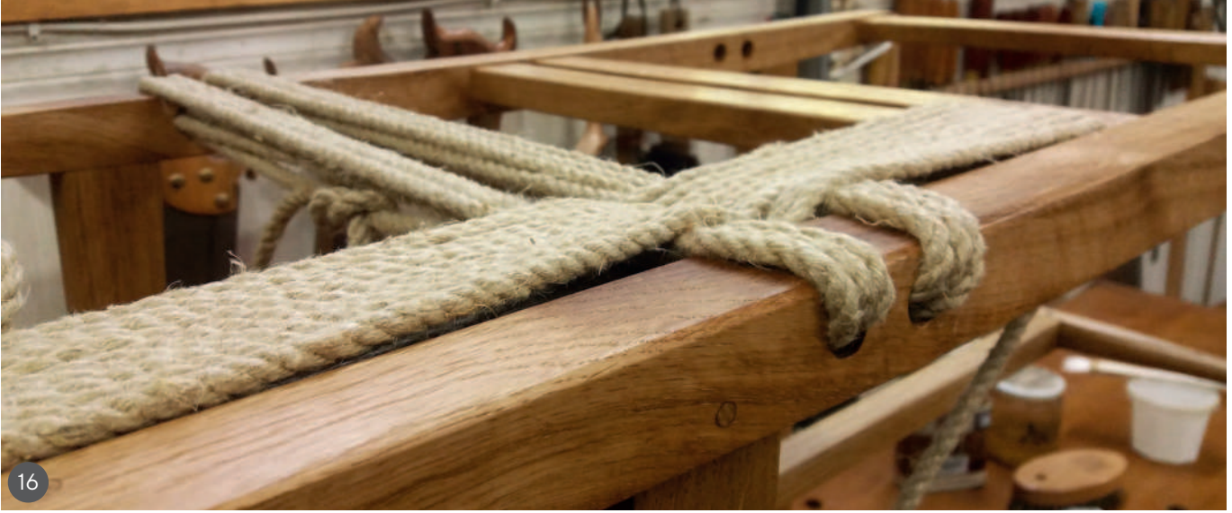
16 Weaving the hemp cord on the stool 17 One finished woven seat
