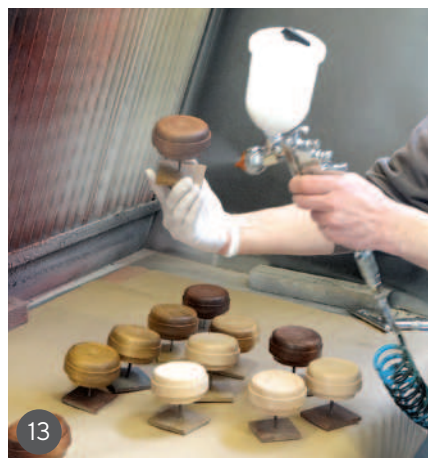
10 Sanding 11 Applying stain with a pad of paper towel 12 Using a brush to get into the details 13 The first coat of lacquer going down 14 The lighter areas on the bun feet 15 Adding the solvent-based stain to the lighter areas
