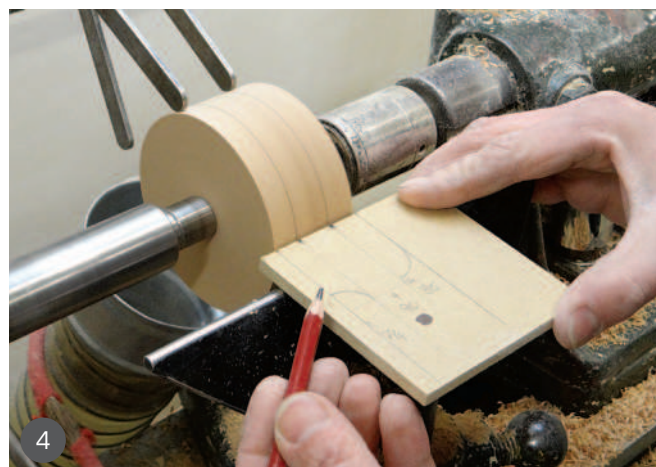
1 Preparing the timber for the bun feet 2 The octagons ready to turn 3 Checking the diameter with callipers 4 The story board in use
