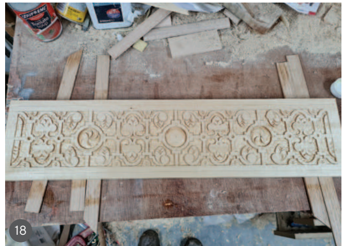
15 Create the pin wheel with strikes of the chisel, then remove a sliver of waste behind each strike 16 Add simple detail to the leaves and any punch work 17 A selection of punches is a good way to add detail to a carving like this 18 Apply the oil finish in several stages
