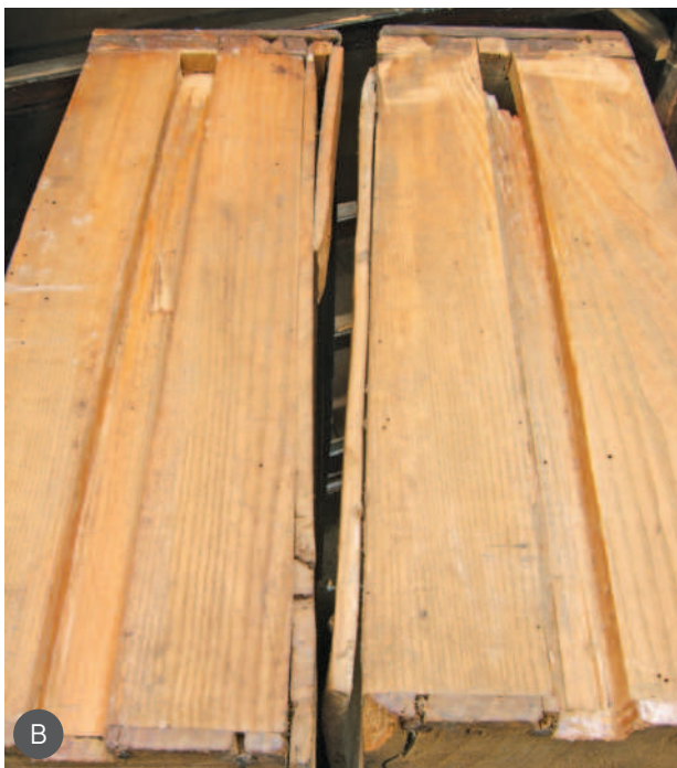
A One drawer's central panel was loose B This drawer had also been fitted with wedges and additional timber C The drawer fronts were tilted with uneven gaps around them D The drawer rails were loose and the grooves on the drawers' sides were worn and uneven
