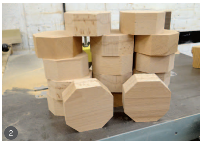
1 Preparing the timber for the bun feet 2 The octagons ready to turn 3 Checking the diameter with callipers 4 The story board in use
