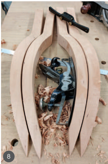
5 The MDF leg template was used to mark out the curves 6 The legs were then roughed out on the bandsaw before shaping on the spindle moulder 7 & 8 The legs were finished using a compass plane 9 The complete frame for the outer table 10 More leg templates were needed for the inner tables
