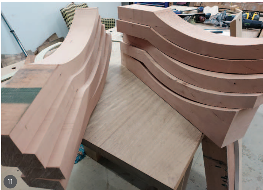
11 The tables were rough cut then shaped with a flexible template before being cut to length 12 The legs were assembled with the side and front rails
