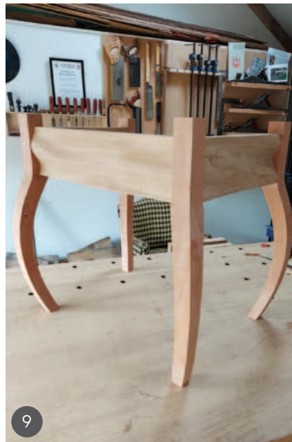
5 The MDF leg template was used to mark out the curves 6 The legs were then roughed out on the bandsaw before shaping on the spindle moulder 7 & 8 The legs were finished using a compass plane 9 The complete frame for the outer table 10 More leg templates were needed for the inner tables
