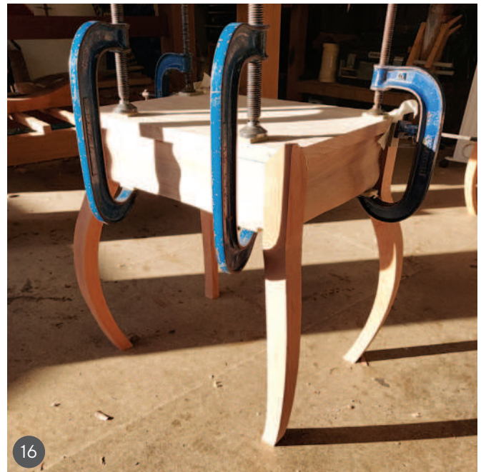
13 & 14 A quick check showed that the tables fit together correctly 15 The tops and frames were joined up successfully ... 16 ... before being jointed and clamped in place
