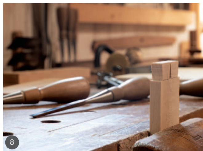
5 One box ... 6 ... two boxes! 7 The drawer fronts 8 Making the dovetails 9 London pattern drawer dovetails 10 The sliding dovetails for the back 11 The finished drawer, ready to be cleaned 12 & 13 Applying shellac to the boxes and drawers 14 Adding blue tape on the drawers helps when applying the finish 15 The drawer is complete but without the pulls
