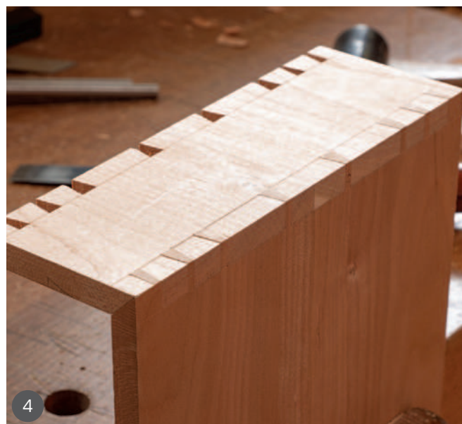
1 Starting to build the carcass: dimensioning the wood 2 The book-matched cherry 3 Detail of the joinery 4 Dry-fitting the carcass
