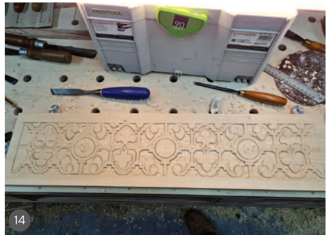
11 The large leaves at either end of the pattern can now be carved 12 Four strikes of the gouge produce the small diamond at the heart of the fleur-de-lis 13 The leaves are carved using chisels to match the shapes 14 With all the lines marked out, it's time to remove the background
