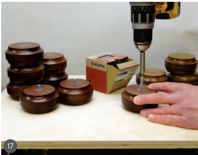
16 Cutting back with a red abrasive pad 17 Adding the stud screws 18 The finished bun feet 19 One of the upholstered ottomans fitted with the bun feet
