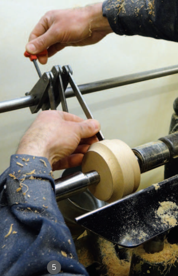
5 Setting the duplicating fingers 6 Turning the cove 7 The duplicating finger drops as I reach the required diameter 8 Turning the bead 9 The negative rake scraper leaves a crisp corner
