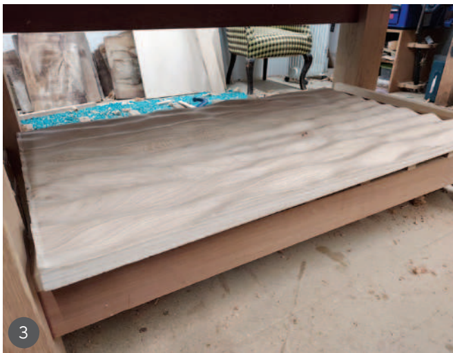
1 The Dune hall table inspired this new commission for a nest of tables 2 The initial concept for the nest of tables was laid out in a 3D watercolour sketch 3 A solid oak plank was needed for the 'dune' effect profile 4 The design was refined to confirm how the tables would nest together
