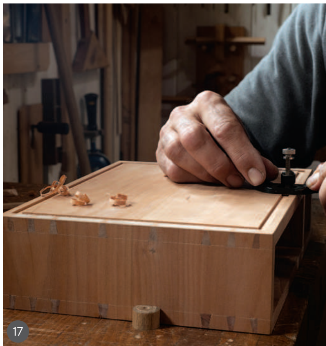
16 The pulls in place on two drawers 17 Making the grooves 18 The boxes with the sticks 19 The boxes fixed together 20 Planing the walnut crotch
