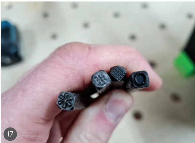
15 Create the pin wheel with strikes of the chisel, then remove a sliver of waste behind each strike 16 Add simple detail to the leaves and any punch work 17 A selection of punches is a good way to add detail to a carving like this 18 Apply the oil finish in several stages
