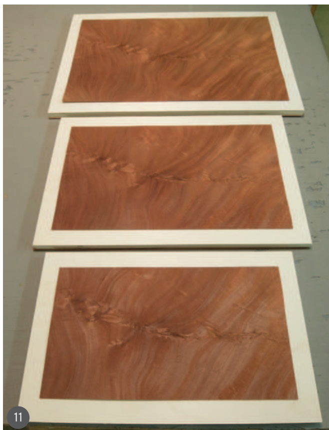
10 Veneering the cross-banding into place 11 The flame veneers, reducing in size, to keep the pattern central 12 Lifting the top corner piece to remove the waste piece below 13 Squeezing the glue out through the joint 14 Veneering with a vacuum press: the flame veneer, oversize and pressed into place ready for the edging
