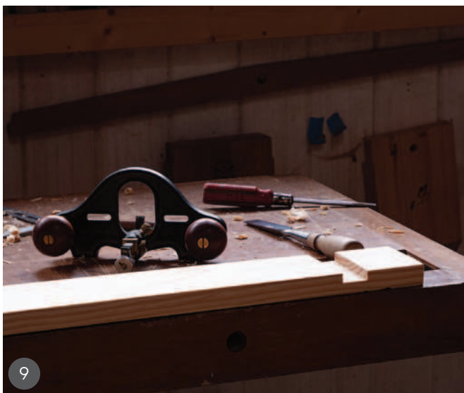
5 Drilling with the hand brace. 6 The mitred tenons and sliding dovetail in the middle of the aprons 7 & 8 Details of the crest rail joinery 9 The half-lap joint with the router plane 10 Planing the seat to join the two boards
