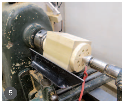
1 Checking the blocks are perfectly square 2 Holding the blocks together in clamps ensures a tight join while turning 3 Lining up the pads with 'cross hairs' 4 Fixing the pads with screws 5 Mounted on the lathe 6 Turning to a cylinder with my spindle roughing gouge
