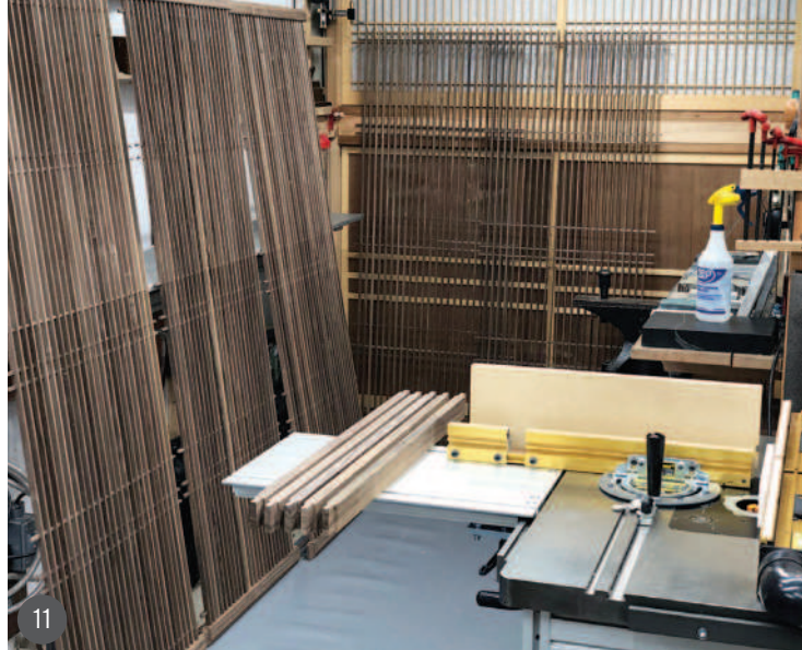
9 Precise gauge blocks were used to make the spacing accurate 10 & 11 The kumiko grid was assembled using a tight compression fit
