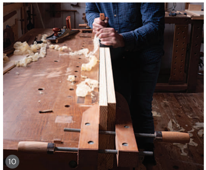
5 Drilling with the hand brace. 6 The mitred tenons and sliding dovetail in the middle of the aprons 7 & 8 Details of the crest rail joinery 9 The half-lap joint with the router plane 10 Planing the seat to join the two boards
