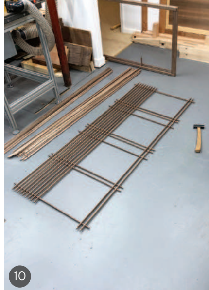
9 Precise gauge blocks were used to make the spacing accurate 10 & 11 The kumiko grid was assembled using a tight compression fit
