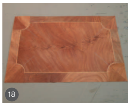
15 The complete built-up pattern taped on the face side 16 Fitting a preformed corner line to the corner 17 Finding and marking the line of the mitre 18 The completed pattern from the back 19 The panel placed in the vacuum bag press 20 Press-veneered panel (top), hand-veneered panel (bottom)
