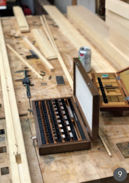
9 Precise gauge blocks were used to make the spacing accurate 10 & 11 The kumiko grid was assembled using a tight compression fit
