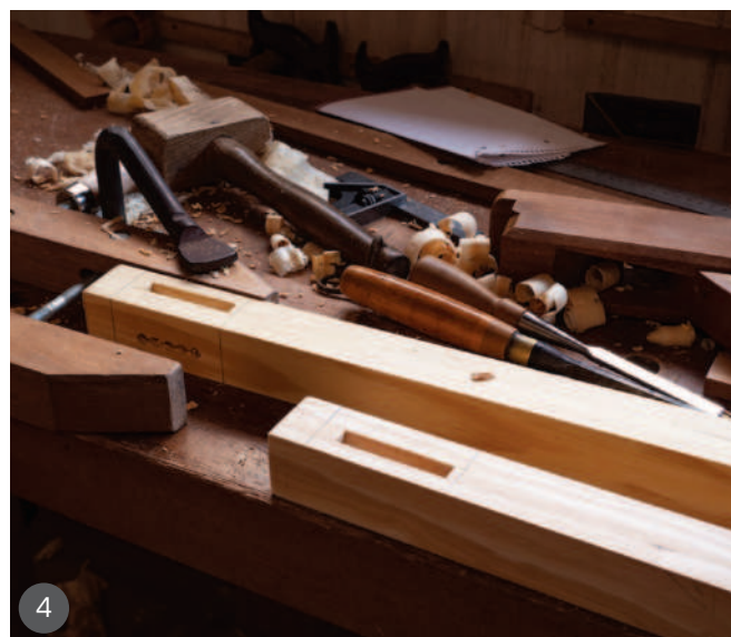
1 Planing the aprons and legs 2 The prepared front and back legs 3 Planing the long apron edges 4 The mitred mortises
