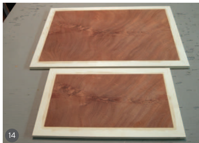
10 Veneering the cross-banding into place 11 The flame veneers, reducing in size, to keep the pattern central 12 Lifting the top corner piece to remove the waste piece below 13 Squeezing the glue out through the joint 14 Veneering with a vacuum press: the flame veneer, oversize and pressed into place ready for the edging
