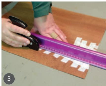
1 I made these veneer hammers from beech and brass 2 A bag press kit helps you get consistent pressure 3 Hand veneering: cutting the counterbalance veneer 4 Veneering a top with everything in reach 5 Gluing the back side of the veneer before turning over 6 Laying the veneer with the veneer hammer 7 Warming areas as necessary with an iron 8 Trimming the corners to a template 9 Square white line being shaped to the corner
