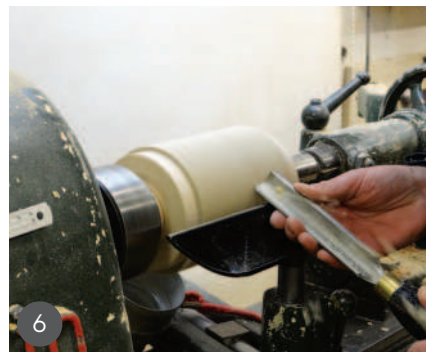
1 Checking the blocks are perfectly square 2 Holding the blocks together in clamps ensures a tight join while turning 3 Lining up the pads with 'cross hairs' 4 Fixing the pads with screws 5 Mounted on the lathe 6 Turning to a cylinder with my spindle roughing gouge
