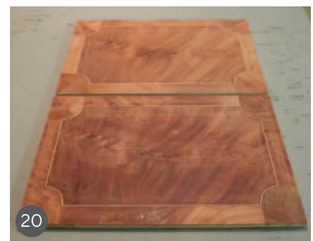
15 The complete built-up pattern taped on the face side 16 Fitting a preformed corner line to the corner 17 Finding and marking the line of the mitre 18 The completed pattern from the back 19 The panel placed in the vacuum bag press 20 Press-veneered panel (top), hand-veneered panel (bottom)
