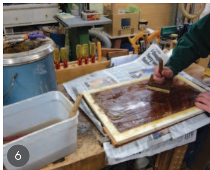
1 I made these veneer hammers from beech and brass 2 A bag press kit helps you get consistent pressure 3 Hand veneering: cutting the counterbalance veneer 4 Veneering a top with everything in reach 5 Gluing the back side of the veneer before turning over 6 Laying the veneer with the veneer hammer 7 Warming areas as necessary with an iron 8 Trimming the corners to a template 9 Square white line being shaped to the corner
