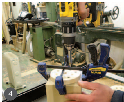
1 Checking the blocks are perfectly square 2 Holding the blocks together in clamps ensures a tight join while turning 3 Lining up the pads with 'cross hairs' 4 Fixing the pads with screws 5 Mounted on the lathe 6 Turning to a cylinder with my spindle roughing gouge
