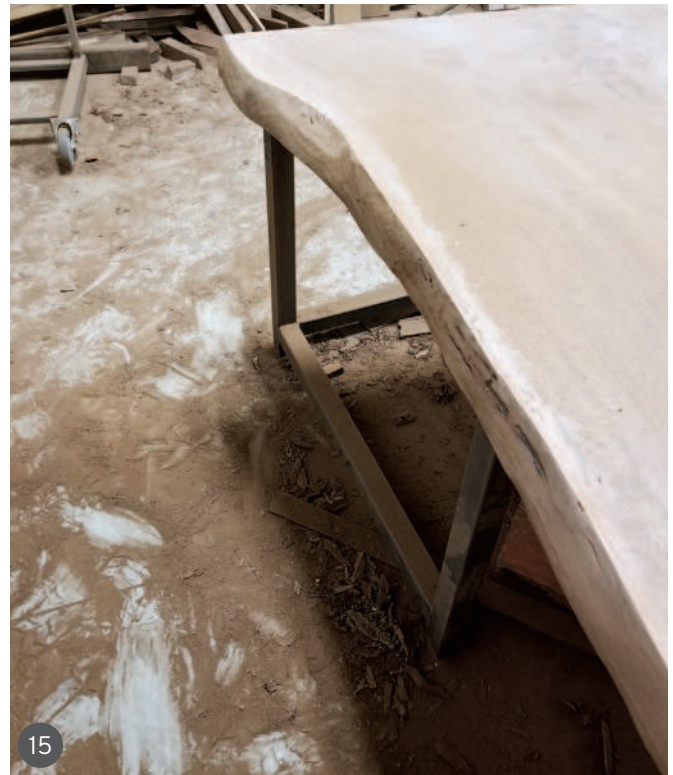
14 The pieces of the Lorraine lattice inlaid into the top 15 Sculpting the edges of the table top to be smooth and flow with the grain 16 The table base is a box steel frame cut and welded to size 17 Details on the table top include bowties and epoxy filler for a smooth writing surface and a stable worktop 18 The boardroom table in situ, after two years' use
