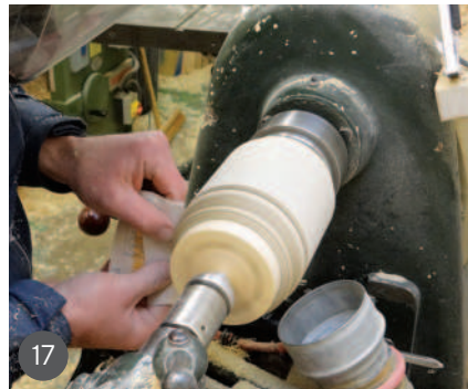
13 Checking my progress against the sample 14 Removing a quadrant from the block 15 Comparing it to the sample shows which areas need more work 16 Further refining the shape 17 Sanding with 180 grit 18 The finished moulding blocks
