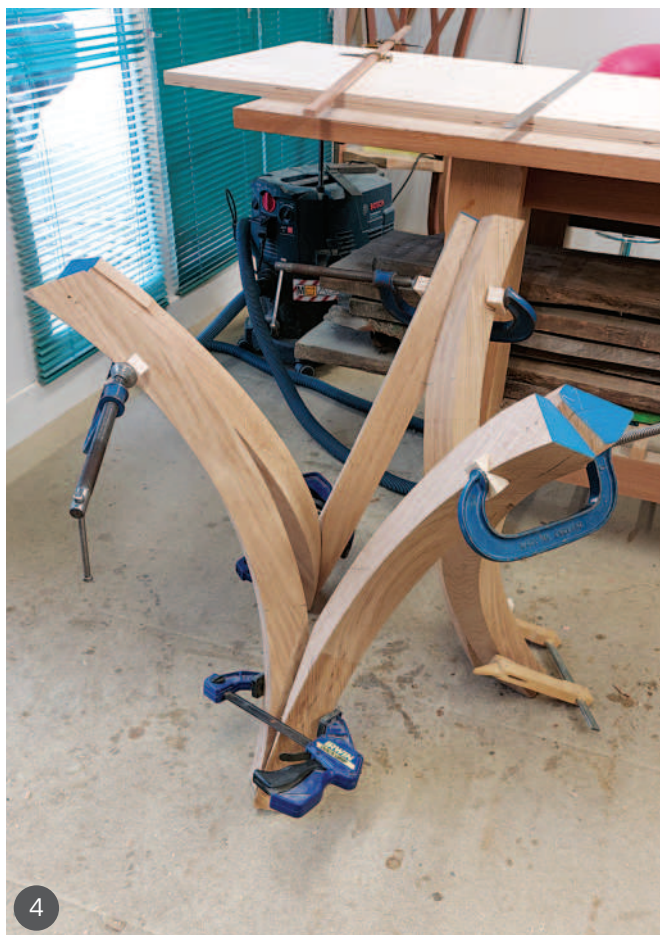
4 I mocked up a fit of the framework to check the shape
