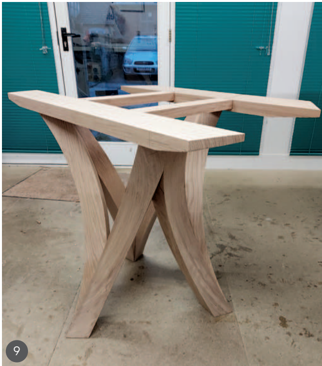
9 & 10 A supporting framework was made from 30mm solid oak 11 The top was oiled first as this was the main feature of the table 12 With the oil finish complete, the table was ready for delivery on Christmas Eve
