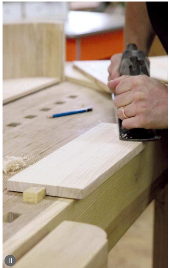
9 The bottom of the drawer was thicker than the groove that holds it, so some material was removed along the perimeter using a special bearing 10 The bonding between the drawer front and bottom is limited to the short side portions. The bottom acts as a spacer between the sides without preventing seasonal wood movements on the front 11 All the drawer pieces were finished with a hand plane before assembly
