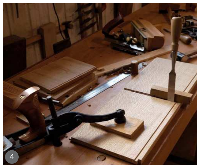
1 Dimensioning the stock by hand 2 Working on the carcass joinery 3 Dry fit of the carcass 4 Making the sliding dovetail for the divider
