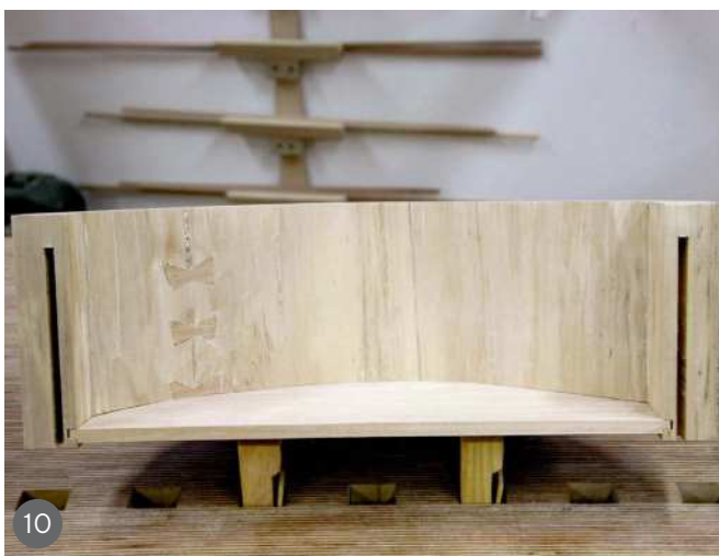
9 The bottom of the drawer was thicker than the groove that holds it, so some material was removed along the perimeter using a special bearing 10 The bonding between the drawer front and bottom is limited to the short side portions. The bottom acts as a spacer between the sides without preventing seasonal wood movements on the front 11 All the drawer pieces were finished with a hand plane before assembly
