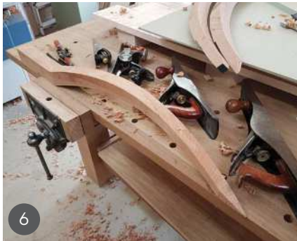
5 The spindle moulder was used to produce the first curve deflection ... 6 ... but the next stage was done by hand 7 The four completed legs. My intention was to create a modern version of the cabriole leg shape 8 The carcass sides were jointed and clamped to the legs 9 & 10 The dovetails at the tops of the legs were worked by hand
