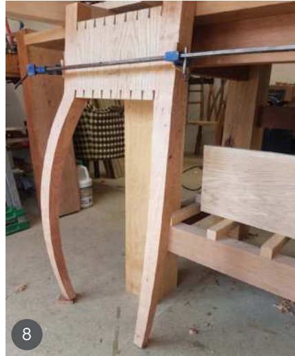
5 The spindle moulder was used to produce the first curve deflection ... 6 ... but the next stage was done by hand 7 The four completed legs. My intention was to create a modern version of the cabriole leg shape 8 The carcass sides were jointed and clamped to the legs 9 & 10 The dovetails at the tops of the legs were worked by hand
