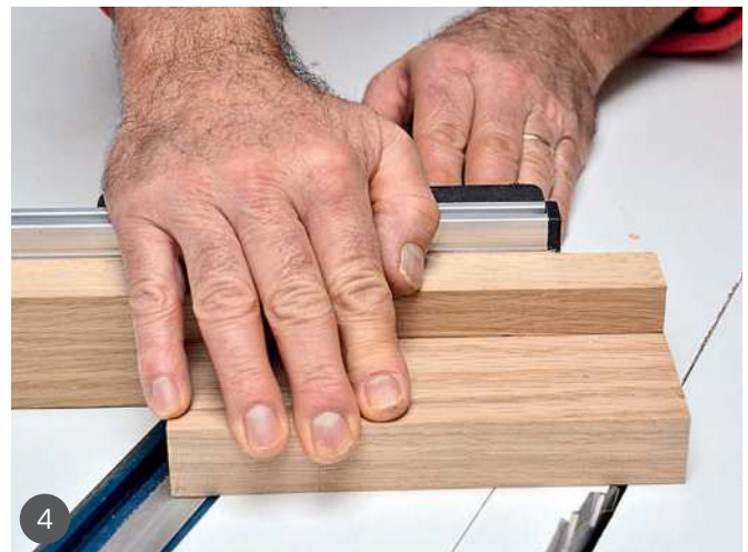
1 My drawing of the joint 2 The tools used to measure the angles and transfer them from the paper to the mitre fence of the saw bench 3 The angle fences supplied with many machines do not normally exceed 45°. To cut more obtuse angles a wedge can be added to the fence to increase the angle it will make 4 Here you can see the angle of the cuts on the crosspiece for which it is not necessary to add the wedge
