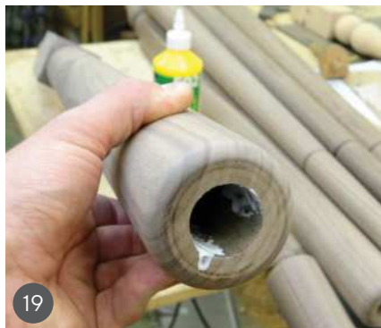
17 Sanding to 320 grit 18 Cutting key lines in the tenon 19 Gluing three-quarters of the way around the mortise to avoid an airlock 20 The complete set of posts, standing vertical to dry
