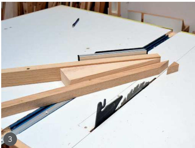
1 My drawing of the joint 2 The tools used to measure the angles and transfer them from the paper to the mitre fence of the saw bench 3 The angle fences supplied with many machines do not normally exceed 45°. To cut more obtuse angles a wedge can be added to the fence to increase the angle it will make 4 Here you can see the angle of the cuts on the crosspiece for which it is not necessary to add the wedge
