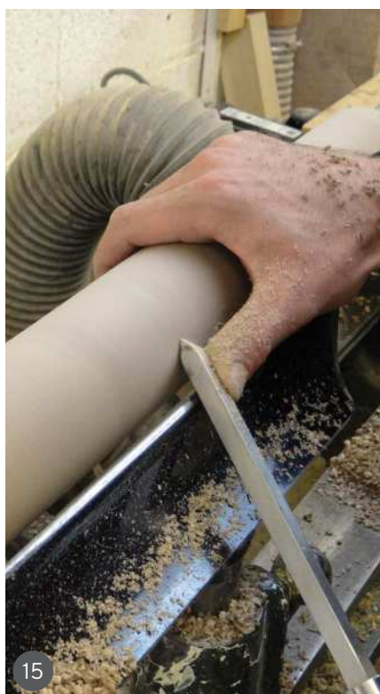
13 Forming the taper 14 Checking with a straightedge 15 Planing with my beading and parting tool, offering support to the work with my front hand 16 Forming the V-groove with rounded edge detail
