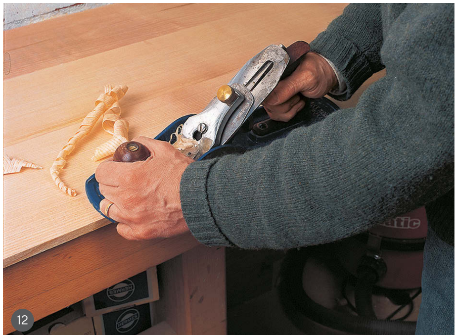
10 Catch and chamfered top detail 11 Close-up of panel 12 Planing the chamfer on the underside of the top
