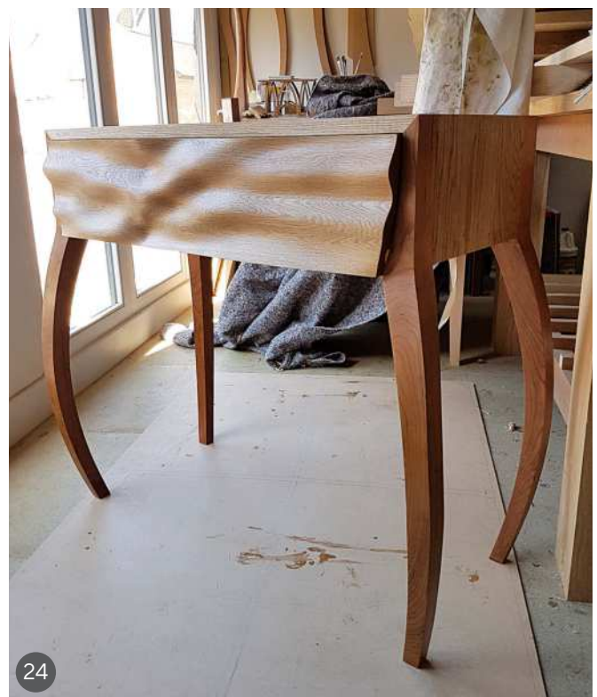
21 The drawer jointed, ready for glue 22 & 23 A central muntin was added to fix the piece 24 Four coats of Osmo Oolyx Satin oil provided the finish
