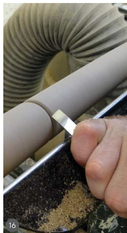
13 Forming the taper 14 Checking with a straightedge 15 Planing with my beading and parting tool, offering support to the work with my front hand 16 Forming the V-groove with rounded edge detail
