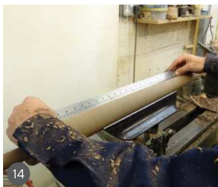
13 Forming the taper 14 Checking with a straightedge 15 Planing with my beading and parting tool, offering support to the work with my front hand 16 Forming the V-groove with rounded edge detail
