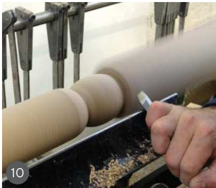
7 The holes cleanly drilled 8 The tools used to turn the bedposts 9 Setting out the foot of the leg 10 Cleanly slicing the pommels 11 The result of the cut 12 The live centre positioned in the hole
