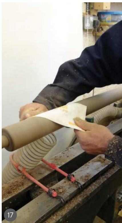
17 Sanding to 320 grit 18 Cutting key lines in the tenon 19 Gluing three-quarters of the way around the mortise to avoid an airlock 20 The complete set of posts, standing vertical to dry
