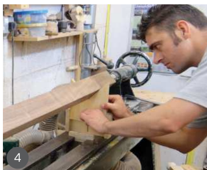
1 The walnut blanks 2 The beautiful flame figure in one piece of walnut 3 The modified drill bit held in the chuck 4 Setting up the V-shaped cradles 5 One hand on the timber, the other turning the hand wheel is all that's needed 6 Drilling in action
