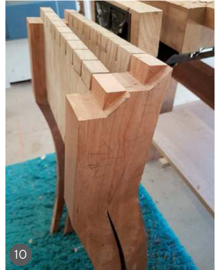
5 The spindle moulder was used to produce the first curve deflection ... 6 ... but the next stage was done by hand 7 The four completed legs. My intention was to create a modern version of the cabriole leg shape 8 The carcass sides were jointed and clamped to the legs 9 & 10 The dovetails at the tops of the legs were worked by hand
