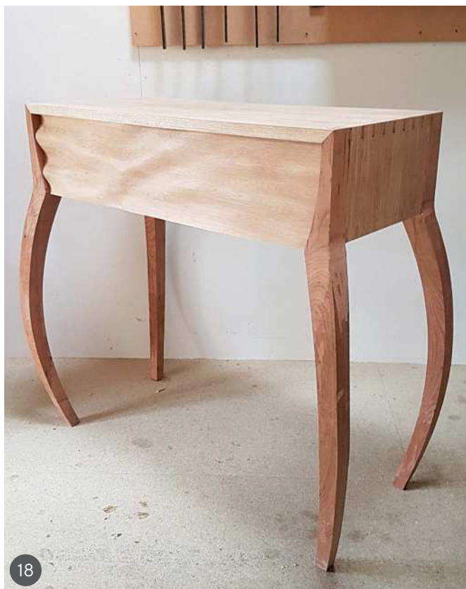
17 The glue-up, using sash clamps 18 & 19 The drawer has a sculpted, undulating front which is eye-catching but tricky to achieve 20 The drawer glued up
