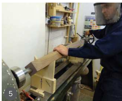
1 The walnut blanks 2 The beautiful flame figure in one piece of walnut 3 The modified drill bit held in the chuck 4 Setting up the V-shaped cradles 5 One hand on the timber, the other turning the hand wheel is all that's needed 6 Drilling in action
