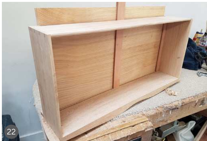
21 The drawer jointed, ready for glue 22 & 23 A central muntin was added to fix the piece 24 Four coats of Osmo Oolyx Satin oil provided the finish
