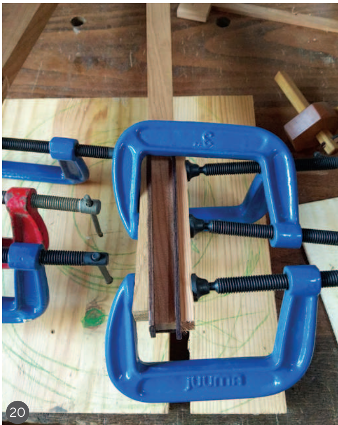
18 Ripping the rosewood for the feet 19 Working on the feet recess 20 Gluing the sides of the feet 21 Back piece of the feet 22 The completed feet
