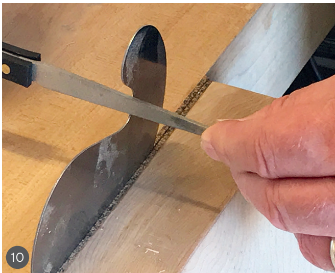
8 Angle the burnisher to about 10–15° to form the final burr along the edge 9 A burnisher deforms the steel at the edges of the card scraper to begin forming a burr. Start with the burnisher square to the faces of the scraper 10 A small diamond file is ideal for polishing the edge of a curved scraper before using a burnisher to form the burr 11 Burnish the edges of a curved scraper the same way you would a straight scraper edge
