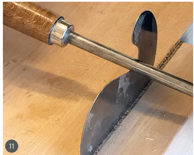
8 Angle the burnisher to about 10–15° to form the final burr along the edge 9 A burnisher deforms the steel at the edges of the card scraper to begin forming a burr. Start with the burnisher square to the faces of the scraper 10 A small diamond file is ideal for polishing the edge of a curved scraper before using a burnisher to form the burr 11 Burnish the edges of a curved scraper the same way you would a straight scraper edge
