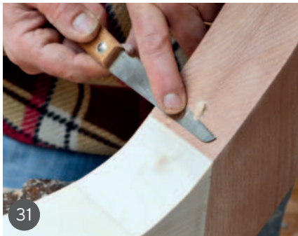
30 Driving in discreet dowels to help hold the tenons in place 31 Using a trimming pullsaw to flush off the dowels 32 The finished table and chairs
