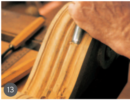
13 Rounding over the convex part of the cyma with an inverted gouge. A back-bent gouge is helpful where the curve changes direction near the lower baluster. Some filing and sanding will be needed to produce a uniform finish 14 The completed volute from the side 15 A three-quarter view, showing the bead and cyma treatment on the front
