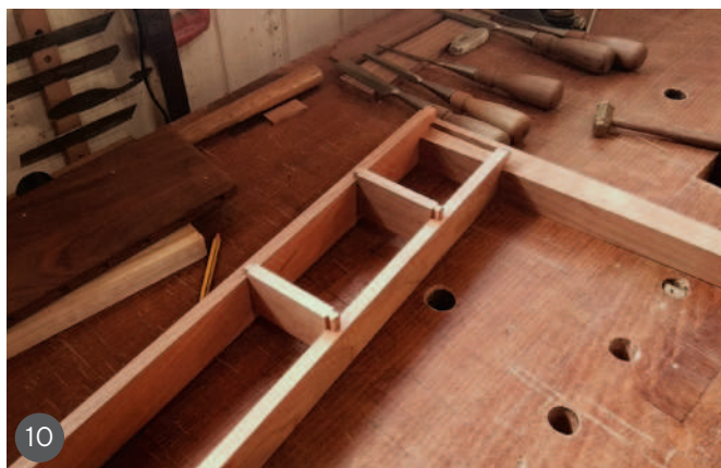
8 Side apron with the drawer before joinery 9 Detail of the side drawer 10 Sliding dovetails on vertical dividers 11 Front view of the vertical dividers 12 Gluing the drawer front veneers 13 Drawer pieces ready for joinery 14 The front drawers 15 Details of the front drawer pulls 16 Front view of the rosewood bead 17 Detail of the bead from underneath
