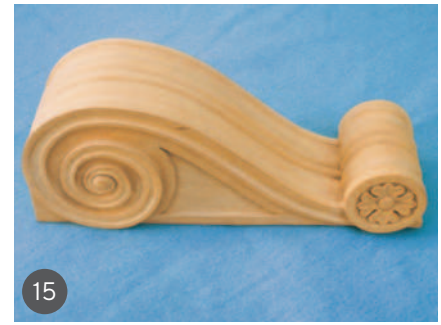
13 Rounding over the convex part of the cyma with an inverted gouge. A back-bent gouge is helpful where the curve changes direction near the lower baluster. Some filing and sanding will be needed to produce a uniform finish 14 The completed volute from the side 15 A three-quarter view, showing the bead and cyma treatment on the front
