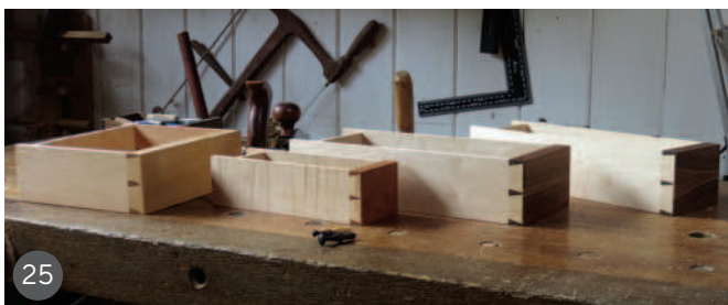
23 Detail of the London pattern dovetails 24 Transferring the tails to get the pins 25 All the drawers joined with London pattern dovetails 26 Detail of the drawer bottoms 27 The cedar of Lebanon drawer bottoms
