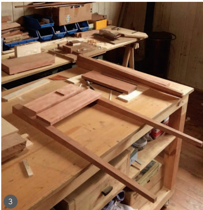
1 Shaping the legs 2 Laying out the side drawer apron 3 Marking for the mortises 4 Detail of the double dovetails joining the leg and side apron 5 Detail of the lower front blade joinery (twin tenons) 6 & 7 Front and side views of the complete structure
