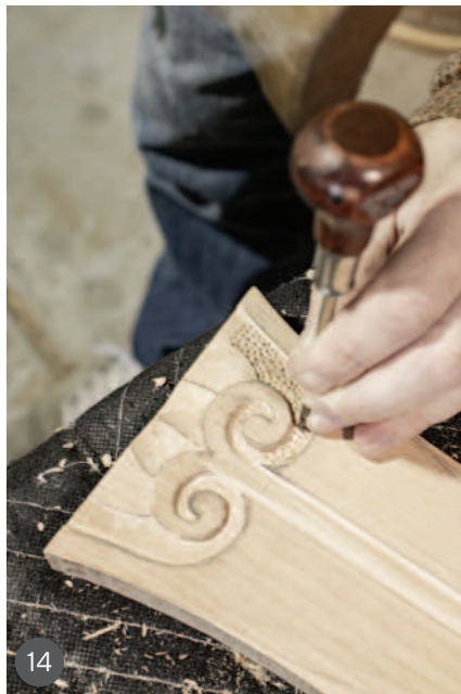
13–16 Using an awl to match textures in the carvings from the original chair
