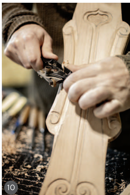
7 Completing the cuts to the profiles 8 & 9 Beginning the carving 10–12 Adding shaped details to match the originals
