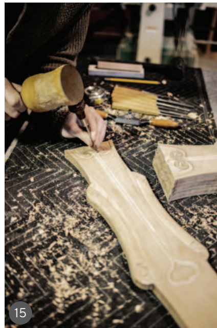
13–16 Using an awl to match textures in the carvings from the original chair
