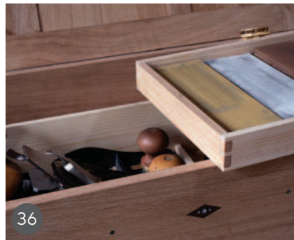
29 Working on the rosewood diamonds 30 Details of the inlays 31 The finished mother of pearl and rosewood inlay details 32 Main compartment division layout 33 The division dovetails 34 Divisions for the tools 35 The joinery details 36 The tray for storing waterstones 37 Overview of the tray and divisions
