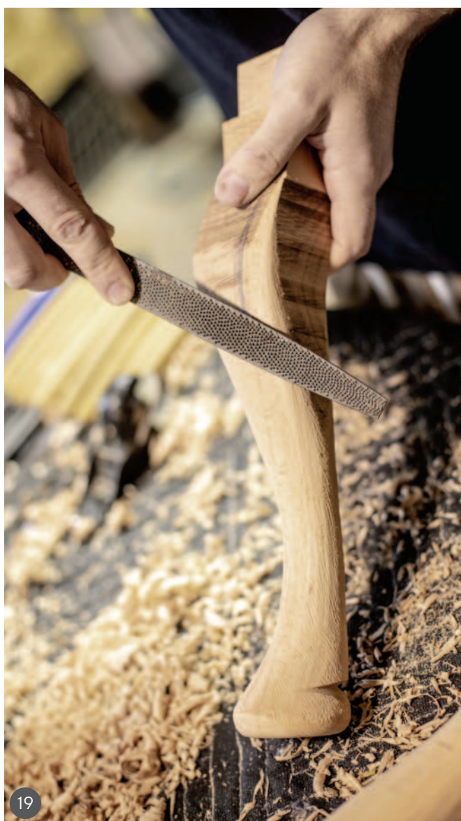
17 & 18 Turning the front legs to match the original profile 19 & 20 Using a rasp to finalise the shape of the front legs
