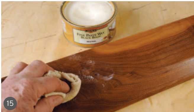
13 Tallow is a very solid, sticky form of blade lubricant useful for handsaws 14 Dark hardening wax is good for filling gaps and helping the antique look 15 Hardening wax needs positive pressure to stick evenly to a highly finished surface 16 A natural bristle brush is good for buffing without damaging surfaces
