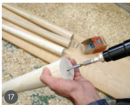
14 Using a storyboard to carefully mark the positions of the fixing tenon and the bottom of the leg 15 Rounding the bottom of the leg with my beading and parting tool 16 Drilling the pilot hole using tailstock support to ensure perfect concentricity 17 Fitting the stud screw into the ash legs 18 The finished ash legs 19 The finished oak legs
