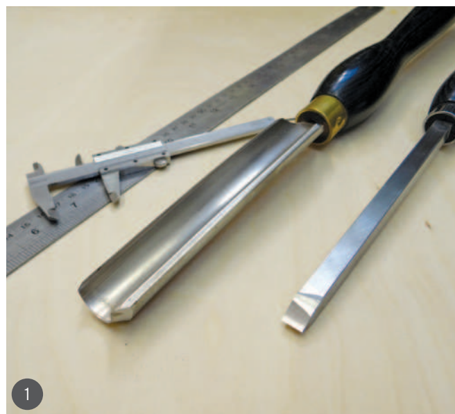
1 The tools for the job. From left to right: spindle roughing gouge, beading and parting tool, Vernier callipers and a straight edge
