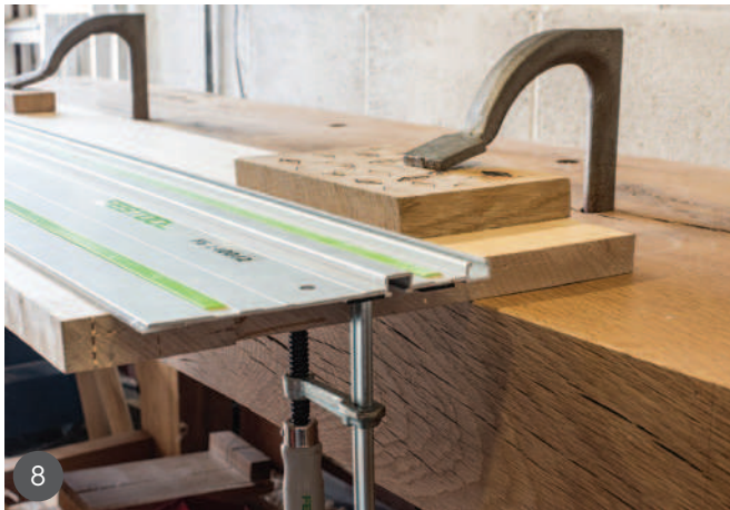
8 Blending modern and historic technology – holdfasts and a sturdy bench top also facilitate using power tools such as a track saw
