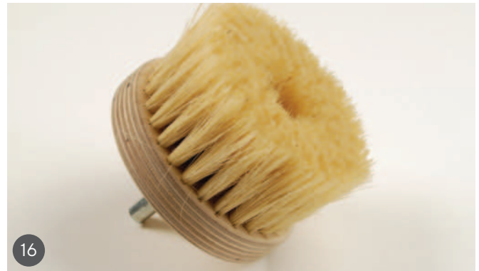
13 Tallow is a very solid, sticky form of blade lubricant useful for handsaws 14 Dark hardening wax is good for filling gaps and helping the antique look 15 Hardening wax needs positive pressure to stick evenly to a highly finished surface 16 A natural bristle brush is good for buffing without damaging surfaces
