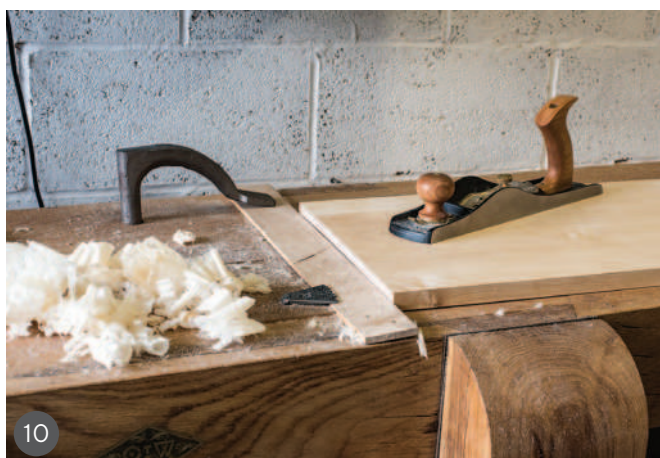
10 For working along the grain of wide boards, a thin batten can be held in place with a holdfast and planing stop
