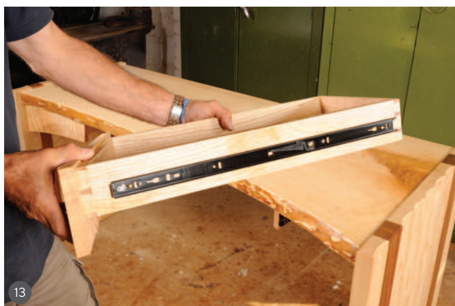
10 Very long single flute screws will hold the desk tightly together 11 A ratchet driver with a Torx bit makes assembly quick and easy 12 The rail needs to go in place before the end is tightened up 13 Now for the side-mounted drawer runners to complete the desk
