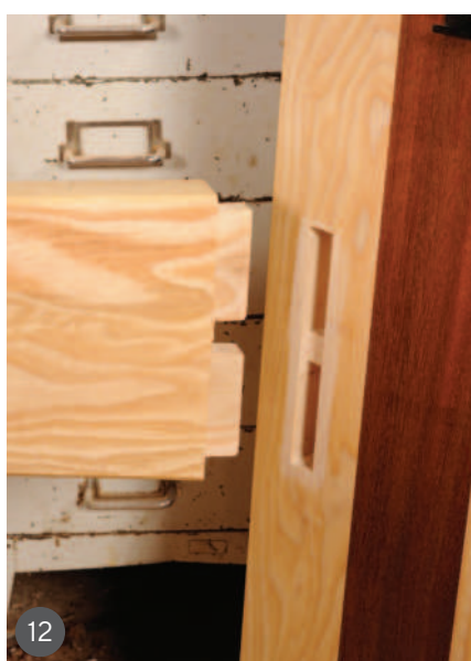
10 Very long single flute screws will hold the desk tightly together 11 A ratchet driver with a Torx bit makes assembly quick and easy 12 The rail needs to go in place before the end is tightened up 13 Now for the side-mounted drawer runners to complete the desk
