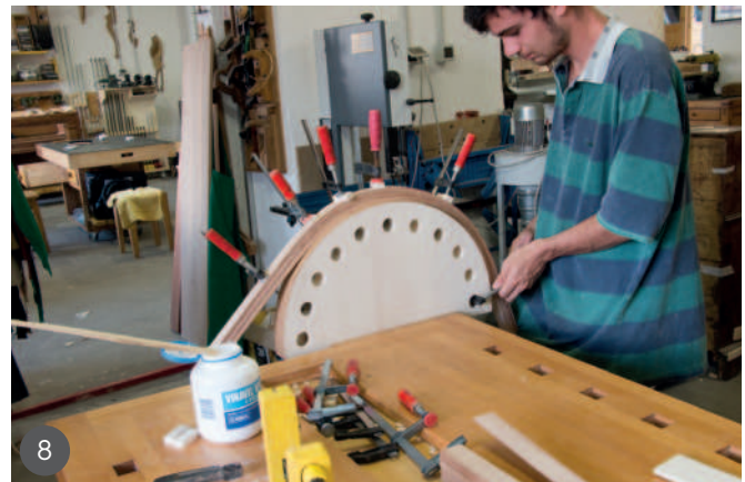
5 Assessing the strips' ability to bend without breaking 6 Trimming the edges of the ply close to the already spokeshaved board 7 Using a straight profile cutter to trim the curve to shape 8 Using a jig to clamp the curved lamp arm
