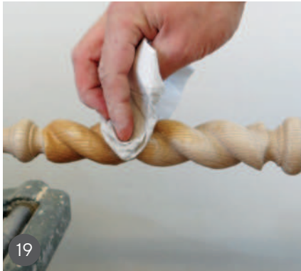
16 The sanding stick in action 17 The twist is looking much improved in this comparison 18 Working with the strip of abrasive 19 Wetting the twist 20 Final sanding with the lathe running at 200rpm 21 The final tidying cut in the cove, to crisp the end of the twist
