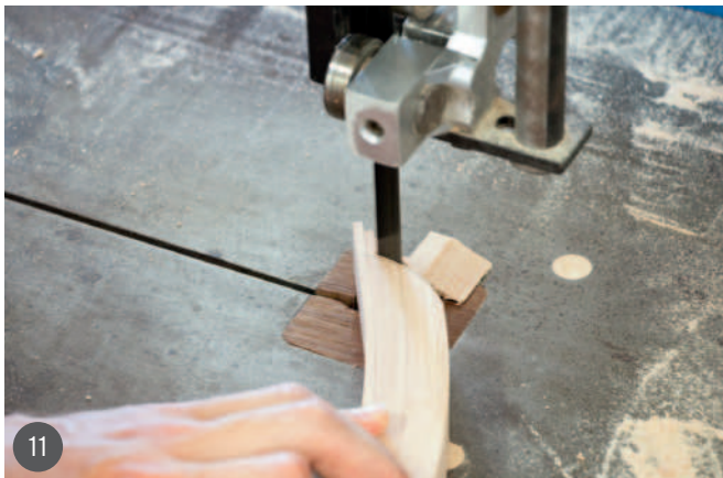
9 Showing the glue squeeze-out when clamped 10 Trimming the arm curve to width 11 The end of the arm being sawn off before sanding 12 A rasp being used to finish the shaping
