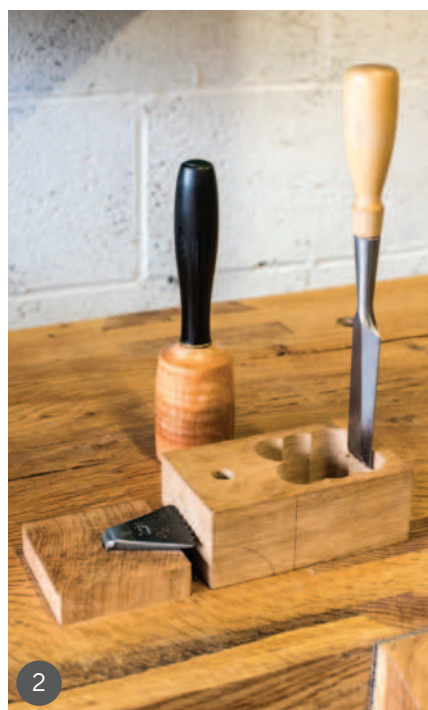
OPPOSITE Testing the location of the grease box, using an auger bit as a temporary fixing 1 Boring the well with a Forstner bit in a hand brace 2 Paring the walls of the well 3 I start by paring the end grain, followed by the side walls 4 The completed well
