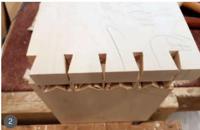
1 Paring down the pins 2 & 3 Checking for fit 4 The dry assembly
