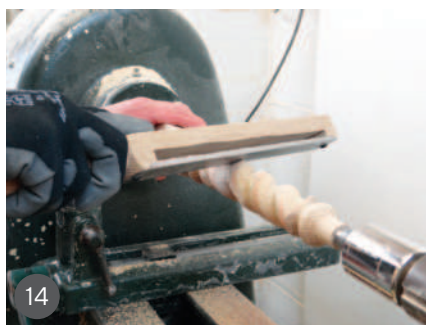
10 The initial grooves complete, and comparing it to the original 11 Working with the larger Microplane 12 Comparing with the original again after the groove is cut 13 Microplane rasps 14 The rigid Microplane blade in use 15 Comparing with the original once again
