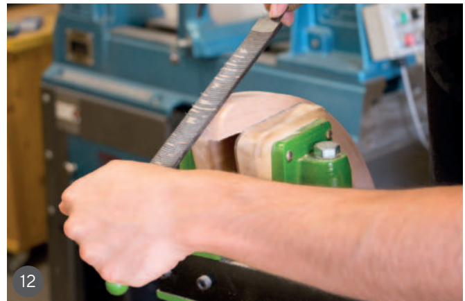
9 Showing the glue squeeze-out when clamped 10 Trimming the arm curve to width 11 The end of the arm being sawn off before sanding 12 A rasp being used to finish the shaping
