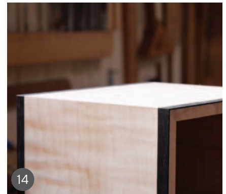
7 Making dados for the drawer runners 8 The glued-up carcass 9 The back, made from red cedar 10 Sawing ebony by hand 11 Planing the ebony strips 12 Planing the inlays once they are glued up 13 The carcass is done 14 Details of the edge inlays
