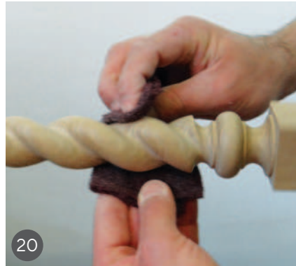
16 The sanding stick in action 17 The twist is looking much improved in this comparison 18 Working with the strip of abrasive 19 Wetting the twist 20 Final sanding with the lathe running at 200rpm 21 The final tidying cut in the cove, to crisp the end of the twist
