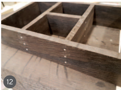
11 Gluing up the tray work 12 The sycamore dowel pins 13 The veneer key and reinforcement pin work 14 Ready for the clean down 15 Fitting the trays 16 Veneer key reinforcements
