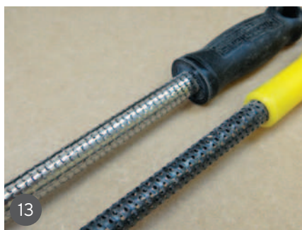
10 The initial grooves complete, and comparing it to the original 11 Working with the larger Microplane 12 Comparing with the original again after the groove is cut 13 Microplane rasps 14 The rigid Microplane blade in use 15 Comparing with the original once again
