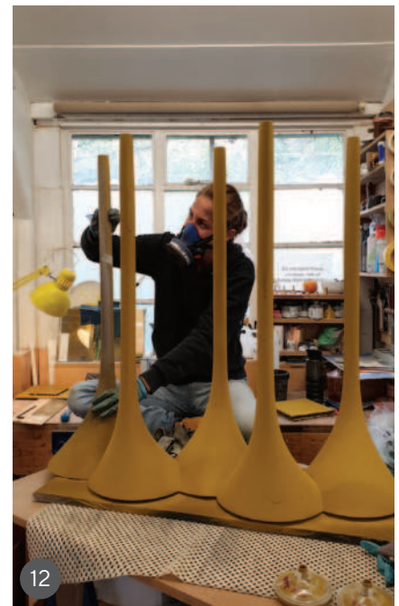
7 The turned brass fit, which will be attached later 8 Progress so far, all bonded together ready for the next stage 9 The deep cone shape in each leg component 10 The tops of the cones coated with metallised paint which is being rubbed back 11 The brass effect starts to appear as if by magic 12 Now for the legs – a respirator is essential because of the metal dust generated
