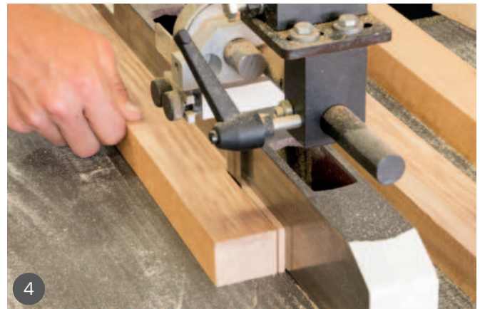
1 Cutting out the birch ply for the lamp base 2 Levelling the edge using a spokeshave 3 Gluing up the base sandwich construction 4 Bandsawing lamination strips with a fine skip tooth blade
