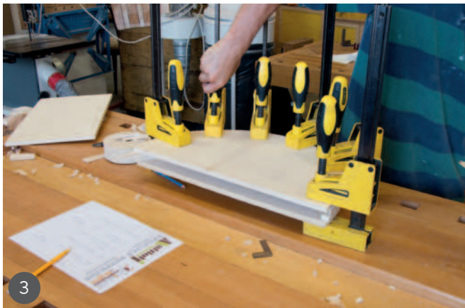
1 Cutting out the birch ply for the lamp base 2 Levelling the edge using a spokeshave 3 Gluing up the base sandwich construction 4 Bandsawing lamination strips with a fine skip tooth blade
