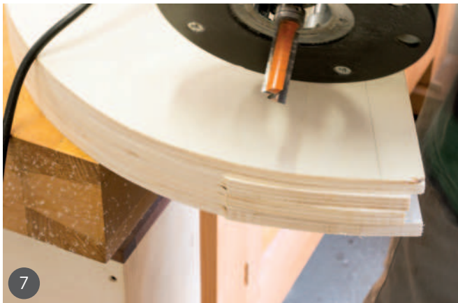
5 Assessing the strips' ability to bend without breaking 6 Trimming the edges of the ply close to the already spokeshaved board 7 Using a straight profile cutter to trim the curve to shape 8 Using a jig to clamp the curved lamp arm
