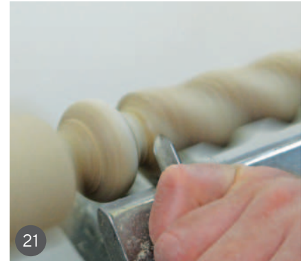
16 The sanding stick in action 17 The twist is looking much improved in this comparison 18 Working with the strip of abrasive 19 Wetting the twist 20 Final sanding with the lathe running at 200rpm 21 The final tidying cut in the cove, to crisp the end of the twist
