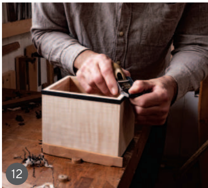
7 Making dados for the drawer runners 8 The glued-up carcass 9 The back, made from red cedar 10 Sawing ebony by hand 11 Planing the ebony strips 12 Planing the inlays once they are glued up 13 The carcass is done 14 Details of the edge inlays
