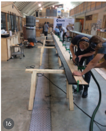
10 Before patching 11 After patching 12 Tracing the outline of each individual board 13 Mauro and Ricardo designing the river joint 14 Templates and tracings of the inserts 15 Gluing the inserts. The templates for the other inserts can be seen on the left 16 A full length template for the river joint clamped to the board as a majority of the waste material is being removed by a jigsaw 17 The first river joint 18 The level of accuracy to the river joint 19 The completed top, over 13 metres long and 5,000 years old 20 The making team – thank you!
