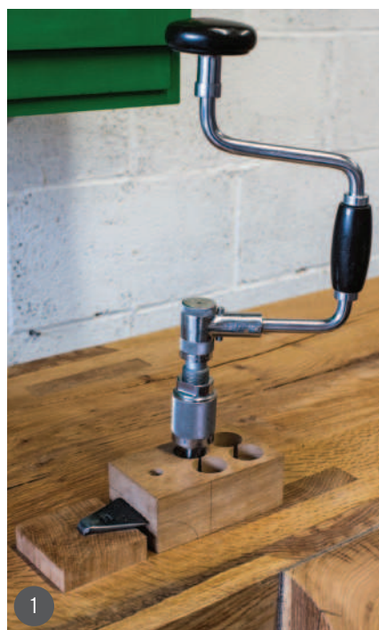
OPPOSITE Testing the location of the grease box, using an auger bit as a temporary fixing 1 Boring the well with a Forstner bit in a hand brace 2 Paring the walls of the well 3 I start by paring the end grain, followed by the side walls 4 The completed well
