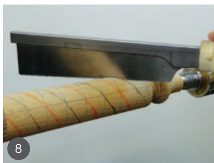
4 The pitch lines drawn on the spindle 5 The spindle showing the pitch lines in pencil and pitch dividing lines in blue 6 Drawing the lines across the grid 7 The setting out is complete with the valleys drawn in pencil and the bines marked in orange 8 First cuts with the saw 9 Making a groove with the small Microplane rasp, following the saw cut
